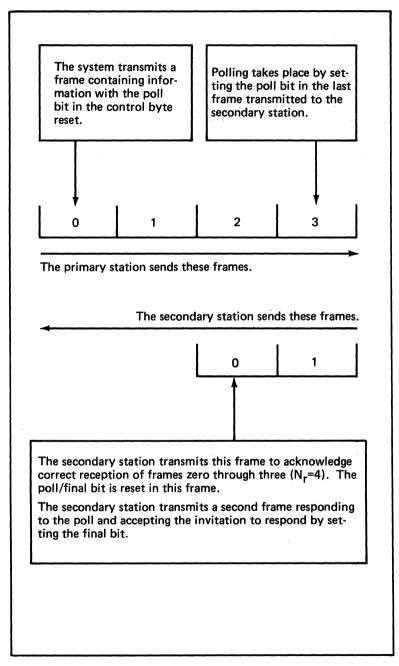
Figure 126. Polling takes place with the single P/F bit within the control byte of a frame
