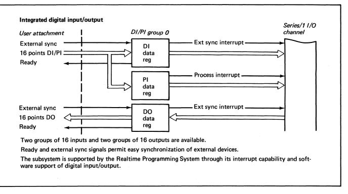
Figure 17. A subsystem can be flexibly configured to interface with a combination of analog and digital, input and output devices (3 of 4)
