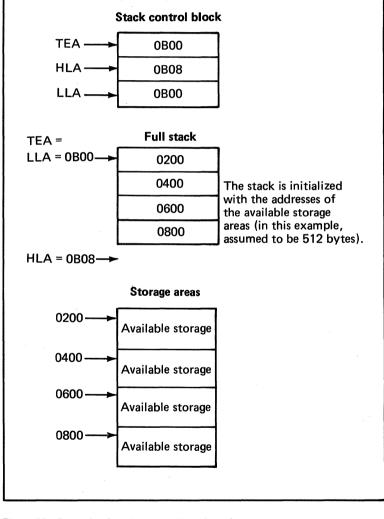
Figure 28. Example of stack usage: allocation of storage areas to concurrent programs (1 of 4)
