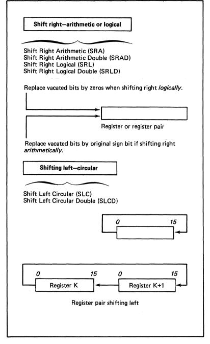
Figure 82. Options for shifting register contents (1 of 2)
