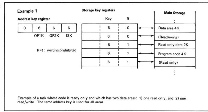
Figure 41. Three examples of address key storage protection (1 of 3)
