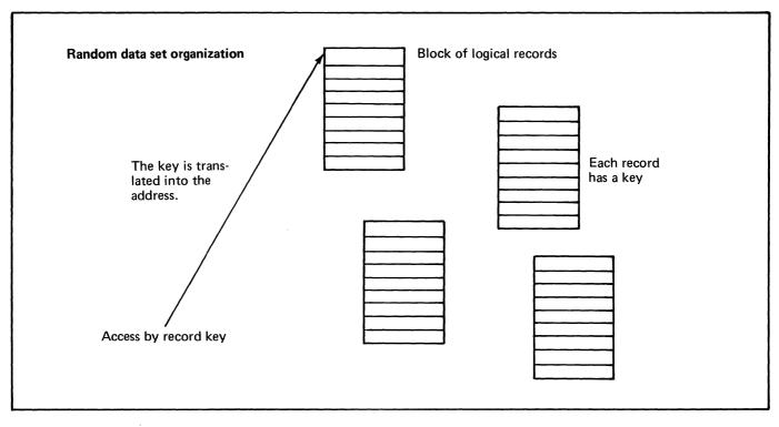
Figure 75. Four data set organizations supported under the Realtime Programming System (2 of 5)
