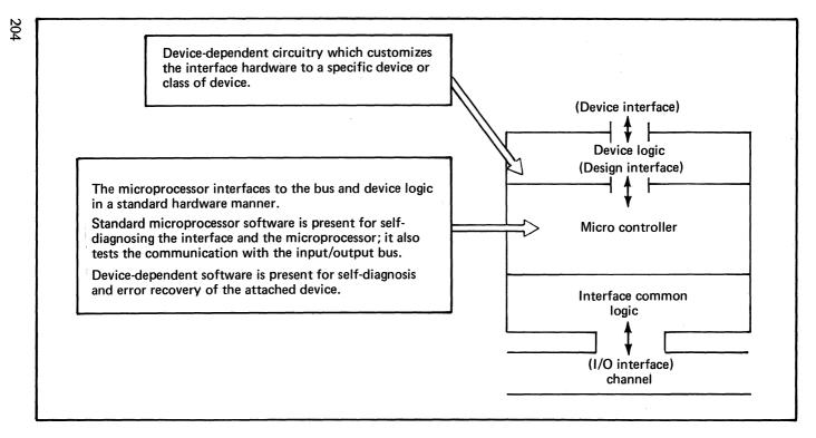
Figure 54. Organization of the microprocessor-controlled interface between the input/output channel and devices
