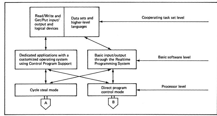
Figure 51. The levels from which input/output must be considered (1 of 2)
