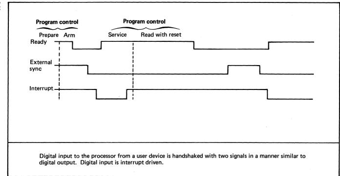
Figure 102. The handshake convention used on digital group output (part 2) (1 of 2)
