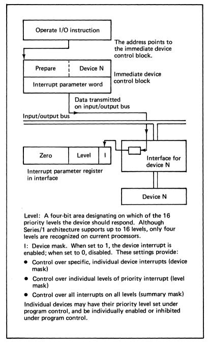
Figure 61. Individual devices under program control
