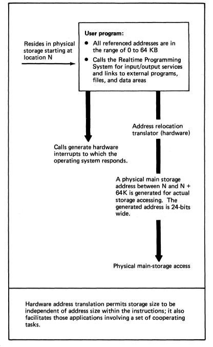
Figure 11. Address relocation for user programs
