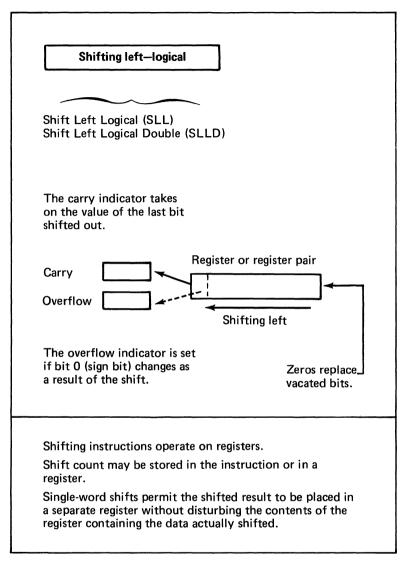
Figure 82. Options for shifting register contents (2 of 2)
