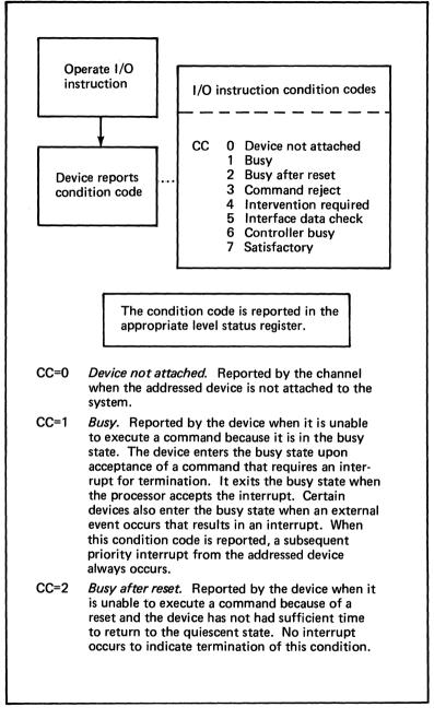
Figure 62. Definition of the eight condition codes which may be reported after each input/output instruction (1 of 2)
