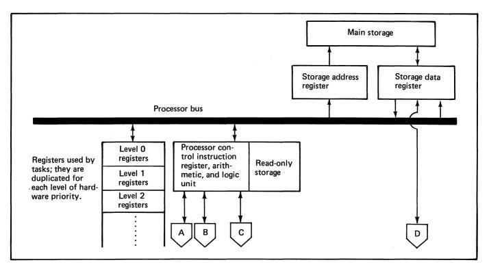
Figure 18. Overall data flow in the Series/1 processor (1 of 2)
