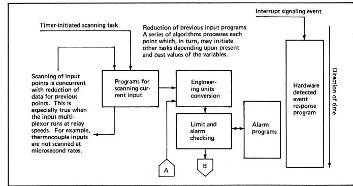
Figure 8. Set of concurrent tasks to carry out data acquisition and control (1 of 2)
