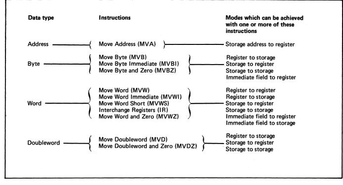
Figure 79. Series/1 instructions and modes for data movement (1 of 2)
