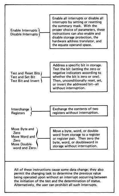
Figure 86. Instructions which can be used to control concurrency
