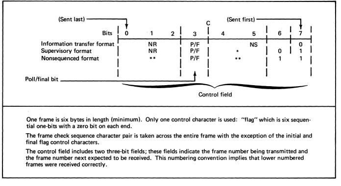
$\mathcal{N}_{1}$  Figure 124. Detailed definition of the SDLC frame format (2 of 2)
