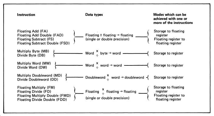
Figure 80. Arithmetic operations, data types, and modes (2 of 2)
