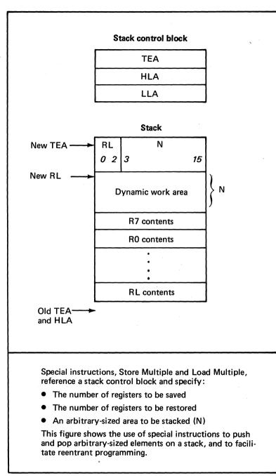
Figure 29. Example of hardware and software integrated design
