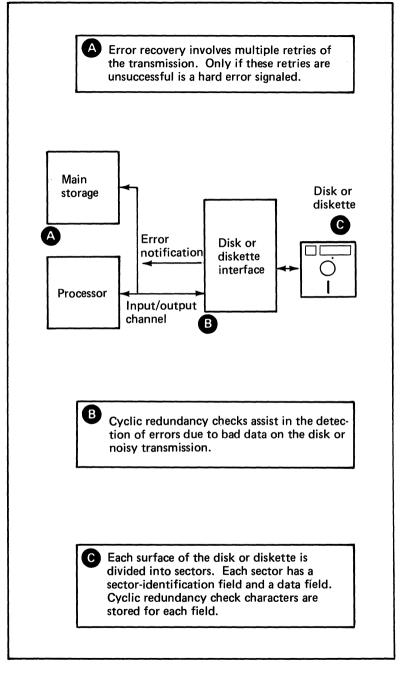
Figure 134. Disk and diskette error detection (1 of 2)
