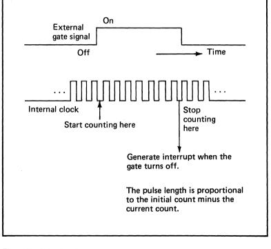
Figure 97. Pulse duration measurement using the external signal and a timer (1 of 2)
