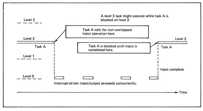
$\vec{x}$  Figure 57. Effect of non-overlapped input/output on task execution (2 of 2)
