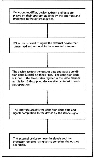
Figure 105. Data bus output sequence (1 of 2)
