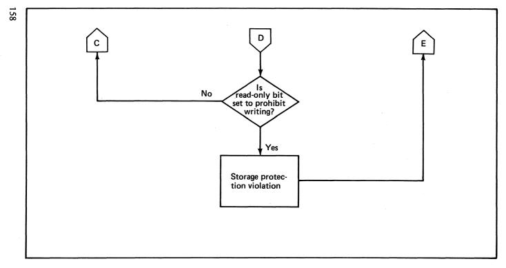
Figure 39. Operation of storage protection during an access (3 of 3)
