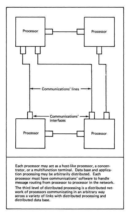
Figure 113. A network of processors
