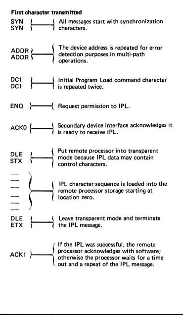
Figure 122. Example of a message exchange containing an Initial Program Load command and acknowledgement
