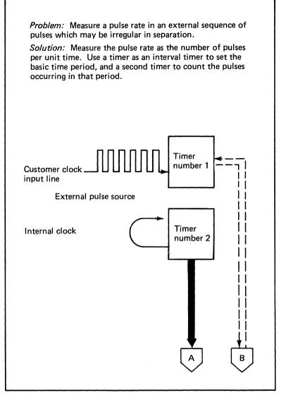
Figure 96. Pulse rate measurement using a pair of timers (1 of 2)
