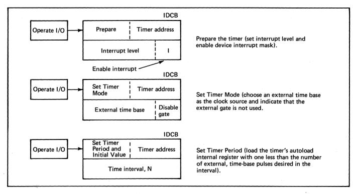
Figure 95. Using the timer to provide interval timing to the processor (2 of 3)
