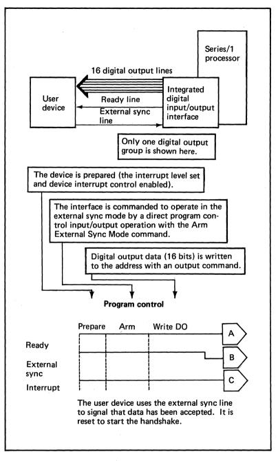
Figure 101. The handshake convention used on digital group output (part 1) (1 of 2)
