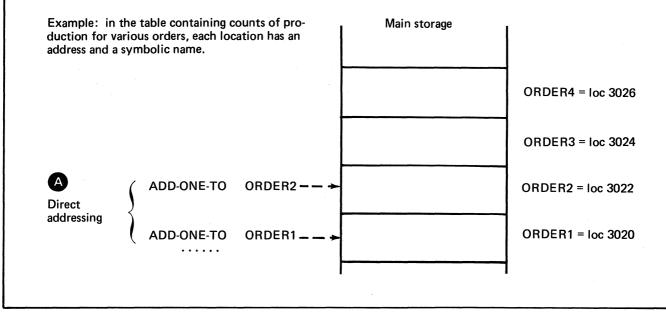
Figure 32. Storage addressing modes which do not use registers (1 of 3)
