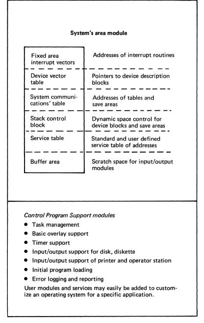
Figure 74. Organization of main storage for a dedicated application utilizing the Control Program Support package (2 of 2)
