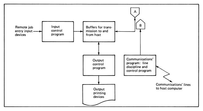
$\vec{\omega}$  Figure 3. Multiple cooperating programs for the multifunction terminal application (2 of 3)
