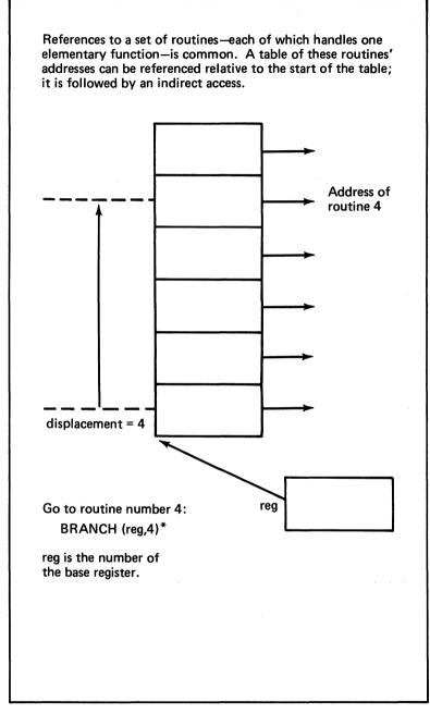
Figure 36. Combined base relative and indirect addressing mode solutions to programming problems (1 of 2)
