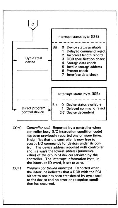
Figure 63. Condition codes accompanying each input/output interrupt (4 of 5)
