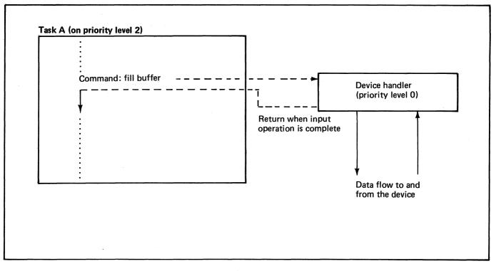
Figure 57. Effect of non-overlapped input/output on task execution (1 of 2)
