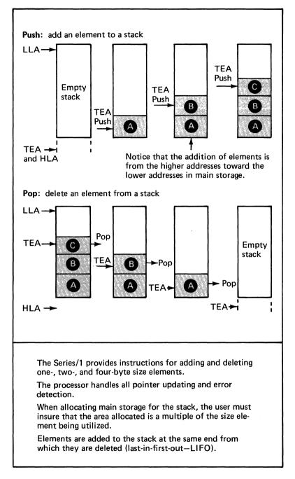
Figure 27. Adding and deleting elements from a stack
