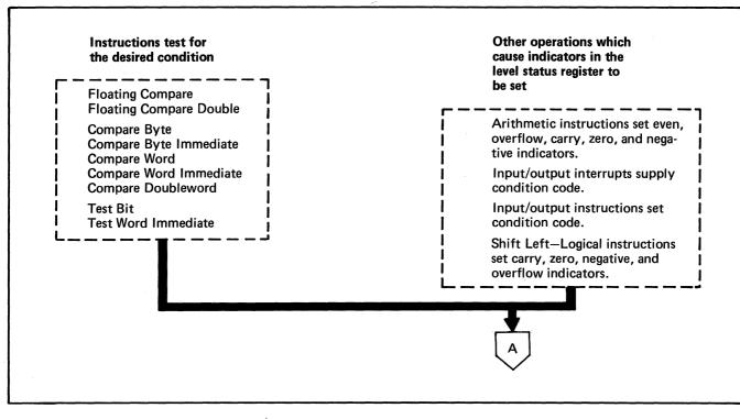
Figure 83. Operation and computation testing instructions (1 of 3)
