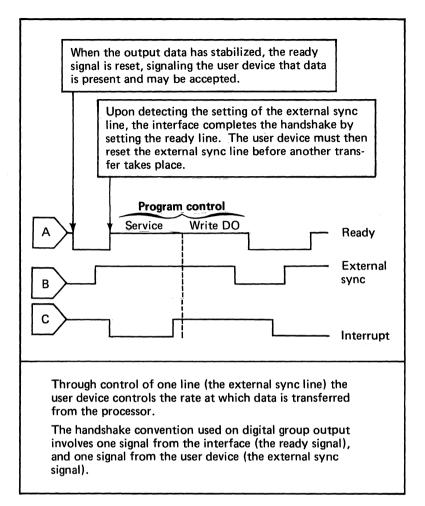
Figure 101. The handshake convention used on digital group output (part 1) (2 of 2)
