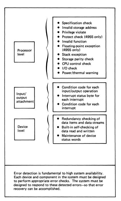
Figure 133. Elements of error detection
