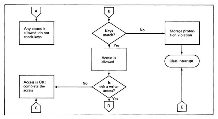
$r_{1}^{h}$  Figure 39. Operation of storage protection during an access (2 of 3)
