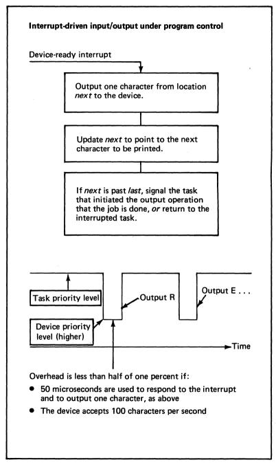
Figure 56. Direct program control of devices (3 of 3)
