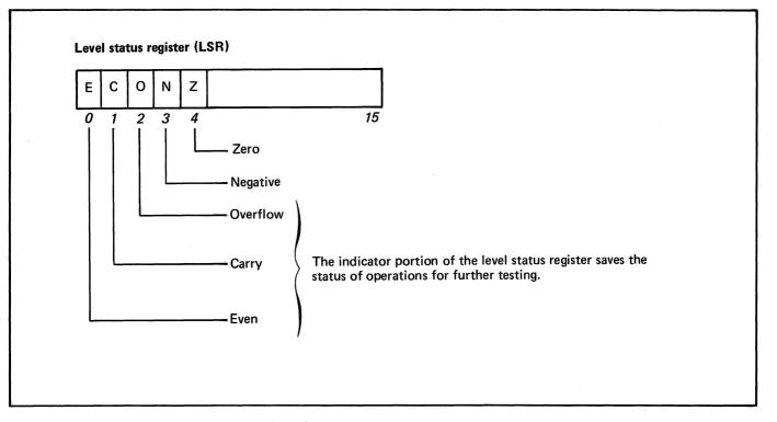
Figure 21. Indicator set in the level status register (1 of 2)
