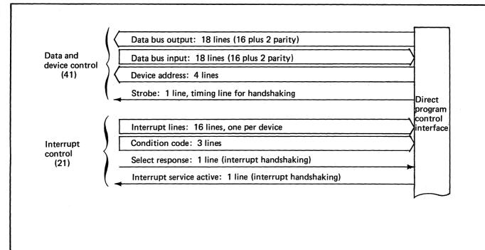
Figure 104. The direct program control interface bus (1 of 2)
