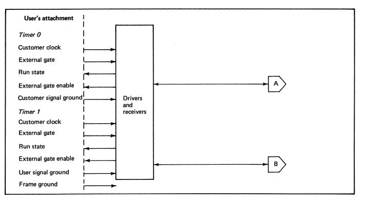
Figure 94. Block diagram of the timers showing their input/output channel connections and external signals for special uses (2 of 3)
