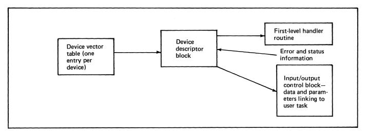
Figure 72. Input/output functions available in the Control Program Support package (2 of 2)
