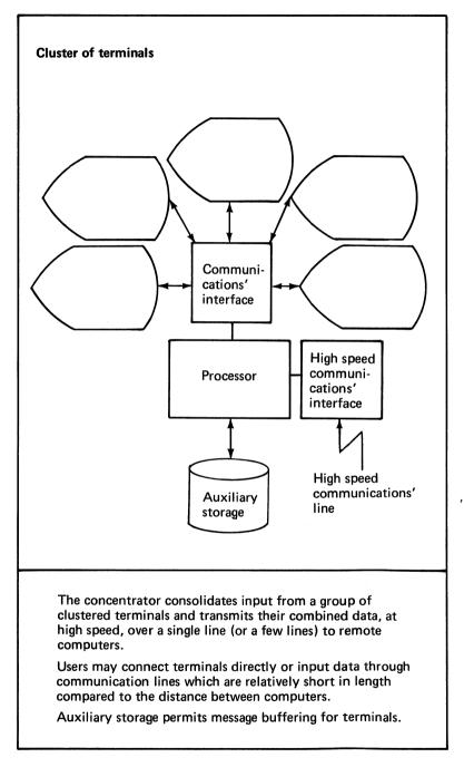
Figure 4. Concentrator configuration
