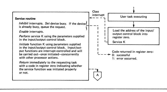
Figure 71. Overlapping and non-overlapping of input/output control (1 of 2)
