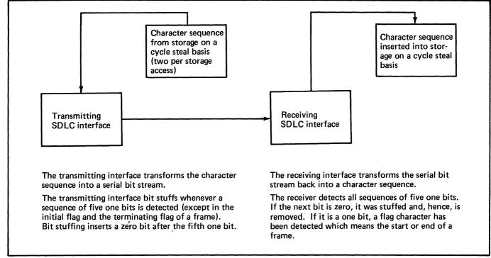
Figure 125. Bit stuffing (1 of 2)
