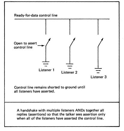
Figure 110. Data transfers with multiple listeners
