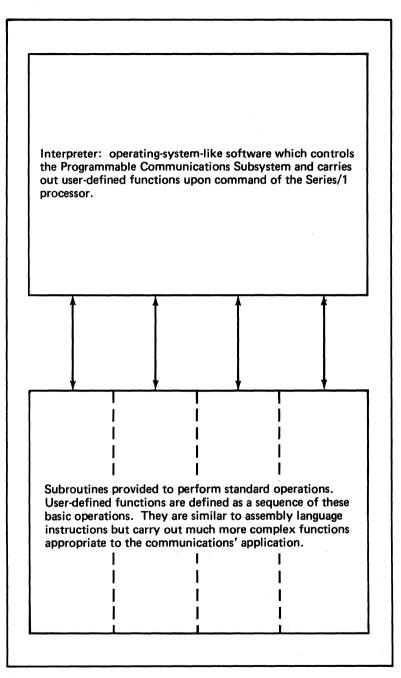
Figure 130. Software organization within the Programmable Communications Subsystem (1 of 2)
