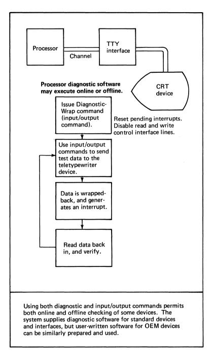
Figure 138. Teletypewriter interface design
