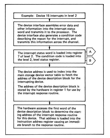
Figure 63. Condition codes accompanying each input/output interrupt (1 of 5)
