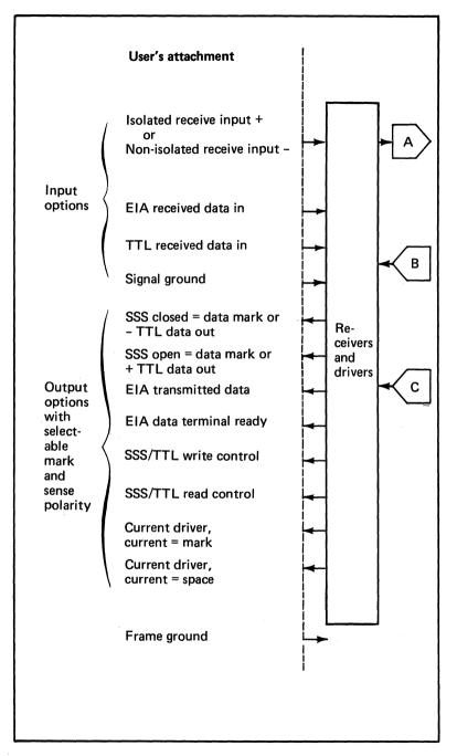
Figure 99. The teletypewriter interface block diagram (1 of 4)
