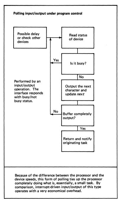
Figure 56. Direct program control of devices (2 of 3)
