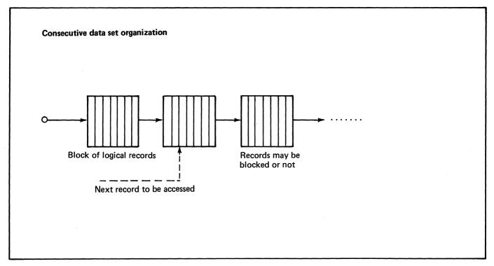
Figure 75. Four data set organizations supported under the Realtime Programming System (1 of 5)
