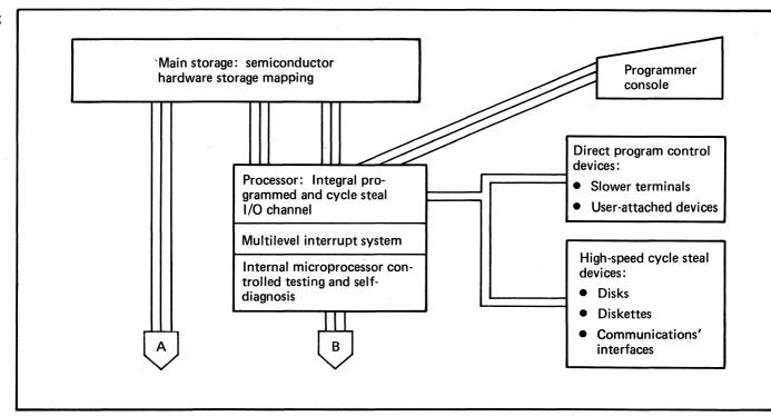
Figure 9. IBM Series/1: an integrated system of hardware, software and maintenance elements (1 of 3)
