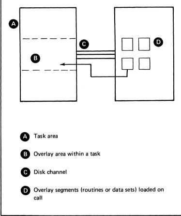
Figure 50. Overlay methods of storage management (1 of 2)
