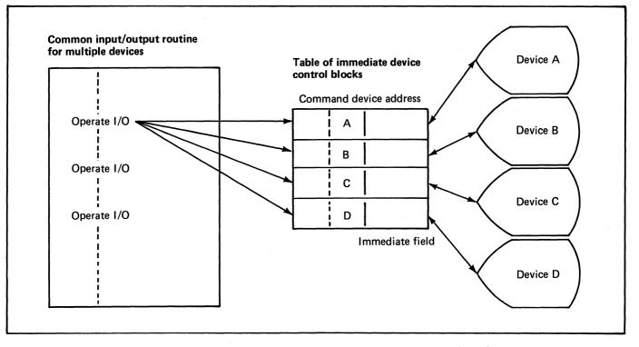
Figure 64. A common input/output control routine addressing different immediate device control blocks (1 of 2)
