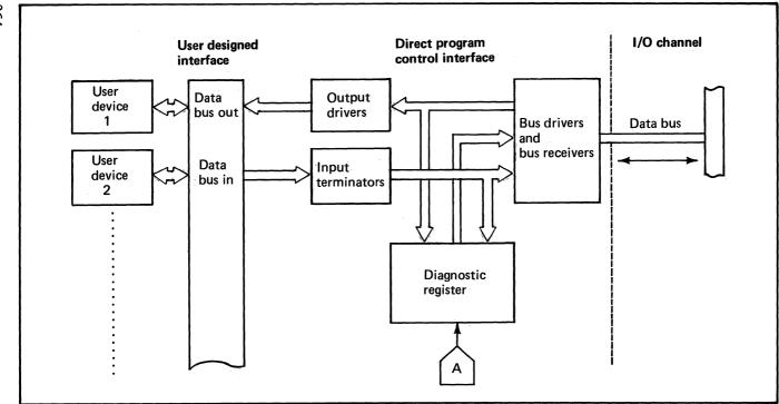
Figure 103. Block diagram of the OEM interface (1 of 3)
