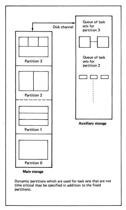
Figure 49. The Realtime Programming System storage management (2 of 2)
