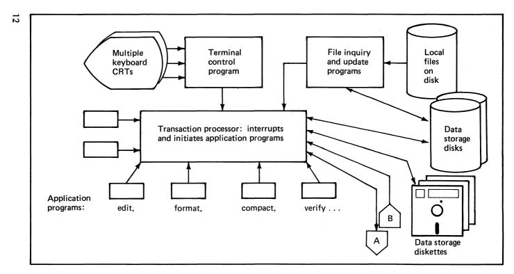
Figure 3. Multiple cooperating programs for the multifunction terminal application (1 of 3)
