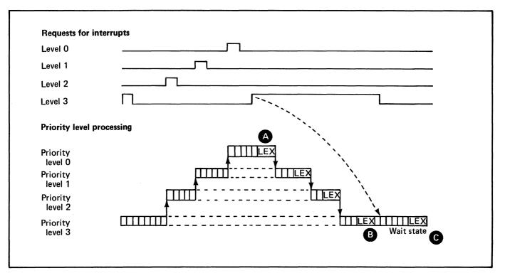
Figure 24. Multilevel priority interrupt response (1 of 2)
