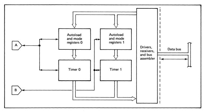
Show Figure 94. Block diagram of the timers showing their input/output channel connections and external signals for special uses (3 of 3)
