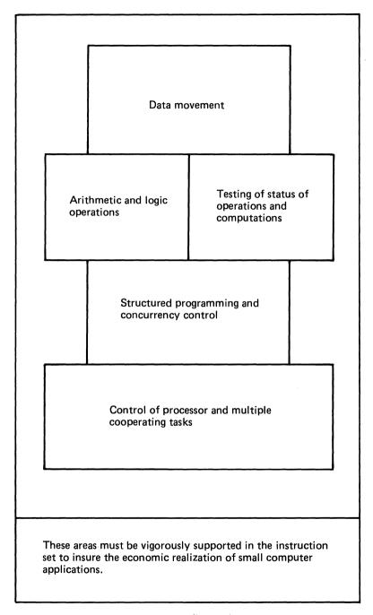
Figure 76. The five areas into which the instruction set can be classified
