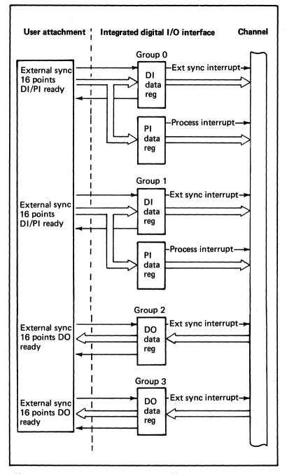
Figure 100. Integrated digital input and output interface (1 of 2)
