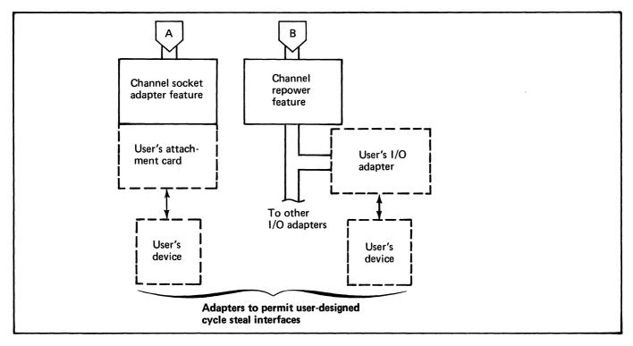
Figure 93. Options for user attachments to the Series/1 (2 of 2)
