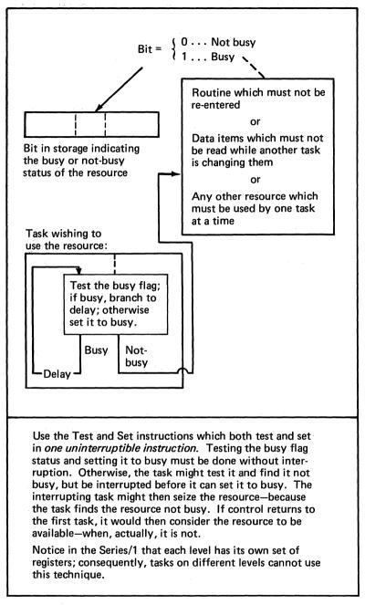
Figure 88. Serializing the use of a resource using the Test and Set type of instruction
