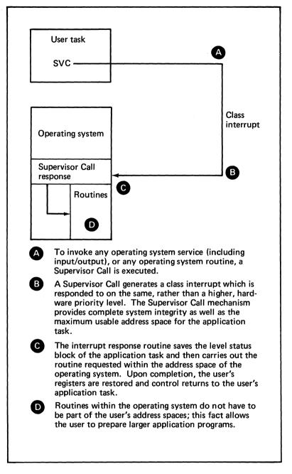
Figure 46. Communications between an application task and the operating system via supervisor calls which generate a class interrupt
