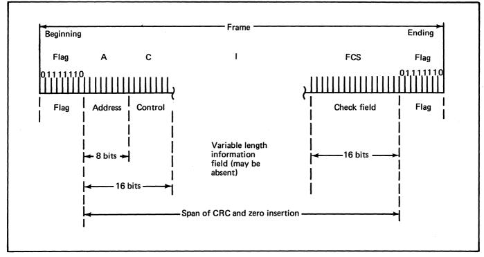
Figure 124. Detailed definition of the SDLC frame format (1 of 2)
