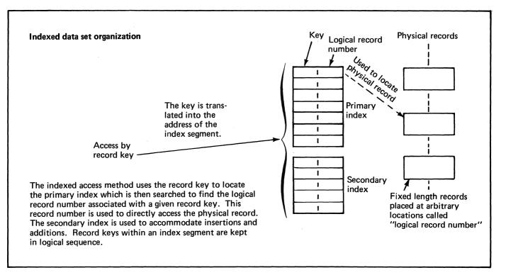
Figure 75. Four data set organizations supported under the Realtime Programming System (3 of 5)
