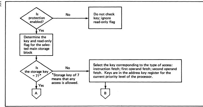
Figure 39. Operation of storage protection during an access (1 of 3)
