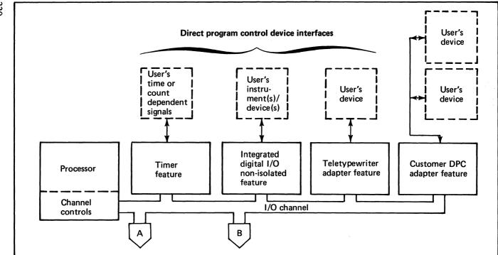
Figure 93. Options for user attachments to the Series/1 (1 of 2)
