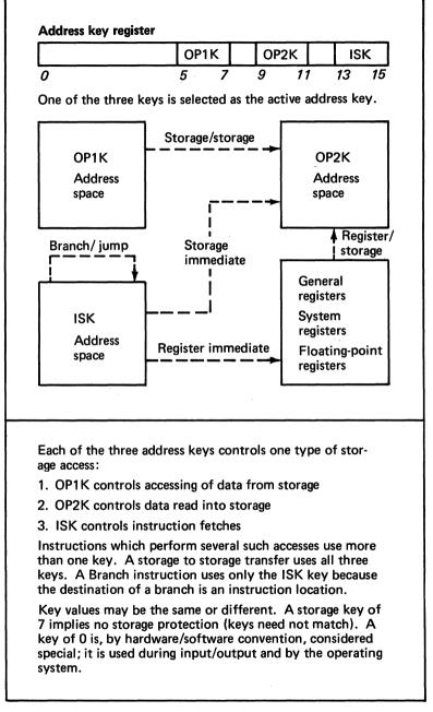
Figure 40. Use of the three storage protection keys by various classes of operations
