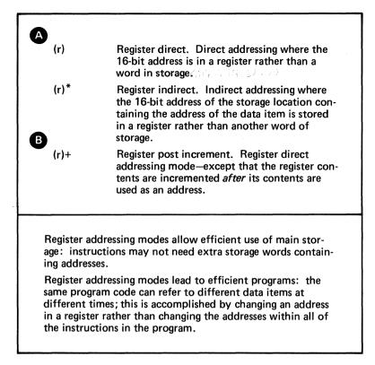
Figure 33. Storage addressing modes using registers for address storage (1 of 2)
