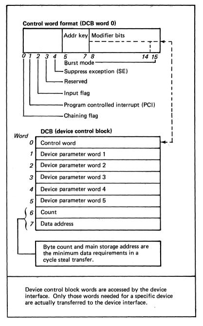
Figure 67. The device control block contains the data necessary to carry out one transfer between a specific device and main storage (1 of 2)
