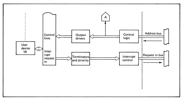
Figure 103. Block diagram of the OEM interface (2 of 3)
