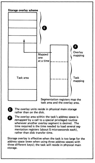
Figure 50. Overlay methods of storage management (2 of 2)
