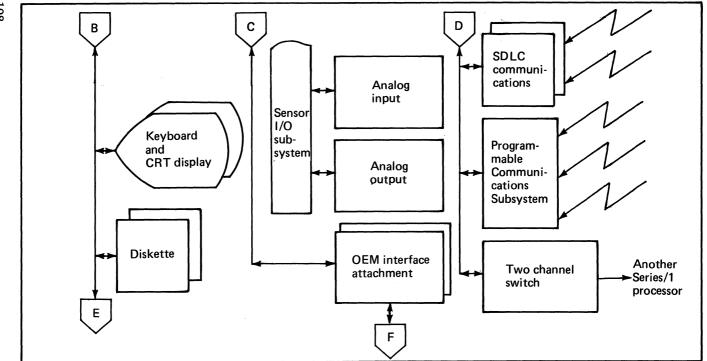
Figure 52. Input/output device combinations (3 of 4)
