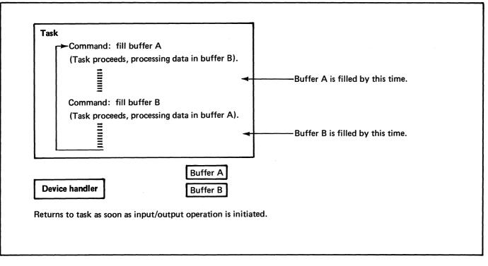
Figure 58. Direct program control and overlapped input/output (1 of 2)
