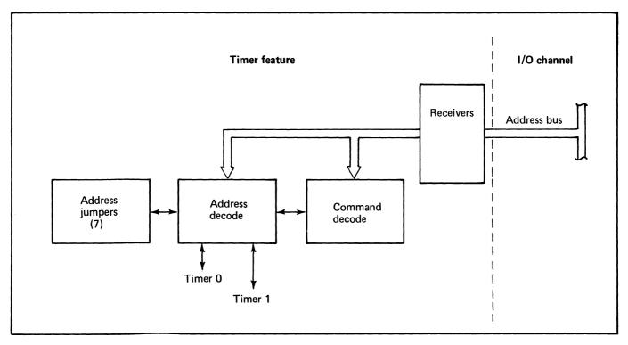
Figure 94. Block diagram of the timers showing their input/output channel connections and external signals for special uses (1 of 3)
