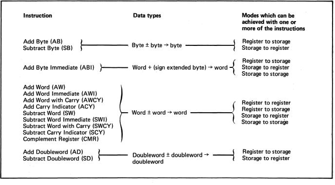
Figure 80. Arithmetic operations, data types, and modes (1 of 2)
