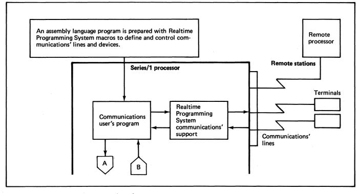
Figure 127. Software use of communications (1 of 2)
