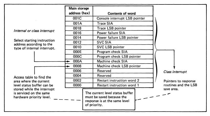
Figure 23. Input/output and class interrupts and the response of the processor (2 of 2)
