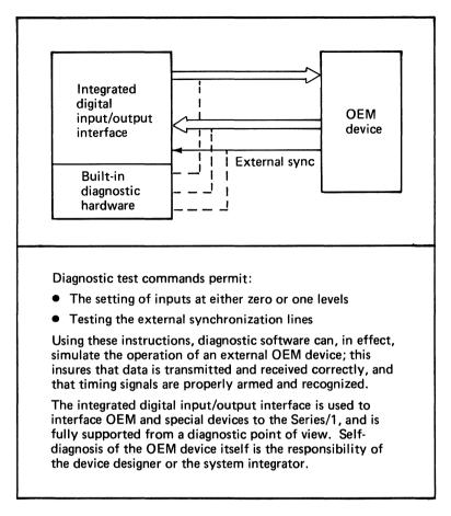
Figure 139. The integrated digital input/output interface
