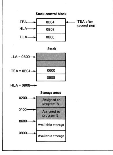
Figure 28. Example of stack usage: allocation of storage areas to concurrent programs (3 of 4)
