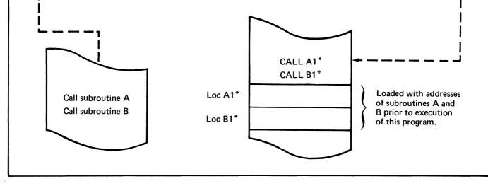
Figure 32. Storage addressing modes which do not use registers (3 of 3)
