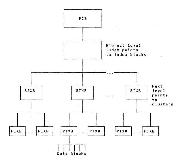
Note that only the highest key in any data block is found in a PIXB entry, a SIXB entry contains only the highest key found in a PIXB, and so on, to the highest index block. This index technique is called <u>sparse indexing</u>.
