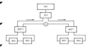
The 3653's on 3659# 1 have CRC errors in the 3651, i.e. the data transmitted from the 3653 has to go through the degradation and therefore gets corrupted.
