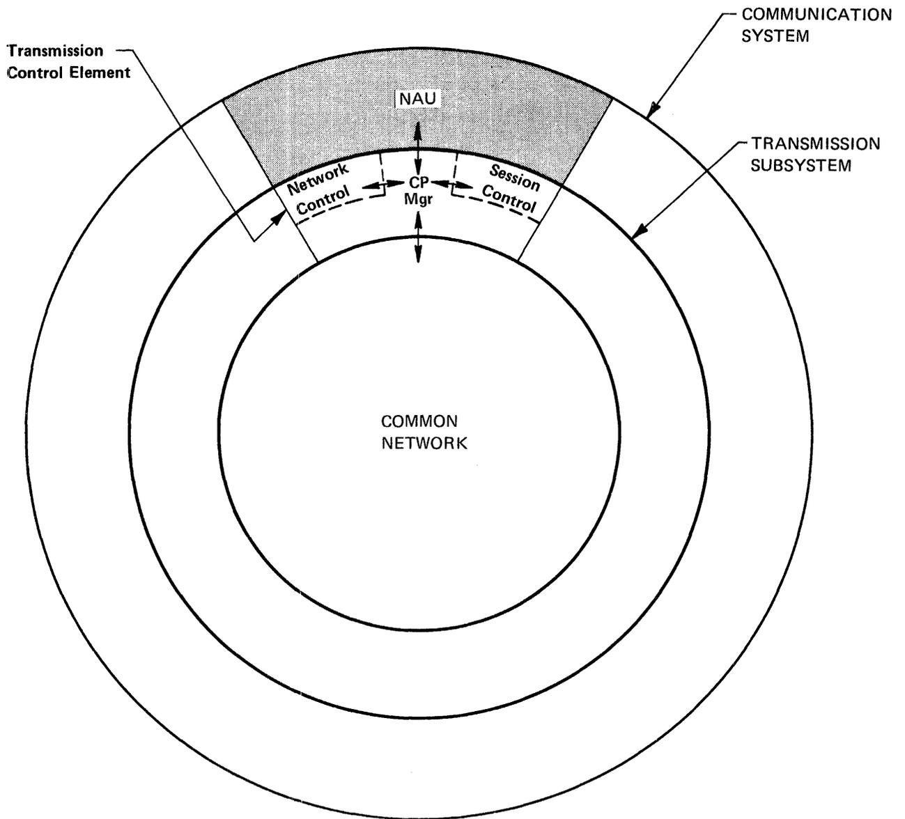
Figure 2-7. Transmission Control Element
