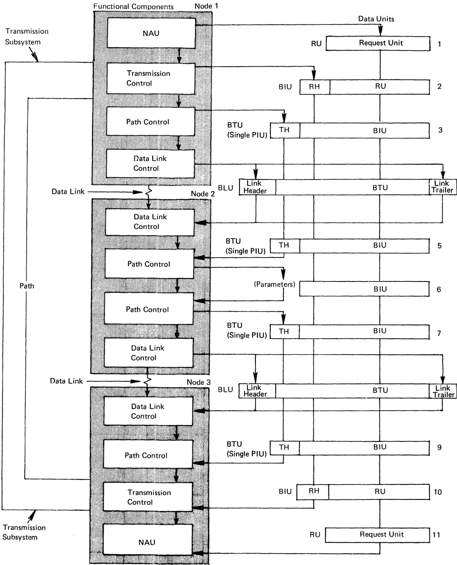
Figure 2-12. Transmission Subsystem Control Data Flow
