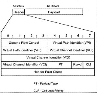
be discarded during times of network congestion. The entire cell header is error checked by the Header Error Control Field. The header is error checked to ensure that cells are not misdirected, but the payload is not error checked. The integrity of the information in the payload is the responsibility of the network users.
