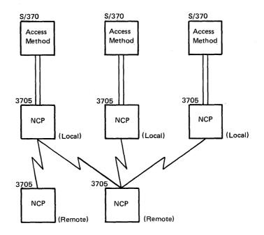
Figure 6-3. NCP in Remote 3705 Communicating with Multiple Access Methods via Cross-Domain Links to NCPs in Local 3705s
