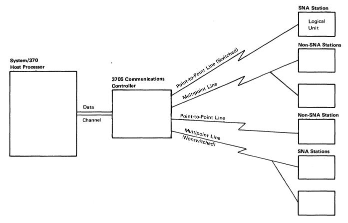
Figure 1-2. Network Showing Communication Lines and One Communications Controller
