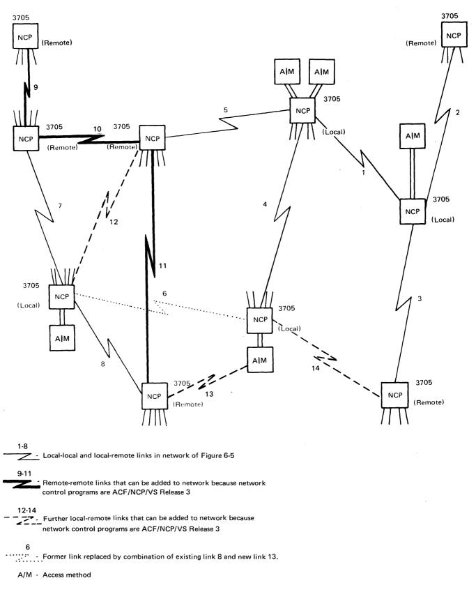
Figure 6-6. Example of a Network Controlled by ACF/NCP/VS Release 3
