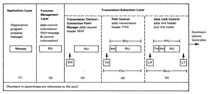
Figure 2-2. Data Flow through Network Layers
