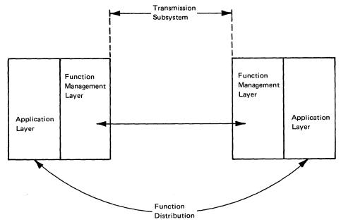
Figure 2-1. The Transmission Subsystem as the Innermost Layer of a Network
