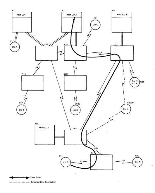
Figure 3-13. Data Flow through an Intervening Domain
