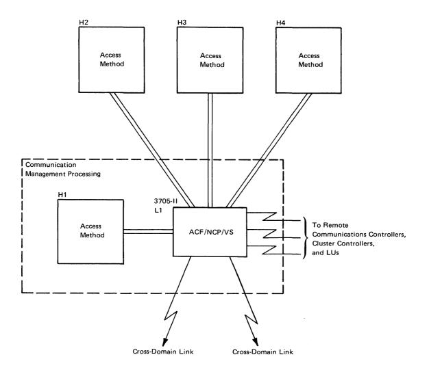
Figure 3-15. Possible Implementation of a Communication Management Configuration
