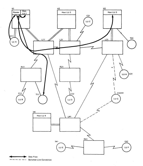
Figure 3-14. Use of a Router or Message Handler
