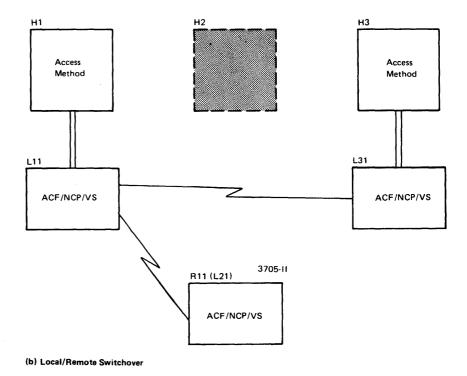
Figure 3-16. Recovery from Host Processor Failures
