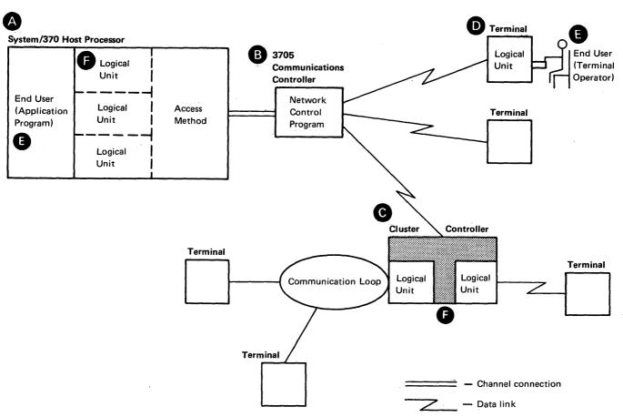
Figure 1-1. Example of a Data Communication Network
