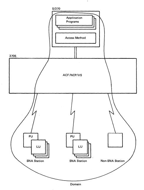
Figure 2-3. ACF/NCP/VS in a Single-Domain Network
