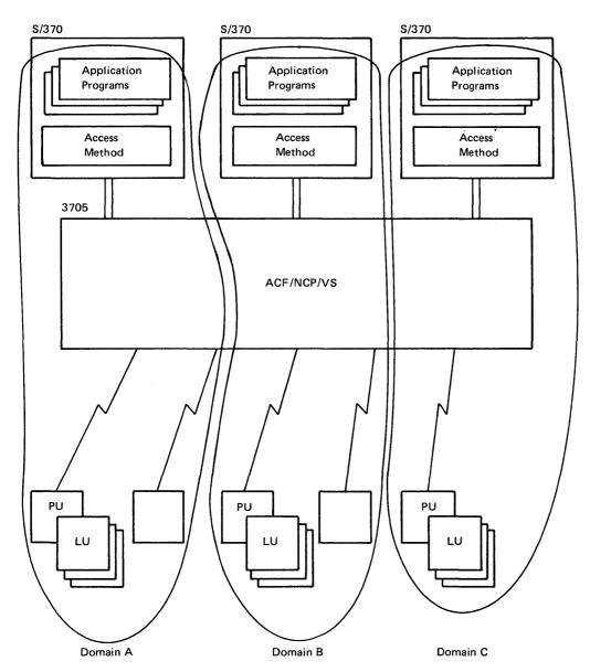
Figure 2-4. ACF/NCP/VS in Multiple Single-Domain Networks
