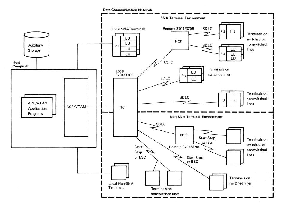
Figure 1-8. The Major Elements in a Single-Domain ACF/VTAM Network
