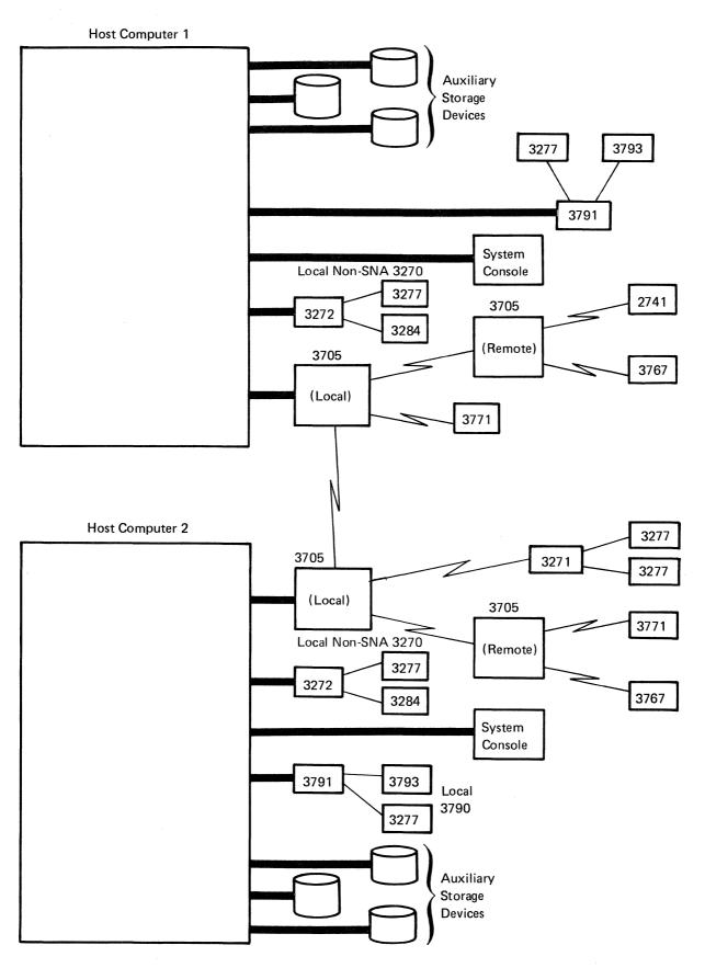
Figure 2-2. Physical Configuration of a Multiple-Domain ACF/VTAM Network
