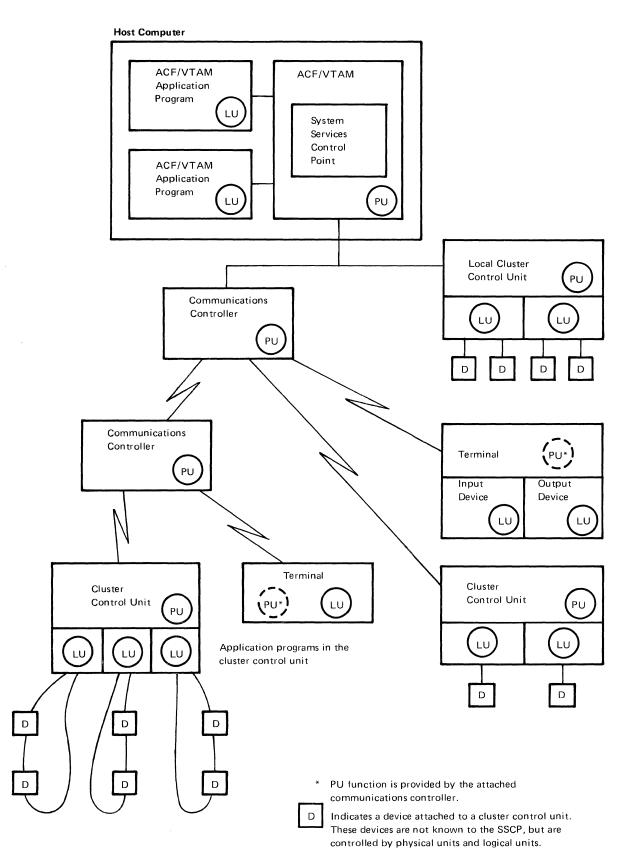
Figure 1-3. The SSCP, Physical Units, and Logical Units in a Network
