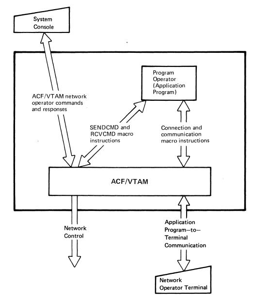
Figure 4-1. Network Operator Control of the ACF/VTAM System
