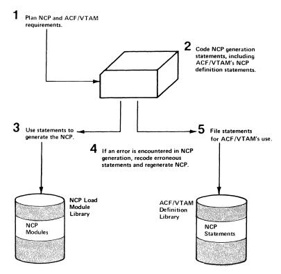
Figure 3-4. Generating NCP Support in an ACF/VTAM System
