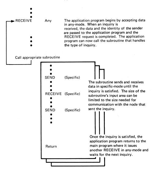
Figure 5-16. Using a Combination of Any-Mode and Specific-Mode
