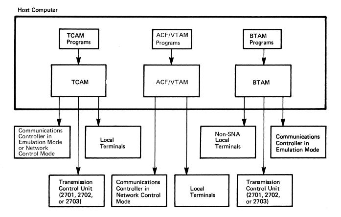
Figure 7-8. Other Telecommunication Access Methods in OS/VS
