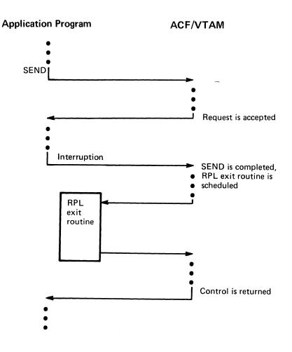
Figure 5-3. Processing Pattern When an RPL Exit Routine is Used with an Asynchronous Request
