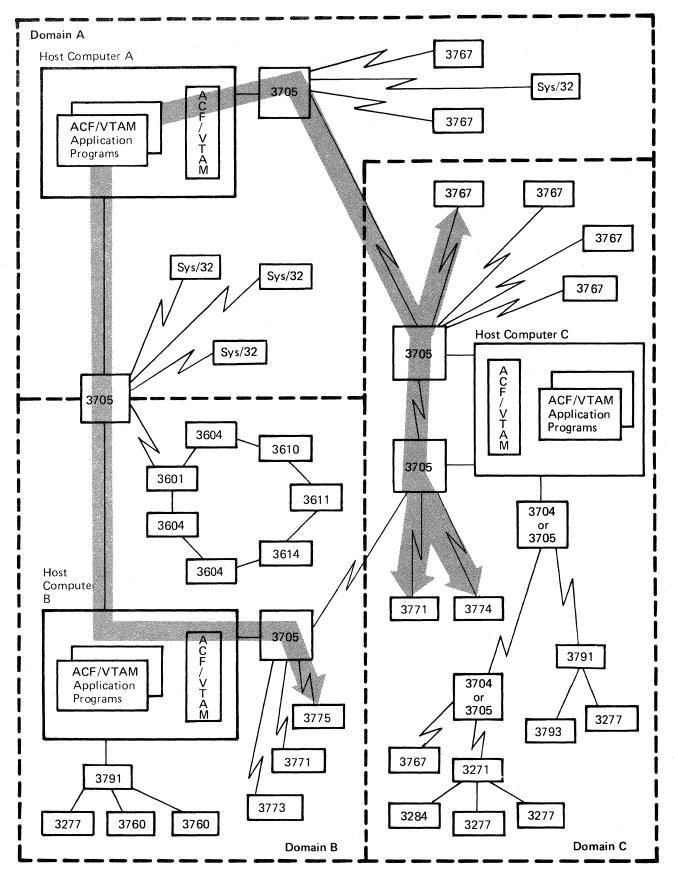
Figure 1-6. Data Flow through a Multiple-Domain ACF/VTAM Network
