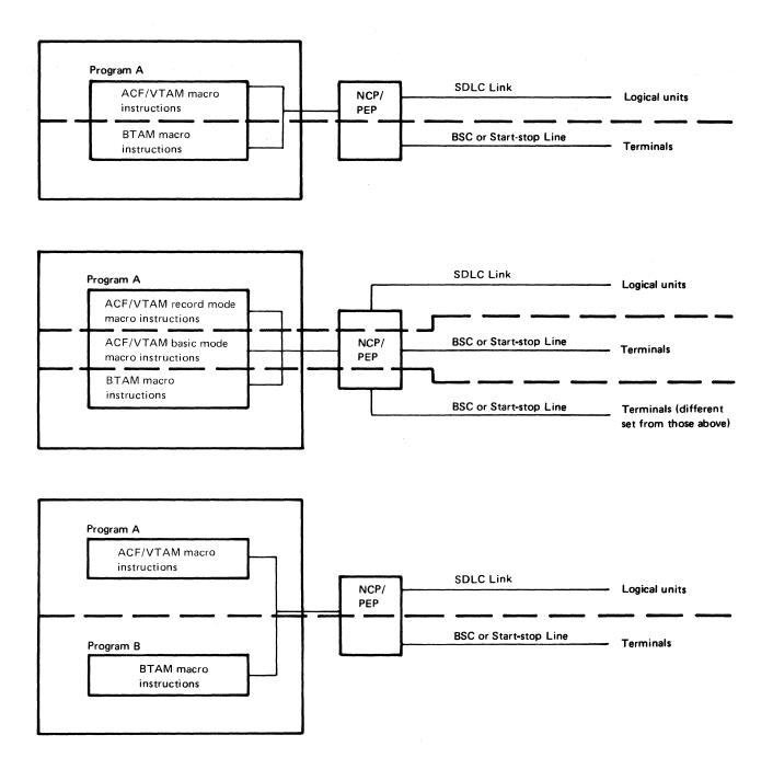
*Notes:* Local and remote 3270 terminals can be communicated with using ACF/VTAM record-mode macro instructions, ACF/VTAM basic-mode macro instructions, or BTAM macro instructions. Using ACF/VTAM record mode allows logical units and 3270s to be communicated with using the same set of macro instructions.
