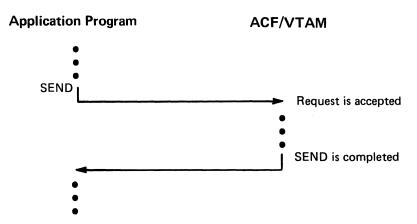
Figure 5-1. Processing Pattern for a Synchronous Request
