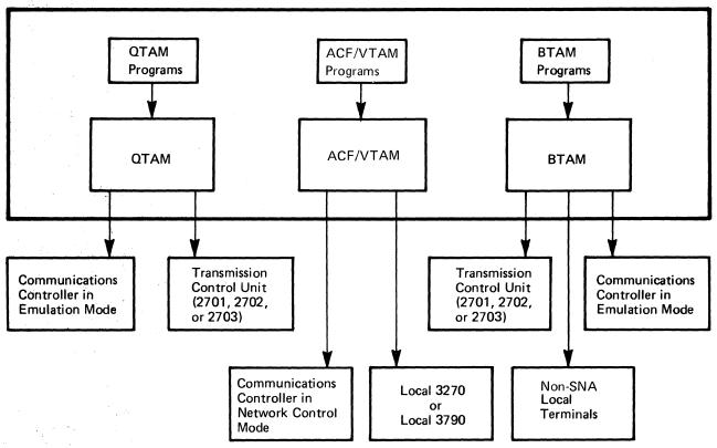
Figure 7-7. Other Telecommunication Access Methods in DOS/VS
