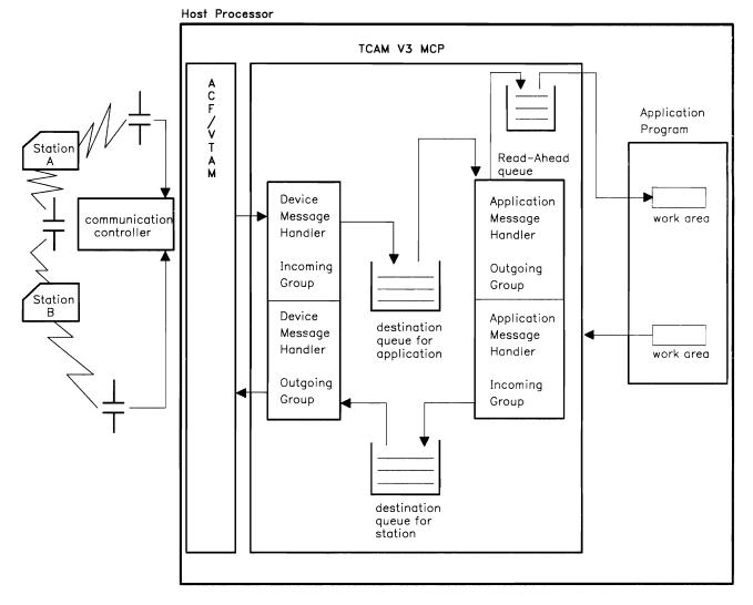
Figure 1-1. TCAM in a Network
