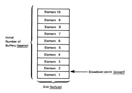
This example shows a pool for which the start options were specified as <u>poolname=(10,bufsize,1)</u>. The initial number of buffers in the pool is 10, the slowdown point is set at 1, and the <u>bufsize</u> is the length in bytes of each buffer in the pool.
