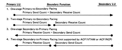
Figure 2-2. Pacing Counts Used to Control One and Two Stage Pacing
