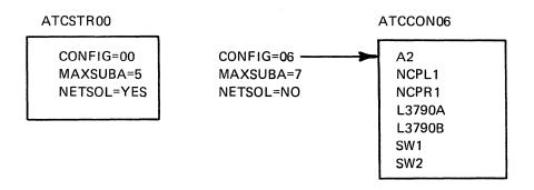
Example C. The network operator enters the START command with the start option LIST=ST. LIST=ST refers to ATCSTRST, which contains a sets of start options. The same configuration and start options are obtained as in Example B. The result is:
