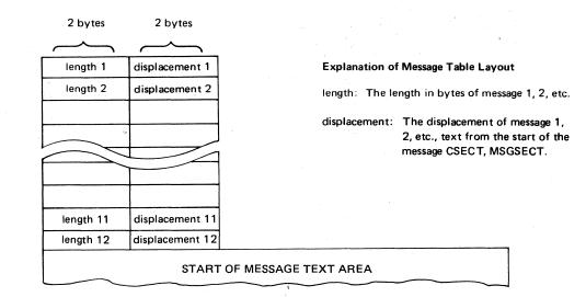
The control section that defines the IBM-supplied message texts is shown below:
