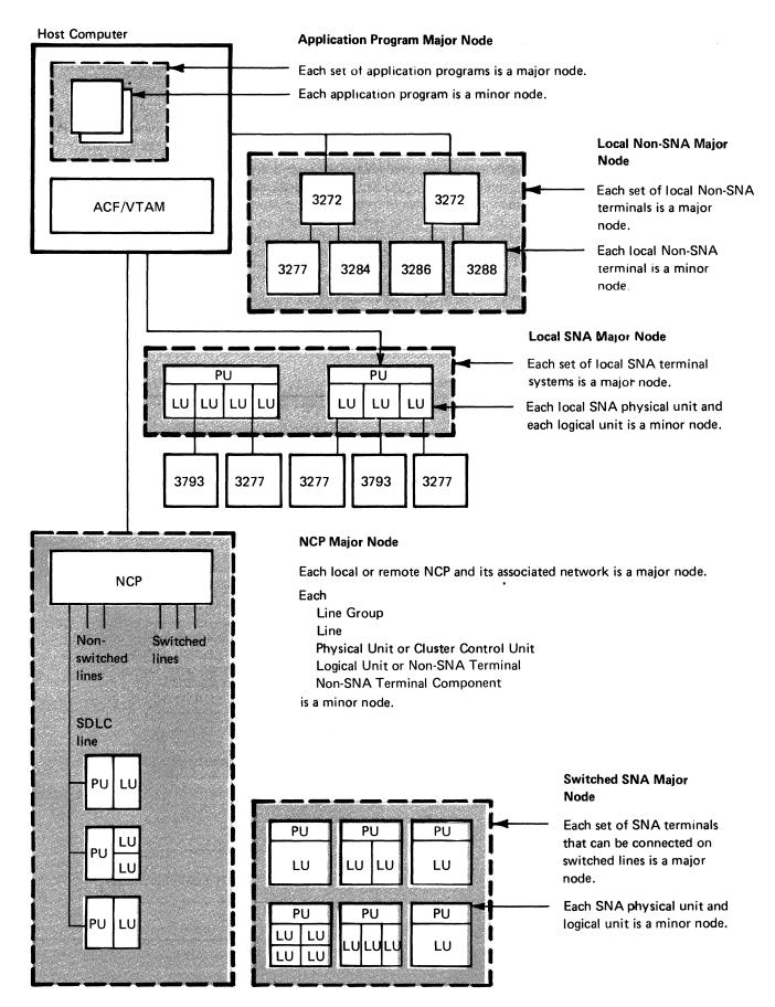
Figure 1-1. Major and Minor Nodes in a Single-Domain ACF/VTAM System
