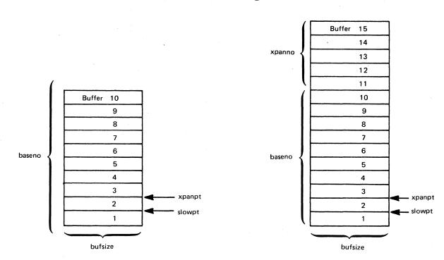
(A) This example shows a buffer pool for which the start options were specified as poolname=((10,bufsize,,1,5,2). After initial allocation, the pool contains 10 buffers (baseno=10), the length in bytes of each buffer is buffsize, the slowdown point is 1, the expansion size is 5 buffers (assume that 5 buffers fill one page of storage), and the expansion point is 1.
