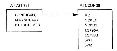
Figure 3-2. Examples of Using CONFIG and LIST Start Options.
