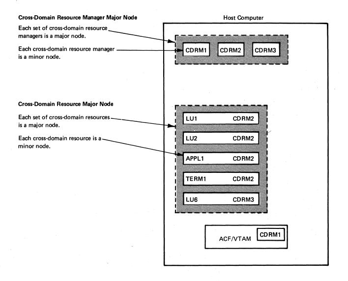
Figure 1-2. Additional Major and Minor Nodes in a Multiple-Domain ACF/VTAM System
