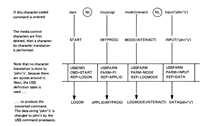
Figure 4-7. Example of Command Conversion
