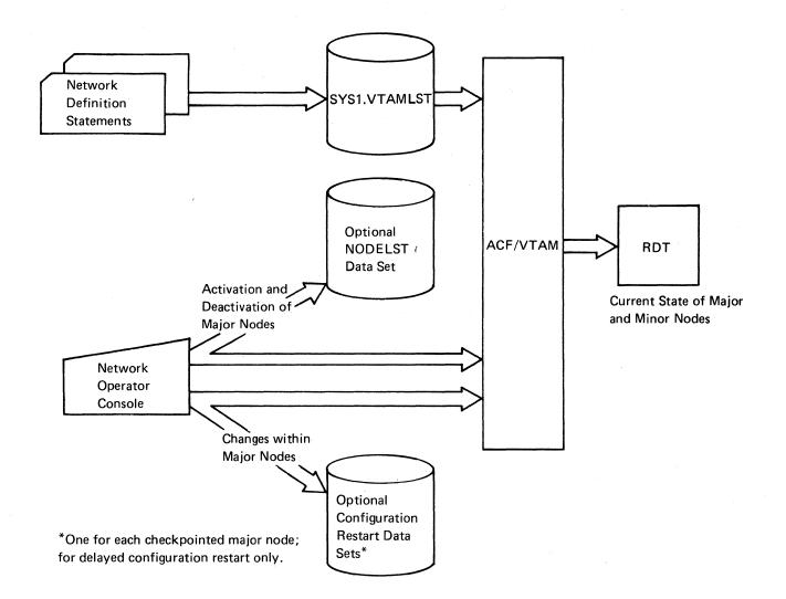
Figure 6-1. Recording Changes to the Network Configuration
