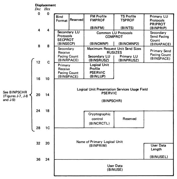
Figure J-4. The Format of BNDAREA (ISTDBIND)
