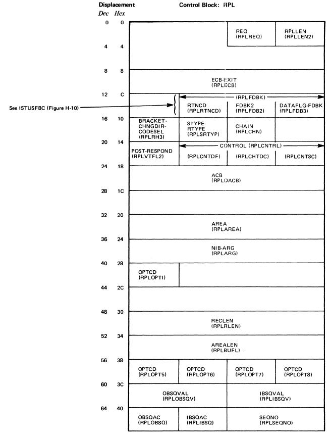
Figure H-8 (Part 1 of 2). The Format of the OS/VS RPL
