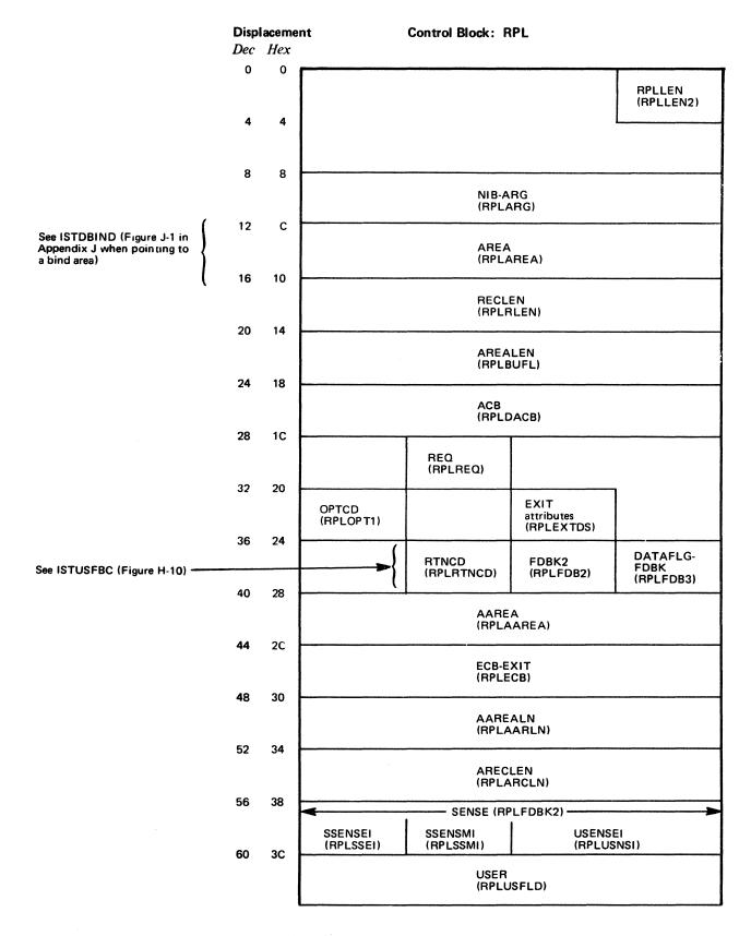
Figure H-7 (Part 1 of 2). The Format of the DOS/VS RPL
