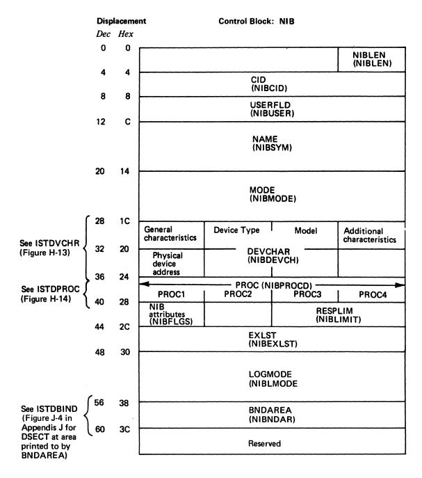
Figure H-11. The Format of the DOS/VS and OS/VS NIB
