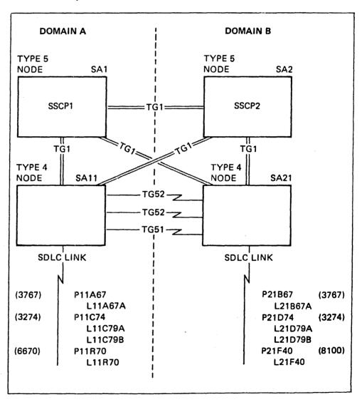
Domains can be connected by SDLC links or by processor channels. Figure 12-2 illustrates the ways that domain A can be connected to domain B.
