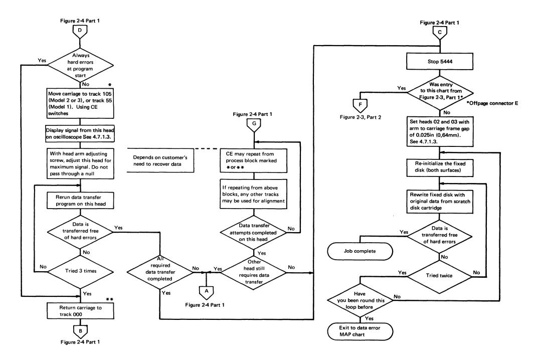
Figure 2-4. Error Recovery Procedure – R/W Head 2 or 3 Replacement (Part 2 of 2) [07530]
