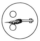
Heavy oxide accumulation in pole tip area cannot be removed
