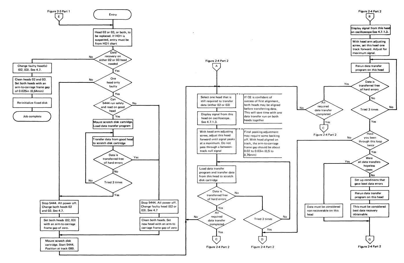
Figure 2-4. Error Recovery Procedure – R/W Head 2 or 3 Replacement (Part 1 of 2) [07501]
