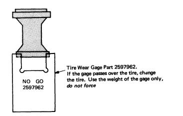
Figure 2-29. Checking Tire Wear [07552]
