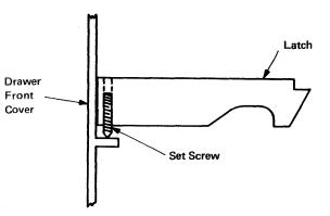
Figure C-2. Drawer Latch Adjustment [07571]
