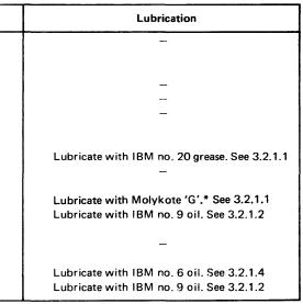
2. This preventive maintenance depends on usage. If the usage exceeds 176 power-on hours per month, perform the maintenace every 1,056 power-on hours.
