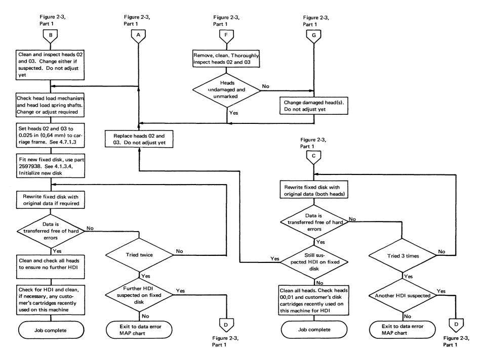
Figure 2-3. Error Recovery Procedure – Suspected HDI on Fixed Disk (Part 2 of 2) [07529]
