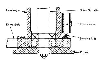
Figure 1-33. Lower Index Transducer [07493]
