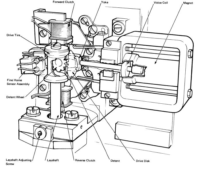
Figure 1-20. Detent Mechanism [07480]
