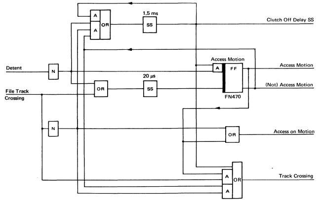
Figure 1-45. Access Control Signals [07506]
