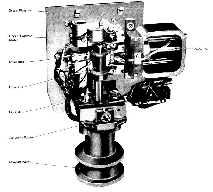
Figure 2-27. Layshaft Assembly (EC Level 391962) [07549]
