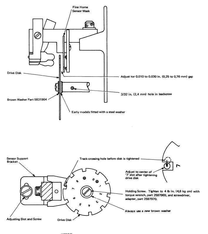
Figure 2-31. Drive Disk Adjustment [07554]
