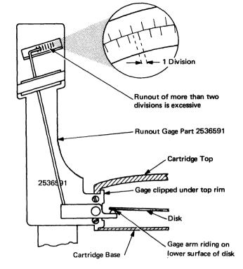
Figure 2-13. Runout Check – Removable Disk [07538]
