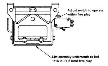
Figure 2-16. Adjusting Cartridge Interlock Switches [07541]
