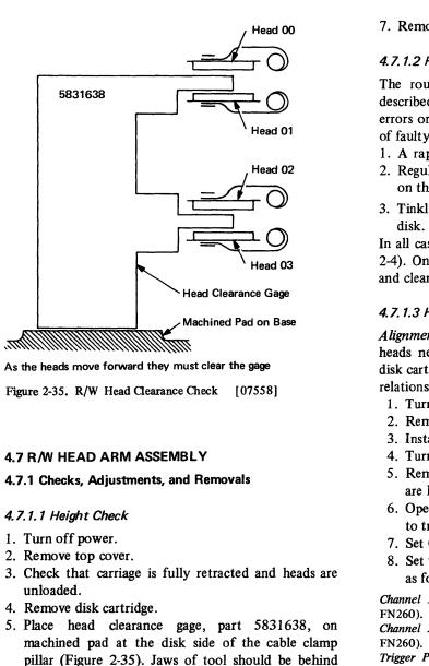
6. Carefully retract carriage and check that the heads clear the jaws of the tool. If a head does not clear the jaws, change the head arm (see 4.7.1.4 and 4.7.1.5) and recheck. If the new head does not clear the jaws, check adjustment of head-load spring shaft (see 4.8.4.1).
