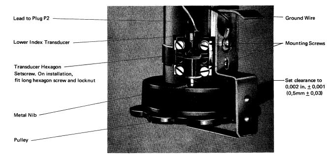
Figure 2-19. Lower Index Transducer [07544]
