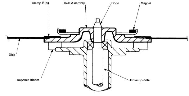
Figure 1-9. Lower Disk Hub Assembly [07469]
