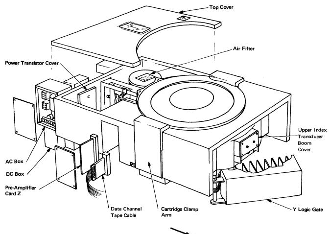
Figure 2-46. Front Top View of 5444 – Locations [07566]
