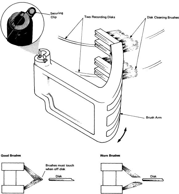
Figure 1-13. Cartridge Handle and Release Catch [07473]
