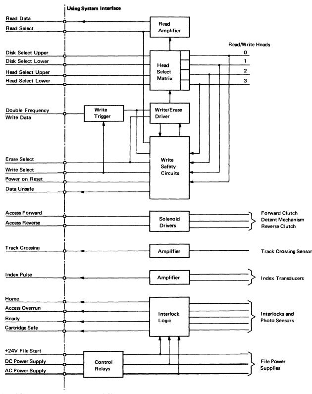
Figure 1-39. Data Flow and Control [07499]
