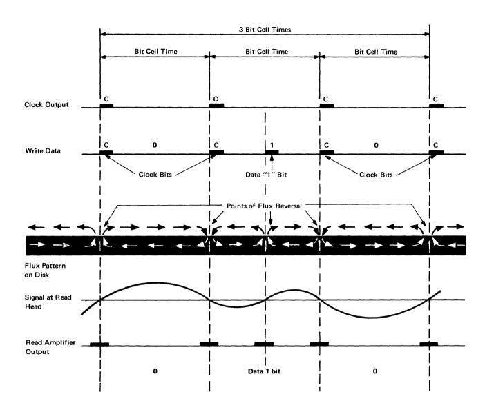
Figure 1-57. Double Frequency Recording – Flux and Pulse Relationship [07518]
