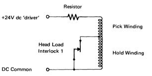
Figure 1-27. Head Load Solenoid Circuit [07487]
