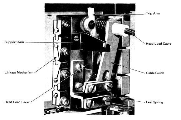
Figure 1-28. Knock-Off Mechanism [07488]
