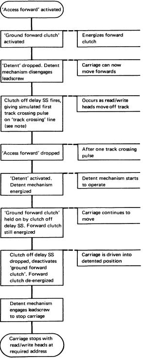
Note: The simulated track crossing pulse is an extra pulse which is required because the detent mechanism takes one track to operate; without this extra pulse the carriage would stop at the wrong track.
