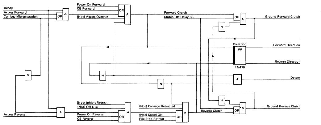
Figure 1-44. Clutch and Detent Signals [07505]
