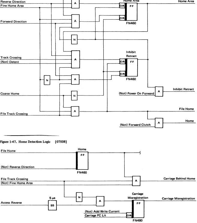
Figure 1-48. Head Movement Error Logic [07509]
