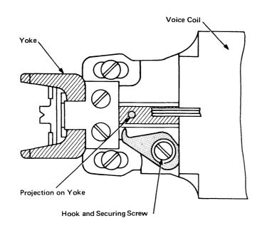
Figure 2-6. Yoke Holdout Hook [07531]
