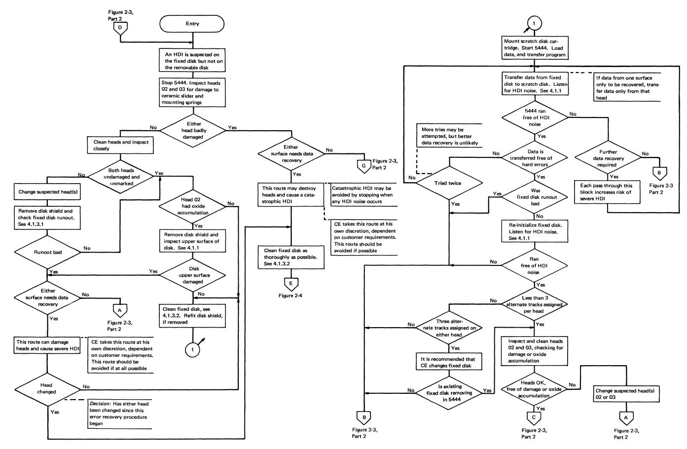
Figure 2-3. Error Recovery Procedure – Suspected HDI on Fixed Disk (Part 1 of 2) [07528]
