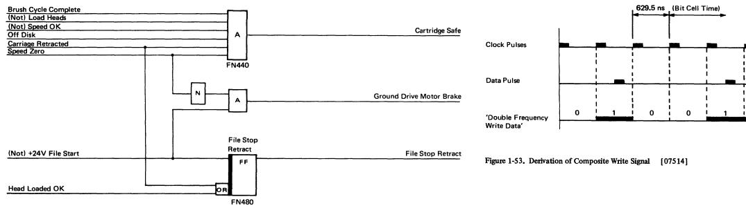
Figure 1-51. Machine Stop Logic [07512]
