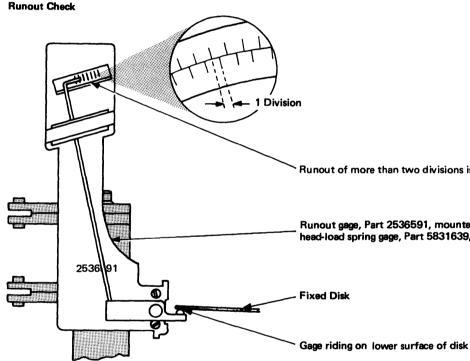
Figure 2-14. Disk Height and Runout Checks – Fixed Disk [07539]
