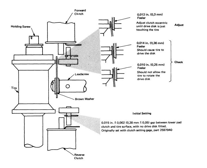
Remove the tire holding screw and withdraw the tire **4.5** assembly. Take care not to damage the drive disk.
