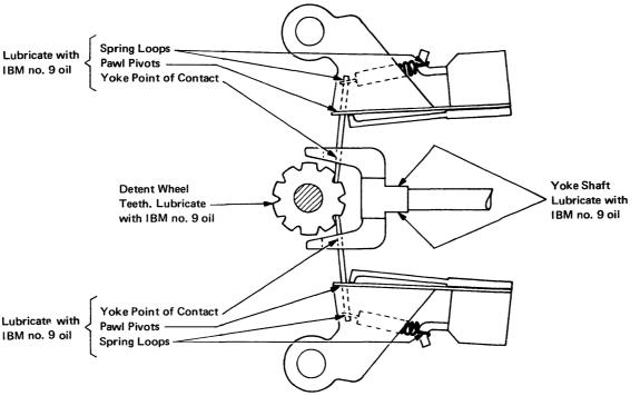
Figure 2-10. Detent Assembly Lubrication [07534]
