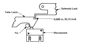
Figure C-1. False Latch Setup [07570]
