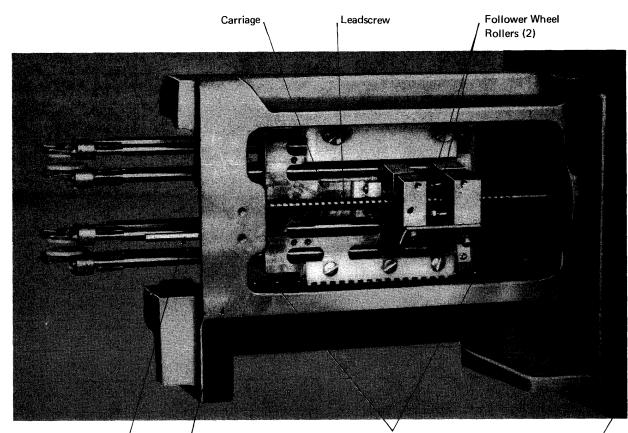
Actuator Frame Inner Limit Stop Shaft Figure 2-25. Actuator Carriage Assembly [07478]
