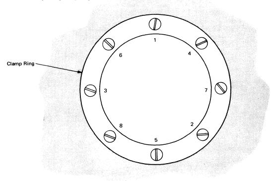
Figure 2-15. Replacement Details – New Fixed Disk [07540]
