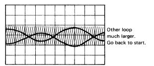
Figure 2-36. Head Arm Alignment, using CE Cartridge Track 073 [07559]
