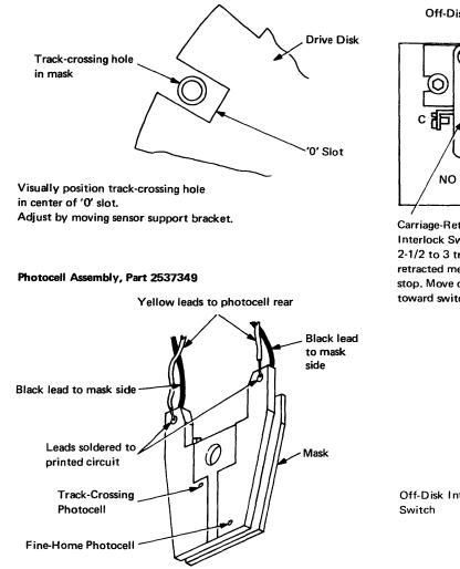
Figure 2-32. Photocell Assembly – Adjustment and Details [07555]
