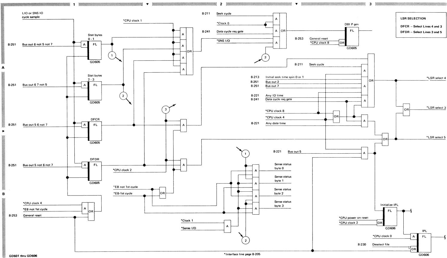
storage register or core. The constant may also be entered into these locations without change. A cycle steal request is started when one of the inputs to the 'condition prior request' latch is active, and gated by a final condition, 'bit ring 7 and phase C'. The remainder of the cycle steal request is as follows:
