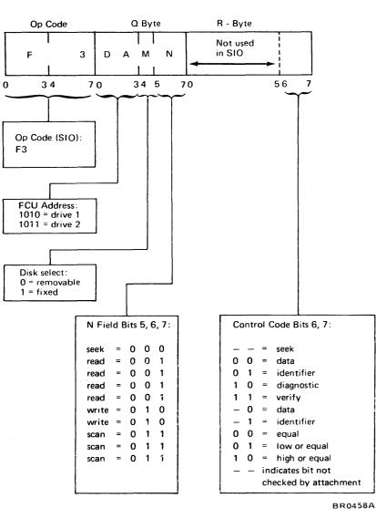
There are four basic disk operations: write, read, scan, and seek. These are further defined into twelve specific operations.
