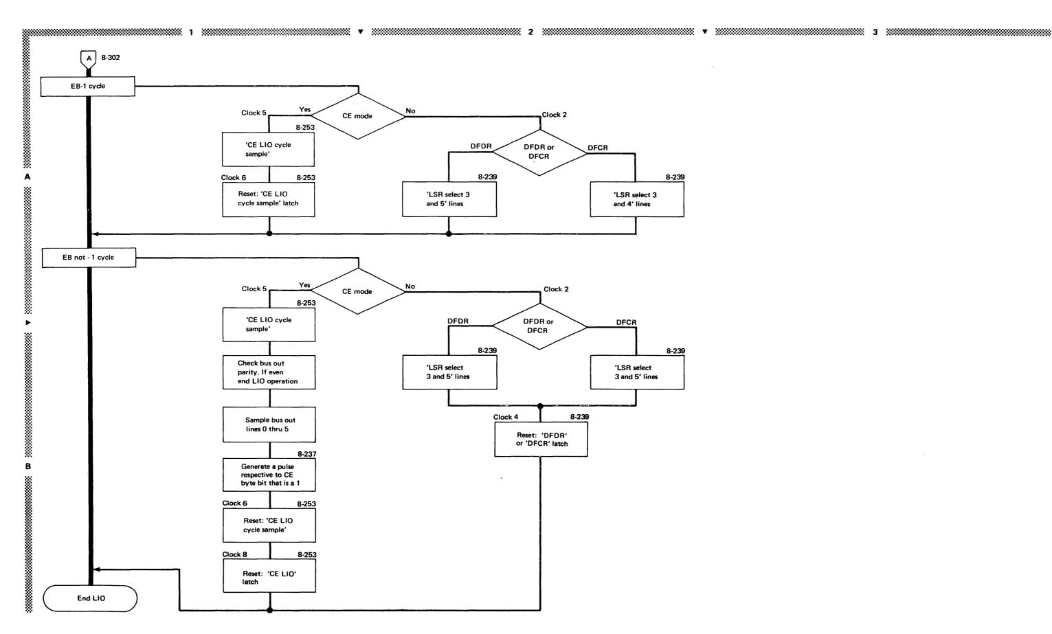
**DISK ATTACHMENT-Operations** Load I/O Operation (Part 2 of 2)
