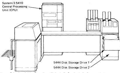
Note: Drive 1 and drive 2 are also called spindle 0 and spindle 1, respectively. BR0442A
