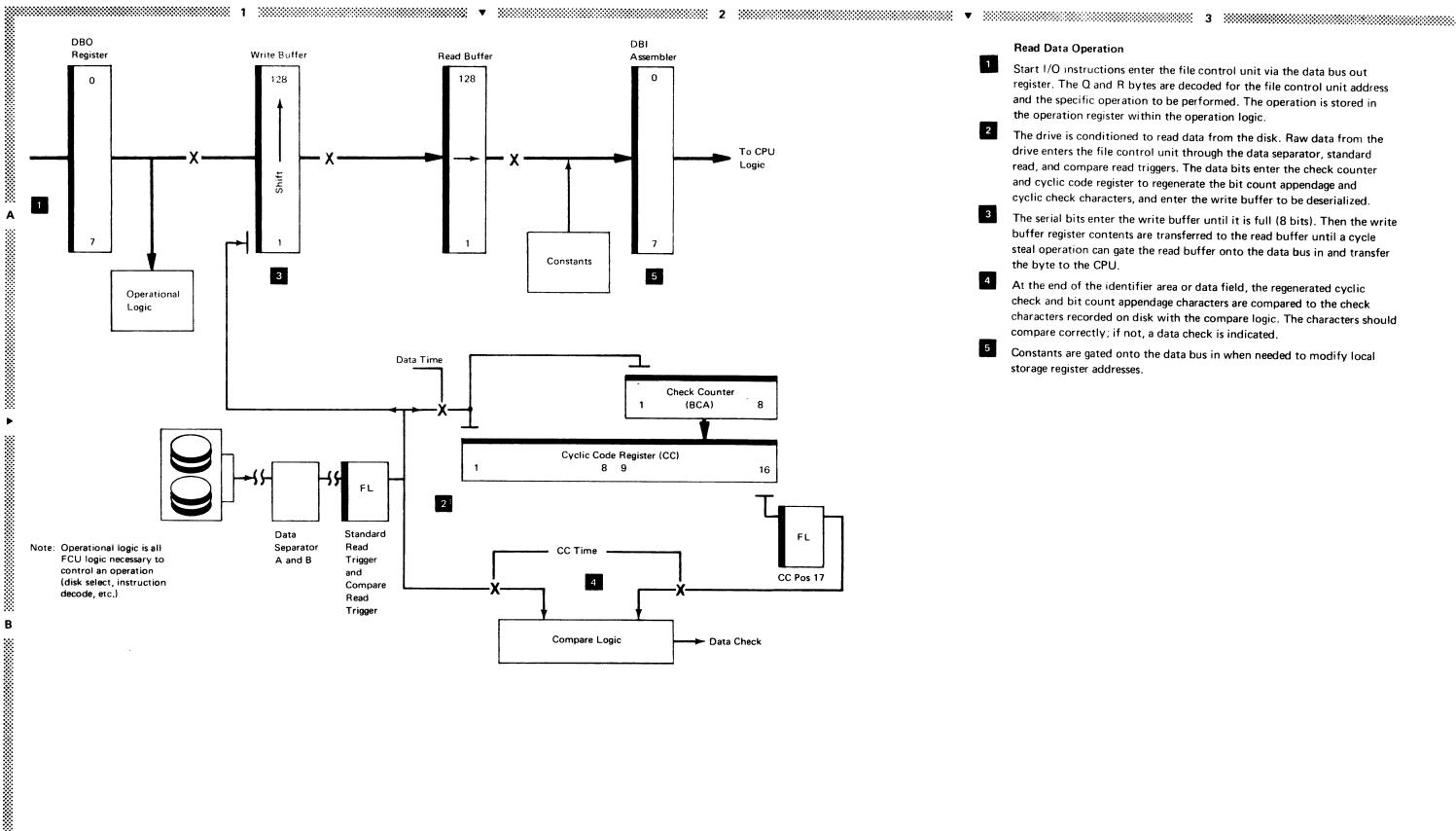
Start I/O instructions enter the file control unit via the data bus out register. The Q and R bytes are decoded for the file control unit address and the specific operation to be performed. The operation is stored in the operation register within the operation logic.
