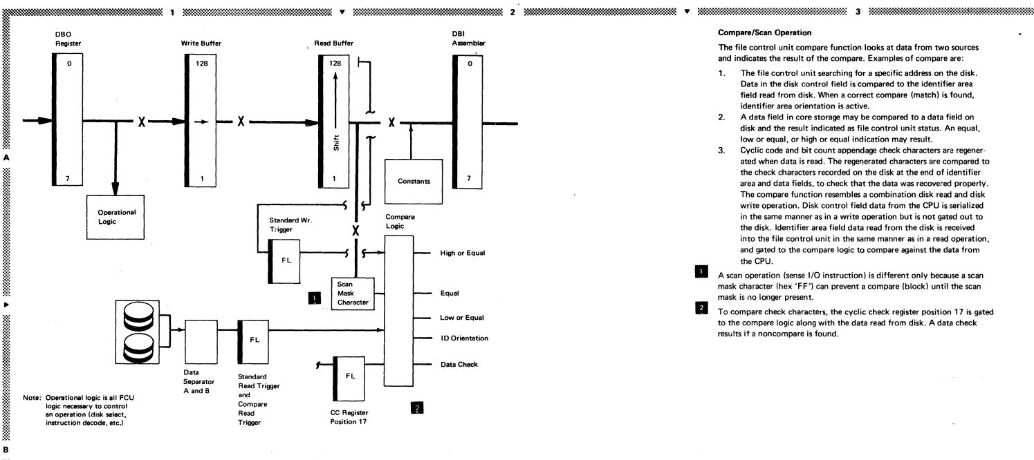
The file control unit compare function looks at data from two sources and indicates the result of the compare. Examples of compare are:
