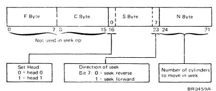
The N byte specifies the number of cylinders the access mechanism will move on the seek. Bit 23 of the S byte specifies the direction of movement. Forward (bit 23 = 1) is from cylinder 0 to 202.
