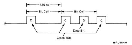
Separated data pulses are processed by the file control unit standard-read and compare-read triggers. As a result, the compare-read data signal is one bit cell in length and one bit cell later in relation to when the data bit was read.
