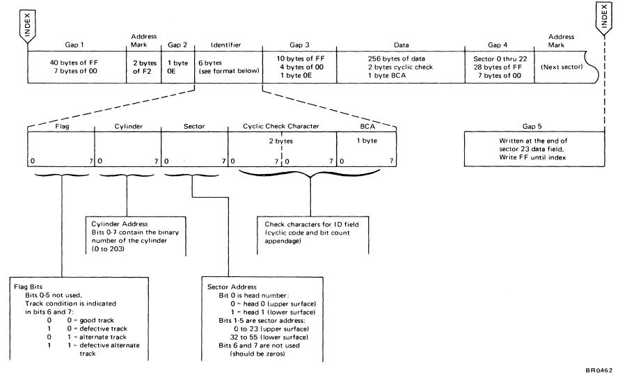
G3 A gap area between the identifier and the data area of a sector. G3 contains 15 bytes: ten bytes of FF, followed by four bytes of zeros, followed by one sync character (hexadecimal OE).
