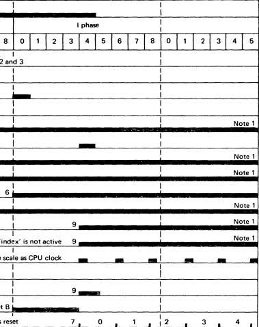
Note 1: These lines are active until 'end operation reset'. Normally this will occur when an operation is complete. An FCU error may cause 'end op reset' to be active at any time
