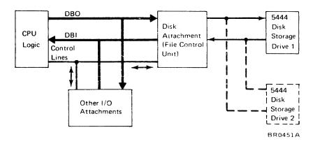
The file control unit contains logic circuits to:
