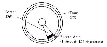
Track 00, the index track label, is described later in this appendix. A program used by a 3741 directly attached to a System/3 requires fixed length records (any specified length between 1 and 128 characters).
