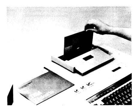
Figure 2. Inserting an IBM Diskette
