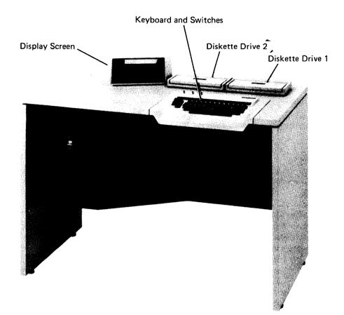
Figure 1. IBM 3741 Data Station or Programmable Work Station
