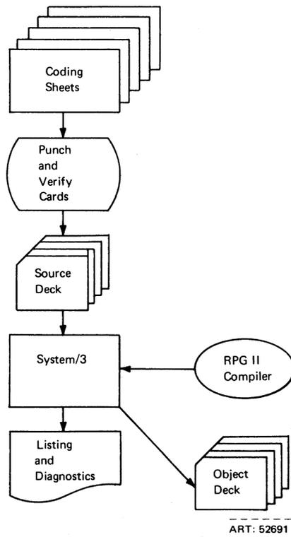
Figure 3-2. Steps in Producing an Object Program
