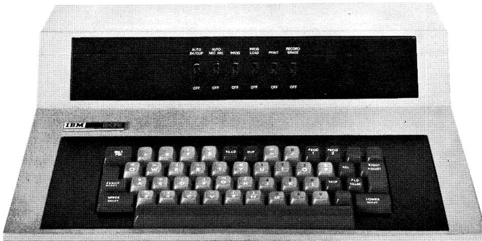
Figure 6-2. IBM 5475 Data Entry Keyboard
