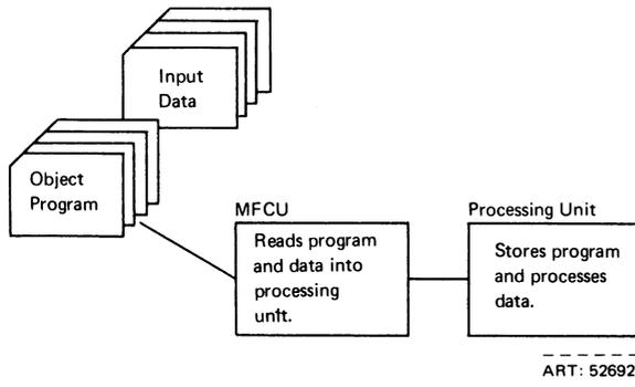
Figure 3-3. Loading a Program and Input Data
