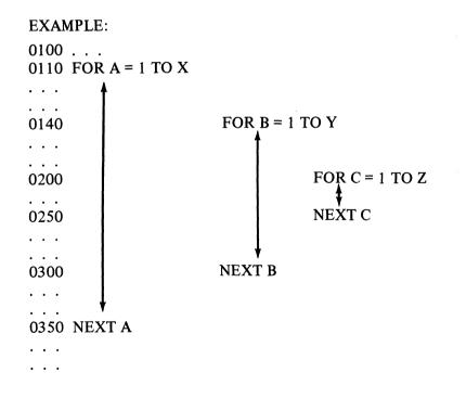
Here the FOR B. . . NEXT B loop is nested in the FOR A. . . NEXT A loop; and the FOR C. . .NEXT C loop is nested in both the FOR B. . .NEXT B loop and the FOR A. . . NEXT A loop. In nested loops, another loop is entered before the preceding loop is concluded.
