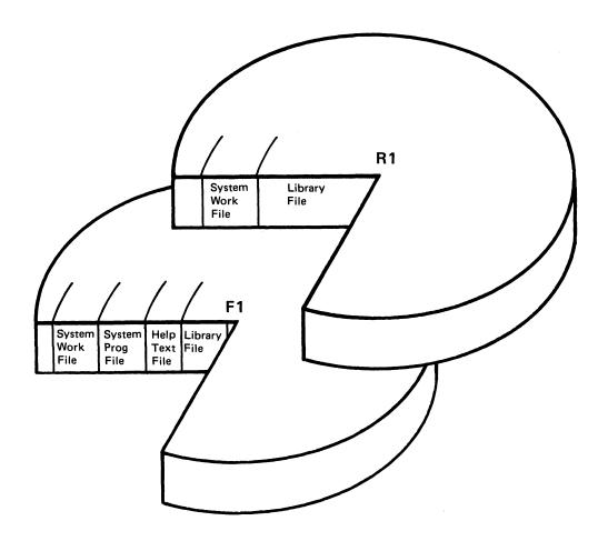
The figure above shows these areas organized on two disks, F1 and R1. The System Program Area, the HELP Text File, a File Library Area, and a System Work Area are on F1. Additional File Library space and a System Work Area are located on R1. This is not the only possible arrangement, but there are two rules that must be observed in organizing disks:
