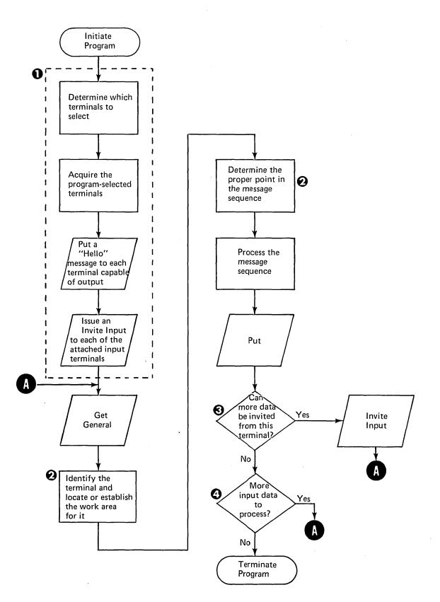
Figure 10. Program that Communicates with a Single Requester Terminal and Program-Selected Terminals
