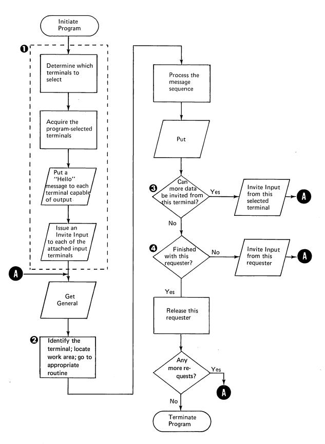
Figure 12. Program that Communicates with Multiple Requester Terminals and Program-Selected Terminals
