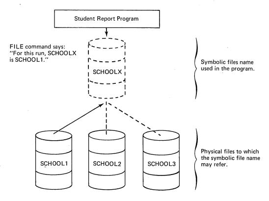
Figure 14. Illustration of FILE Command
