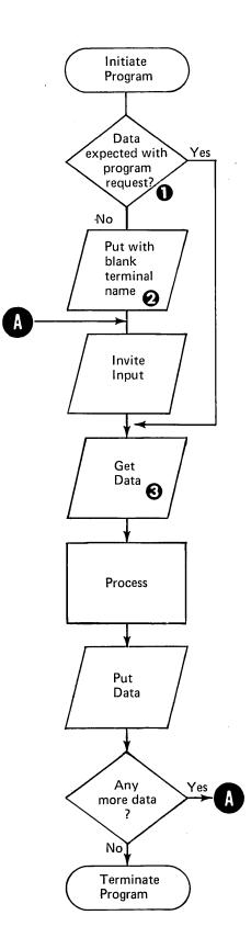
Figure 9. Program that Communicates with a Single Requester Terminal
