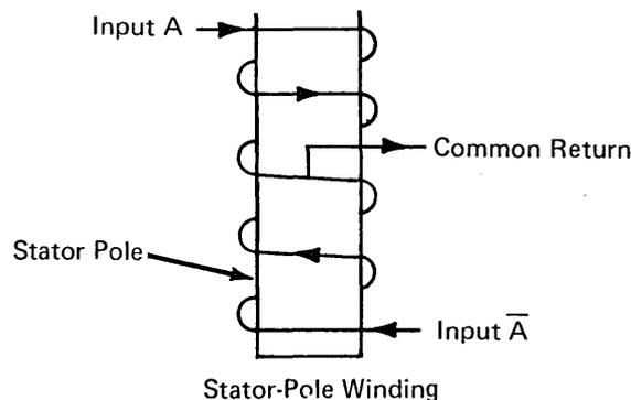
*Note:* Current flows only in one-half of the winding at a time. Polarity of the stator pole is determined by which half of the winding has current.
