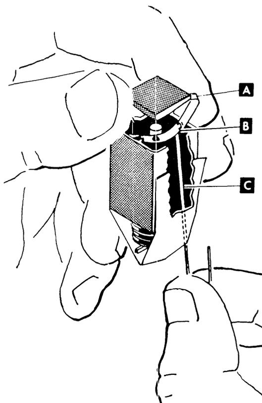
10. Check the key stem ears for taper in the center slot and form the ears if necessary.
