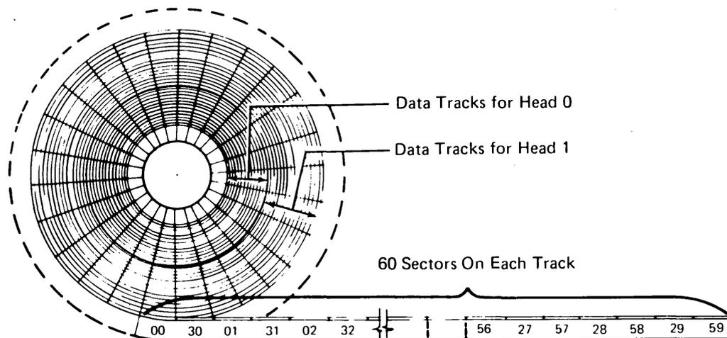
VFO sync is 12 bytes of hex FF used to synchronize the read clock with data bits from the disk. When the 12 VFO sync bytes are being written on the disk, the attachment forces 8 bytes of hex FF, and then cycle steals the other 4 bytes from a 10 byte field of hex FFs in storage.
