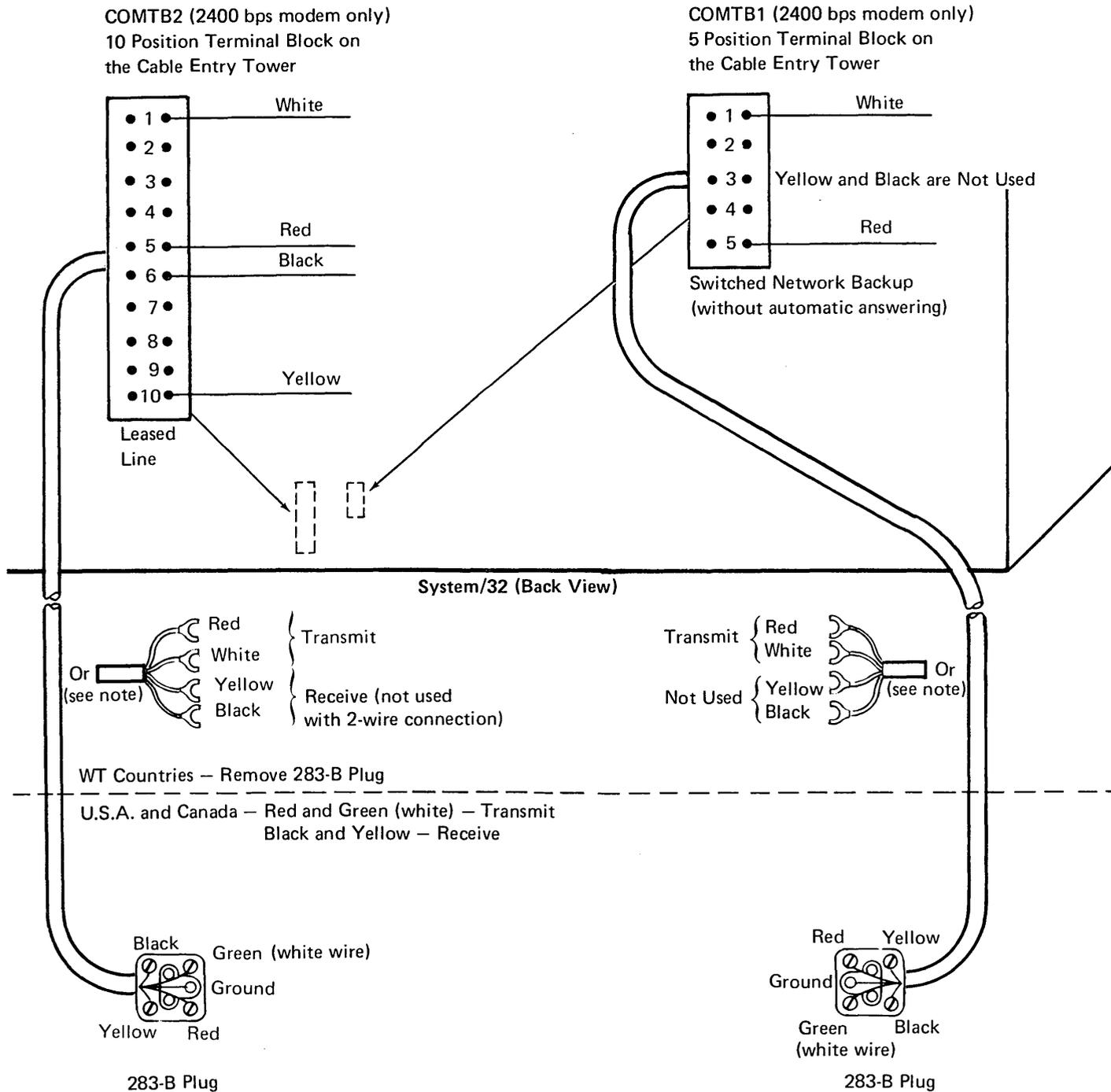
*Note:* There is only one cable to the common carrier from each terminal block. The 283-B plug is used in the U.S.A. and Canada; it is removed for WT countries.
