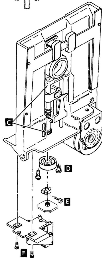
6. Remove stepper motor **F** and leadscrew wheel **E**.
