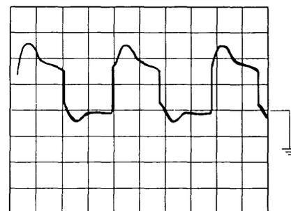
Note the loss of amplitude in the negative portion of the waveshape.
