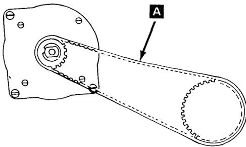
7. The ribbon drive belt should track on the pulley so that there is at least one sixteenth of an inch between the belt and the motor top plate. To increase the clearance, add shims under the rear edge of the ribbon mounting bar assembly.
