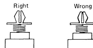
11. Install the key module in the keyboard (6.3.2).
