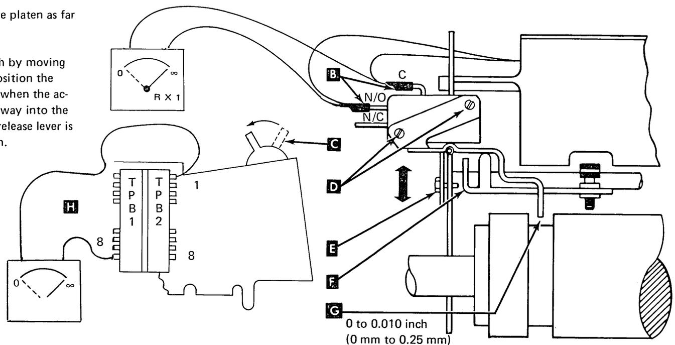
8. Tighten the switch assembly mounting screw **E**.
