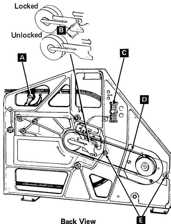
6. Tighten the screws on the spindle locking arm.
