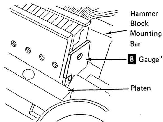
11. Lift the gauge about 0.060 inch (1.52 mm) above the bottom lip of the platen **F**, and set the forms thickness control on 1 to clamp the gauge.
