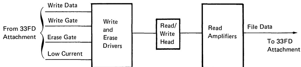
Low current line is under microprogram control and is active from logical track 42 through 76. When this line is active, the current through the write head is reduced.
