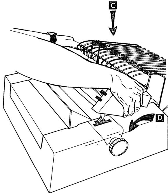
*Note:* When reinstalling, make sure that the gears **E** mesh properly, the platen knobs turn, and the forms tractors rotate.
