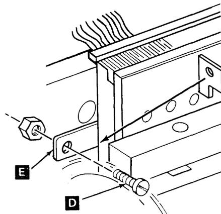
13. Remove screw **D** from the left end of the hammer block mounting bar, and slide the hammer position scale **E** to the right.
