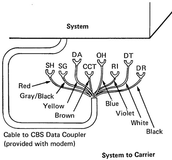
Refer to paragraph 10.3.1.1 in this section for the WT PSN cable connections.
