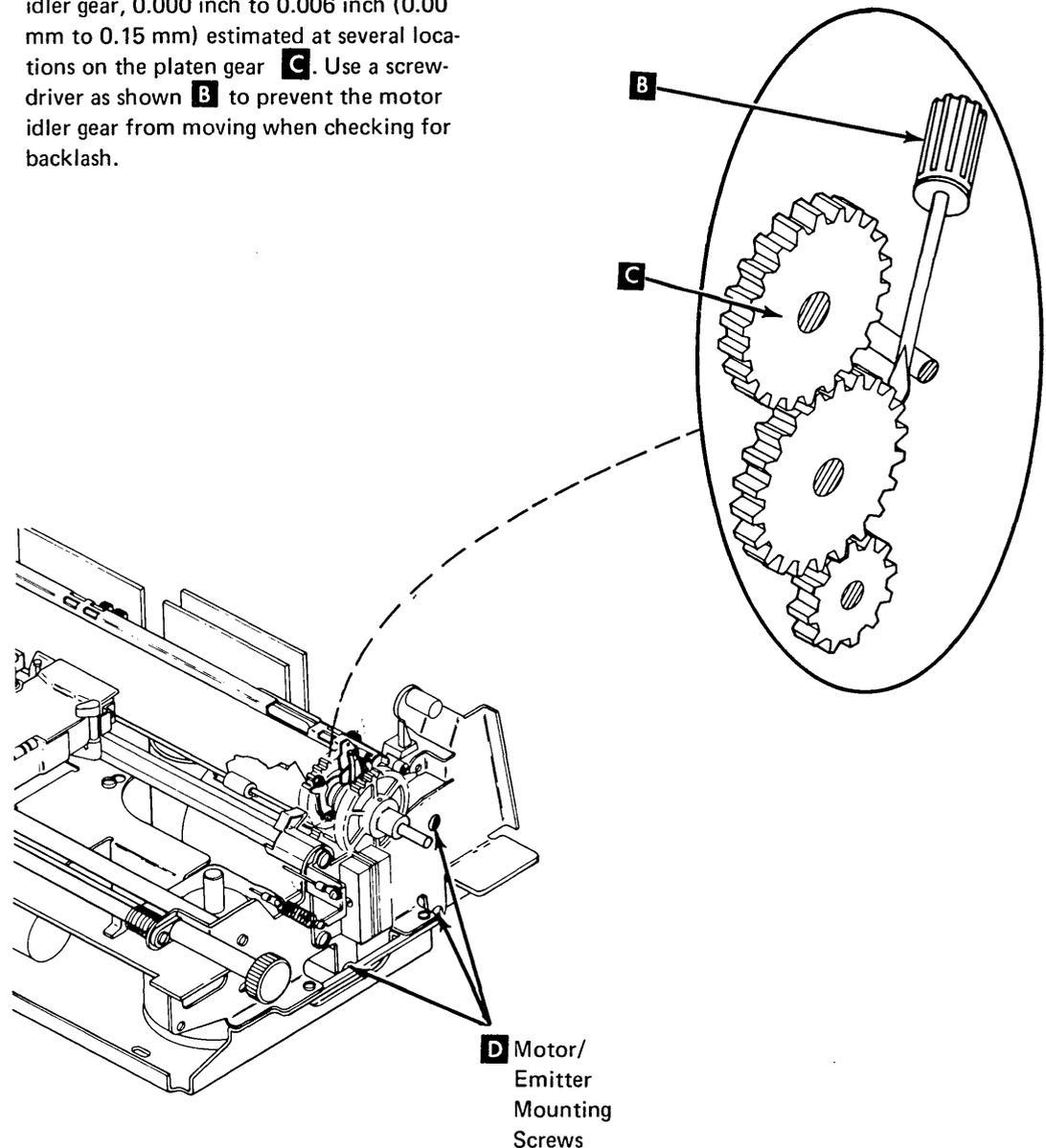
5. Tighten the mounting screws and check for binds and minimum backlash at several locations on the platen gear.
