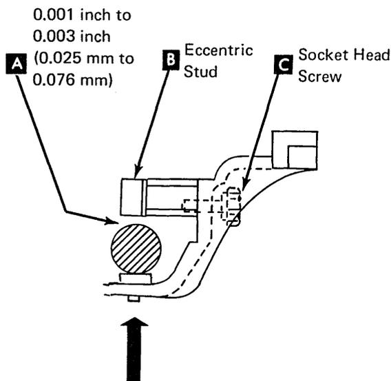
3. Adjust the carrier main shaft (hexagonal) as follows:
