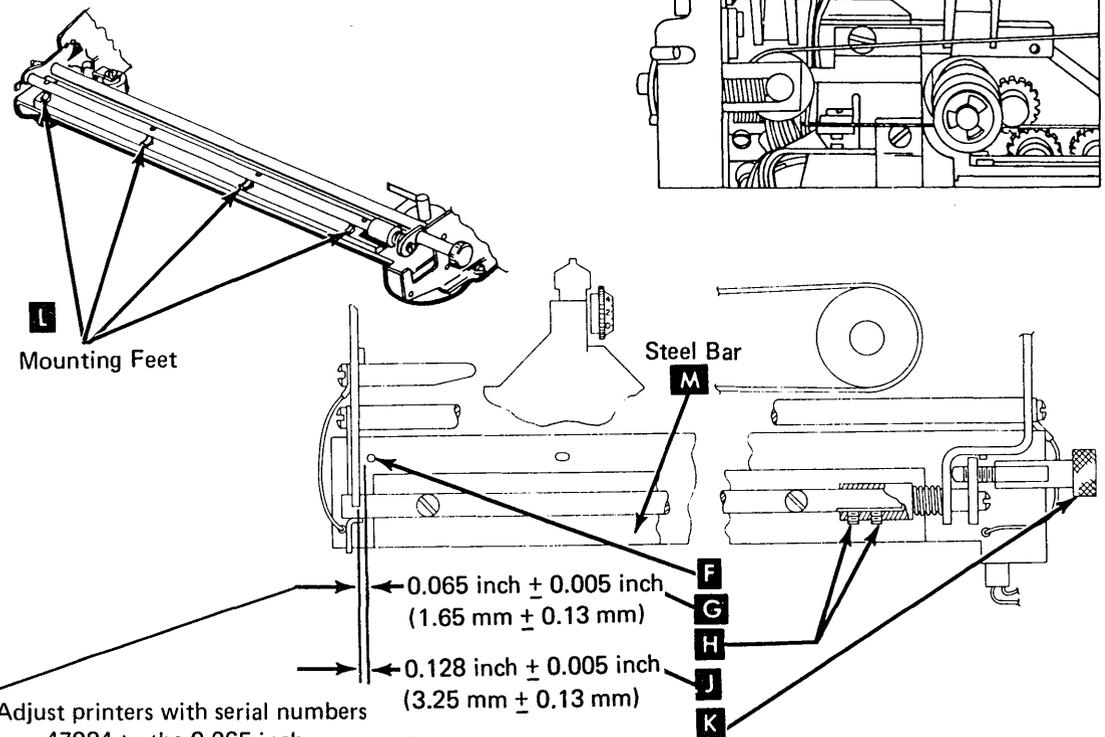
*Note:* Adjust printers with serial numbers below xxxx47984 to the 0.065 inch clearance. Adjust printers with serial number xxxx47984 or higher to 0.097 inch  $\pm$  0.005 inch (24.64 mm  $\pm$  0.013 mm).
