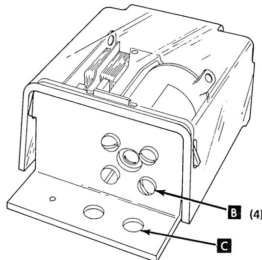
Relay is mounted on outside of right side frame.
