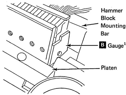
10. Lift the gauge about 0.060 inch (1.52 mm) from the edge of the forms guide, and set the forms thickness control on 1 to clamp the gauge.
