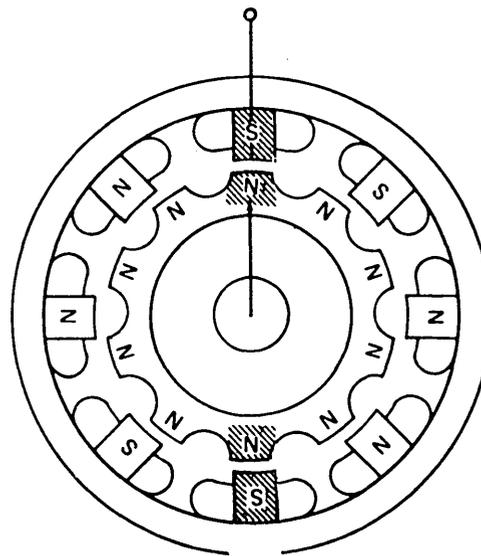
If we physically rotate the stator (in either direction), the rotor maintains its detented position and follows the stator as shown. (Both the stator poles and the rotor rotated clockwise 45 degrees.)
