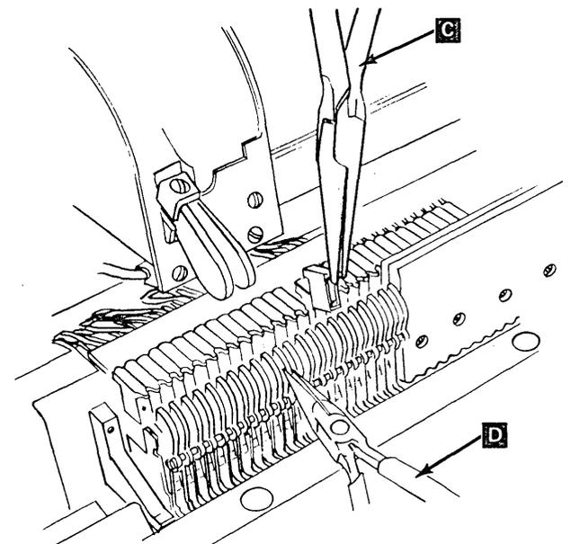
**Odd (Lower) Coil Removal**
