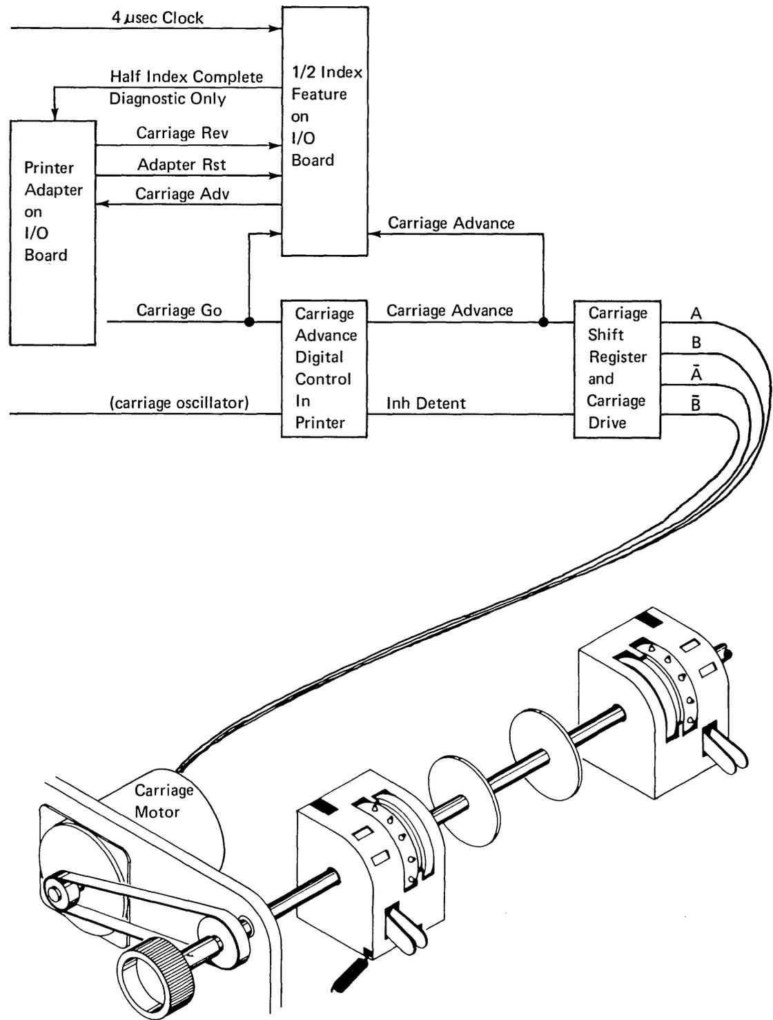
A half line space operation is initiated by setting the carriage reverse bit (bit 4) in a control load command (IOCL) with a modifier of A. Half index mode is reset by bit 5 of the command and the half index feature card is reset by bit 5 of the command, dropping carriage go, or resetting the printer attachment.
