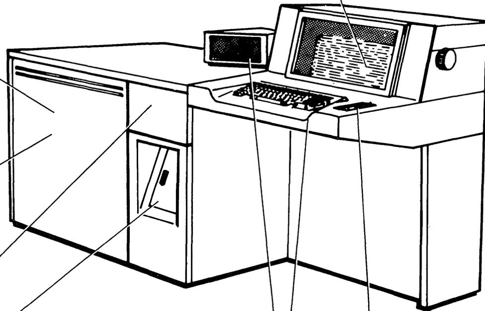
The **display unit** is used for prompting, job output, and error messages. Up to six lines of 40 characters per line can be displayed at one time.
