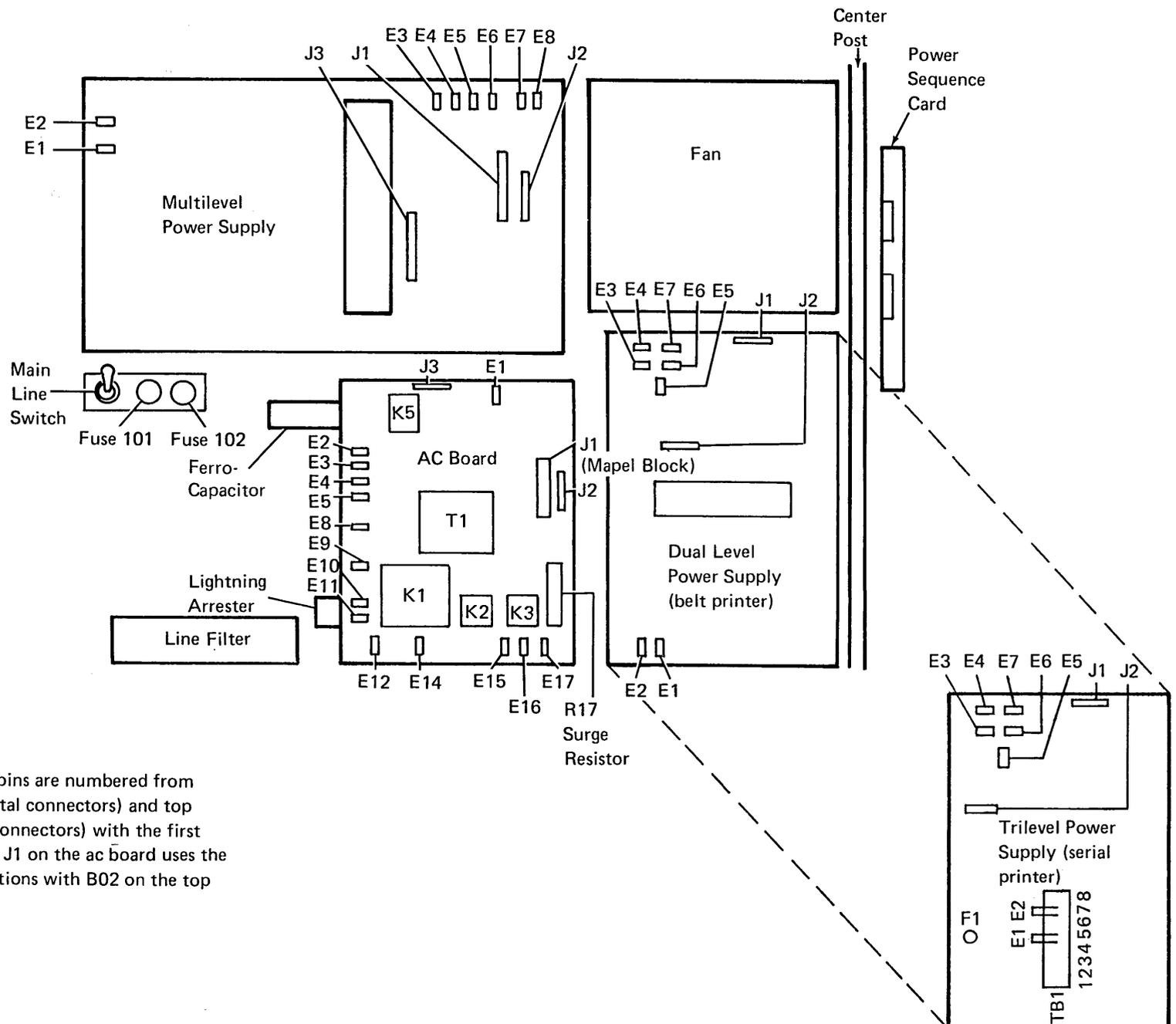
*Note:* The J socket pins are numbered from left to right (horizontal connectors) and top to bottom (vertical connectors) with the first pin being number 1. J1 on the ac board uses the conventional designations with B02 on the top left.
