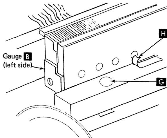
2. Close the print unit and set the forms thickness control on 3.
