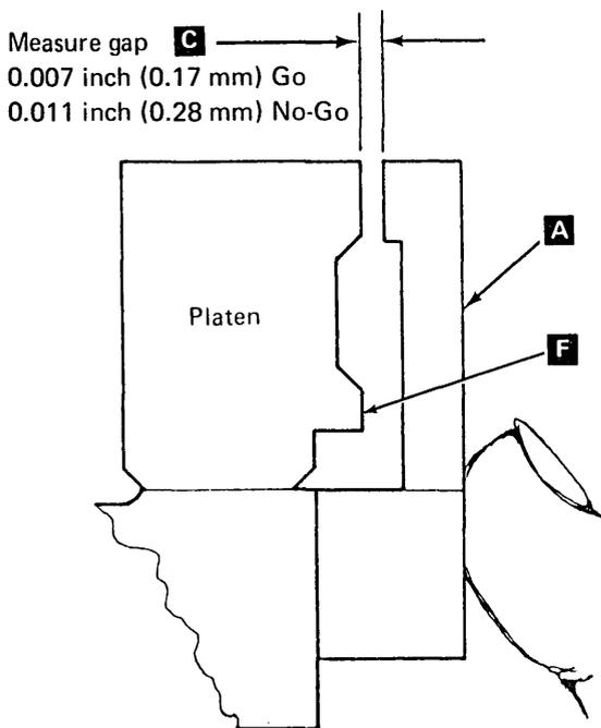
6. Do the platen gap adjustments. (Omit the remaining steps in this service check.)
