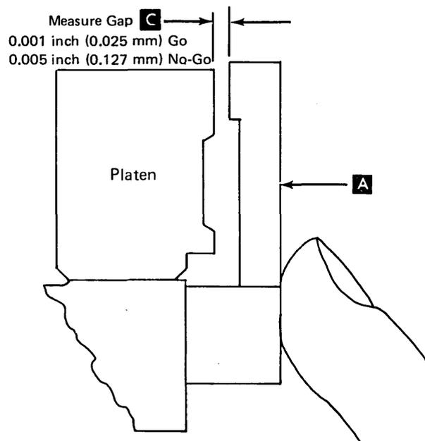
5. Do the platen gap adjustments. (Omit the remaining steps in this service check.)
