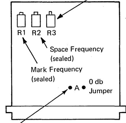
Jumper A is required for full adjustment range. Remove the jumper for networks that restrict the transmit level attenuation to a level of less than -2 db (WT).
