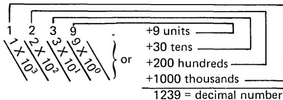
As shown above, the decimal numbering system allows counting to ten in each position—from units to tens to hundreds to thousands, etc. The binary system allows counting to two in each position. Register displays are binary: a bit light on is a 1; a bit light off is a 0.
