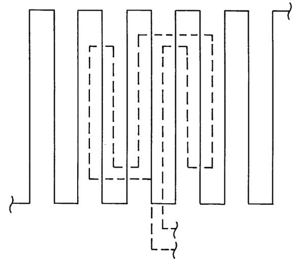
This illustrates the null position of the print emitter land pattern. The land pattern of the print emitter pickup is shown in phantom.
