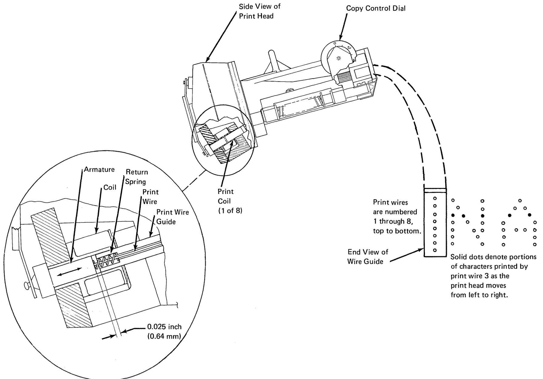
As required by the character pattern, each wire can strike the ribbon up to four times per character (for example, print wire 5 when printing the character A).
