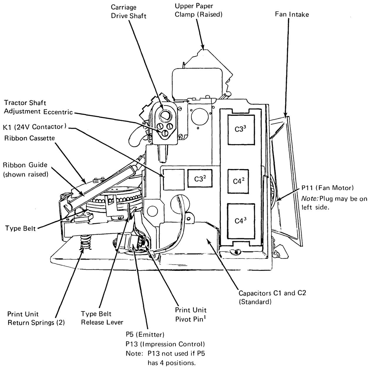
*Note:* C1 through C4 are located under the logic gate on some early machines with 3  $\mu$ f capacitors C3 and C4. See 4.3.5.
