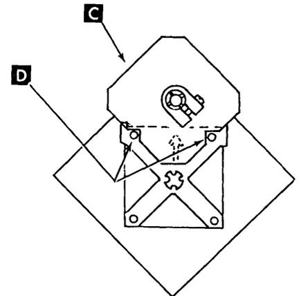
8. Slide the stepper motor wheel toward the leadscrew until pins contact notches. No clearance is allowed.
