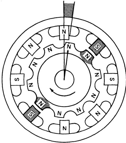
The stepper motor is advanced by pulses provided by two triggers in the adapter.
