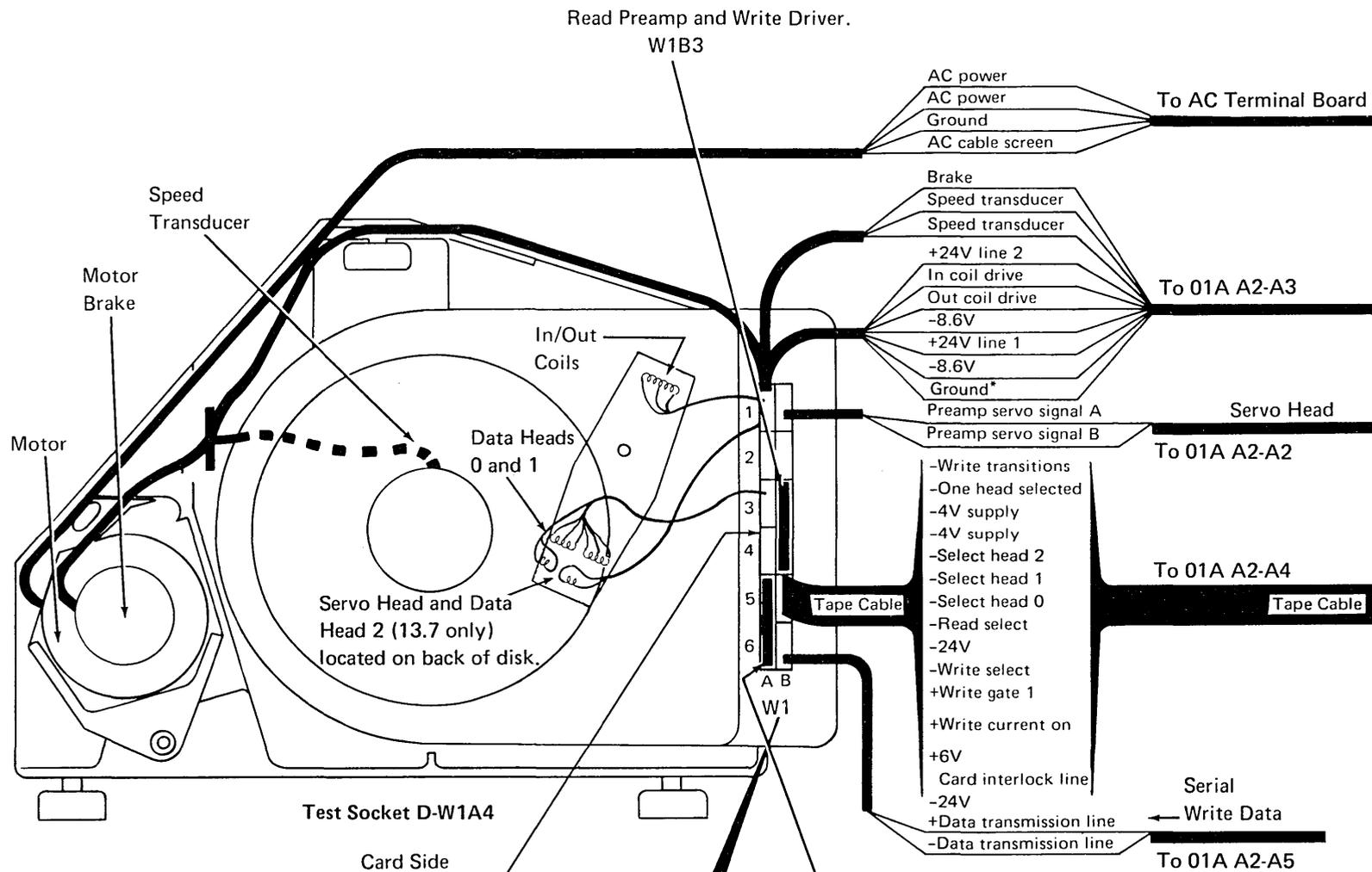
Inaccessible pins on other cards are connected to pins on D-W1A4, to allow testing (see logic page GV270).
