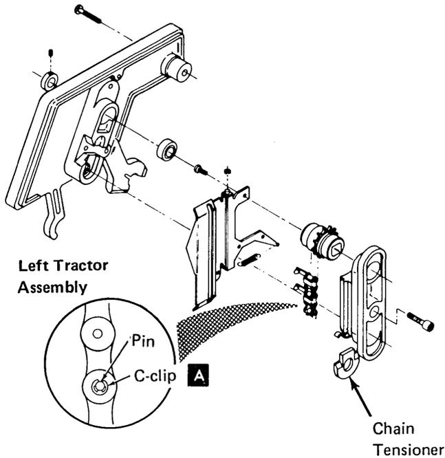
5. Machines equipped with an adjustable left tractor should follow this procedure. With the left tractor in the leftmost position, adjust the collar **E** to allow 0.200 inch  $\pm$  0.010 inch (5.08 mm  $\pm$  0.25 mm) movement of the tractor.
