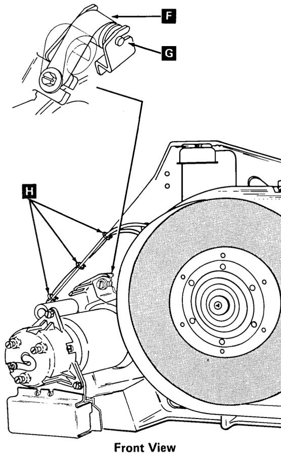
13. Tighten the screws on the spindle locking arm.
