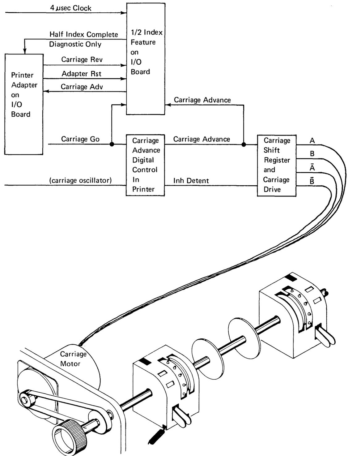
A half line space operation is initiated by setting the carriage reverse bit (bit 4) in a control load command (IOCL) with a modifier of A. Half index mode is reset by bit 5 of the command and the half index feature card is reset by bit 5 of the command, dropping carriage go, or resetting the printer attachment.
