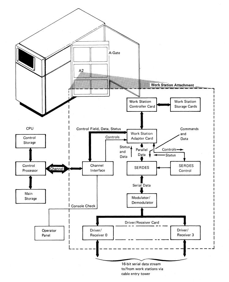
All work stations communicate with the attachment through a 16-bit serial data stream via twinaxial cables. For a description of the data stream, see Serial Interface to Work Stations later in this section.
