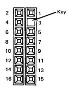
Connector C-B1J7 16-Position Cable Connector Pin Side P/N 2731844
