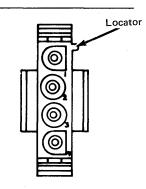
Connectors J4, J9, and C-B1J2 6-Position **Board Connector** Pin Side P/N 1295112
