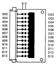
Connector J11, C-B1J3, C-B1J4, and C-B1J5 24-Position Cable Connector Probe Side P/N 5800634
