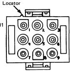
Connector J1 12-Position Cable Connector Pin Side P/N 1847535
