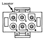
Connectors J10, J20, and C-B1J1 9-Position **Board Connector** Pin Side P/N 1473911
