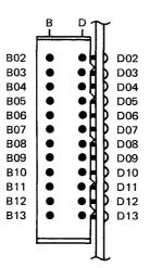
Connector J6 24-Position Board Connector Pin Side P/N 818869
