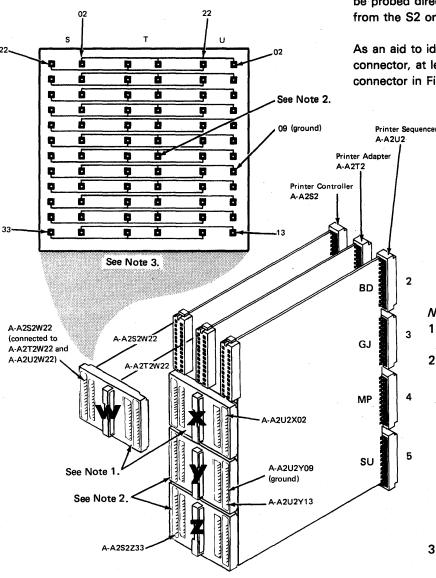
Figure 08-2. Printer Attachment Top Card Connectors
