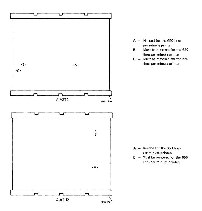
Figure 08-4. Printer Adapter Cards Jumpering
