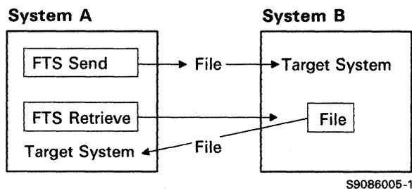
Figure 12-1. Example of File Transfer Subroutines
