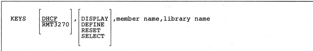
Figure K-1. KEYS Procedure Syntax Diagram
