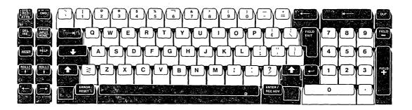
Figure 3-24. 5251 Typewriterlike Keyboard
