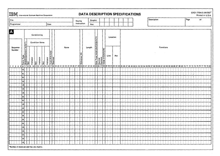
The data description specifications form is used for coding the data description specifications for externally described data files:
