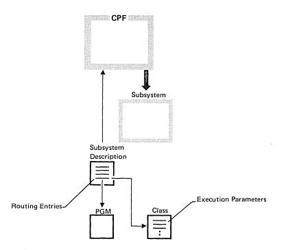
The same class can be specified for any number of routing entries. The parameters that are specified in a class include:
