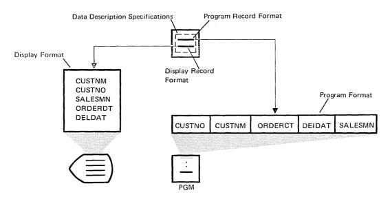
If program described data files are used for display devices, the record formats and display formatting must be specified in the application program that processes the file. The following discussion about display device support is limited to the use of externally described data files.
