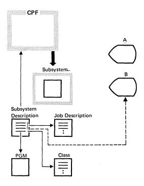
In this example, one of the work entries in the subsystem description specifies work station B as a source of work. The work entry also specifies a job description. The routing entry specifies the program and class to be used when a routing step (within a job) is started.
