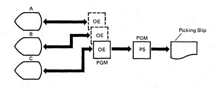
To prevent this delay, the program that produces picking slips processes entries by processing messages from a message queue, as shown in the next drawing. The order entry program sends a message to that queue for each order and then continues processing.
