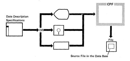
2. A command is entered to create the file. This command identifies the source file that contains the data description specifications for the file:
