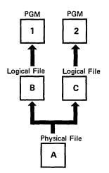
Data in a physical file can be used by any number of logical files. Each file can impose its own characteristics, such as field length and type, on the data. However, the data is always stored in the system according to the characteristics and organization specified by the physical file. When a data record is accessed through a logical file, the data is transformed to meet the requirements of the logical file. This data transformation is not apparent to the program using the file.
