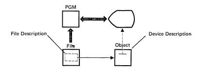
Device files created by CPF are program described data files. That is, the formats of the records in these files must be described in the programs that use them. Additional device files can be created to meet any special processing requirements.
