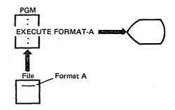
3. Using record format A, CPF displays the record on the screen. The two constant fields (NAME: and ENTER NO.) are specified in the record format. The variable from the application program is displayed following NAME:. The input field following ENTER NO. is to be filled in by the work station user.
