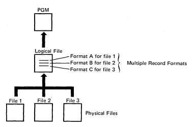
The records processed from a logical file can vary in length because of the different record formats used. The access path for the logical file determines the order in which the records are processed from the physical files. This makes different record formats from different physical files available through one logical file.
