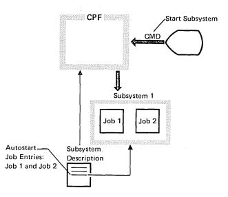
Examples of autostart jobs are jobs that perform initialization functions for applications or jobs that are used as service jobs by other jobs that execute in the subsystem.
