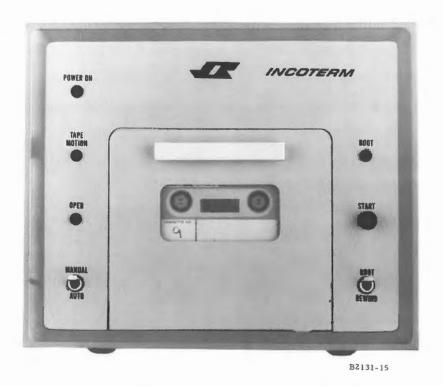
Figure 2-1. SPD-T Operator Controls And Indicators
