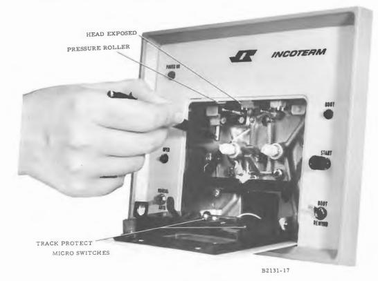
Figure 5-3. Tape Head Exposed
