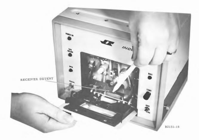
Figure 5-1. Releasing the Receiver Detent
