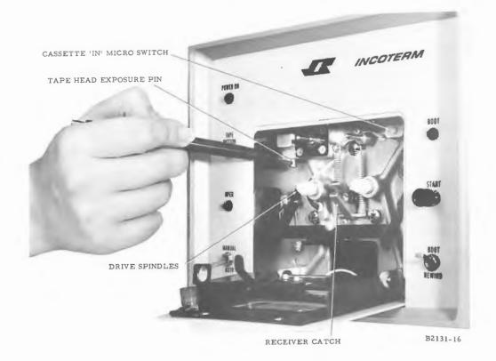
Figure 5-2. Method Used to Expose Parts for Cleaning
