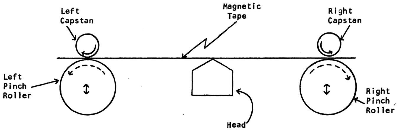
Figure 2-17. Typical Pinch Roller Drive
