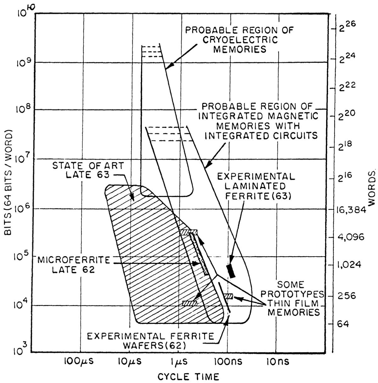
Figure 6-1. Storage Capacity and Cycle Time of Memories (After Rajchman)
