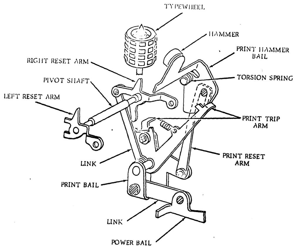
Figure 2-12. Drum Printer
