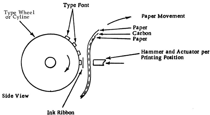
Figure 2-3. Rotating Drum Printer
