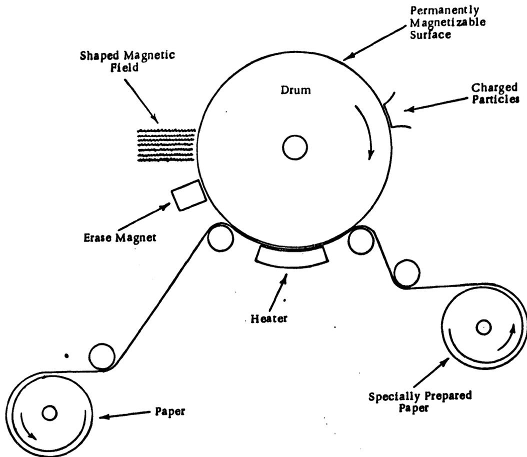
Figure 2-11. Magnetic Printer
