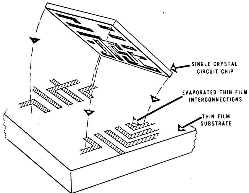
Figure 5-2. Flip-Chip Technique
