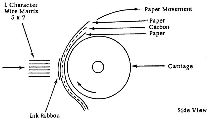
Figure 2-5. Matrix Printer
