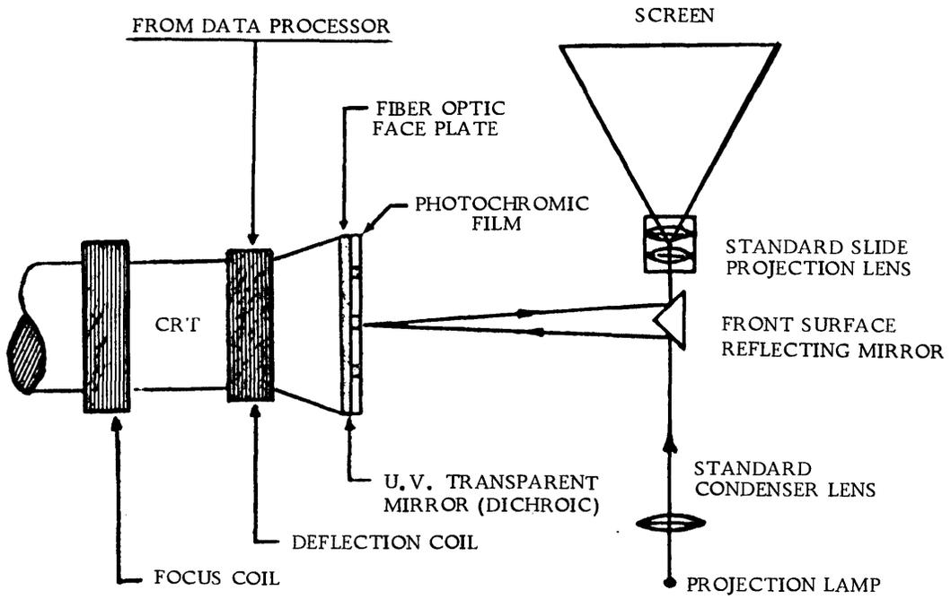
Figure 4-5. Photochromic/CRT Large Screen Display
