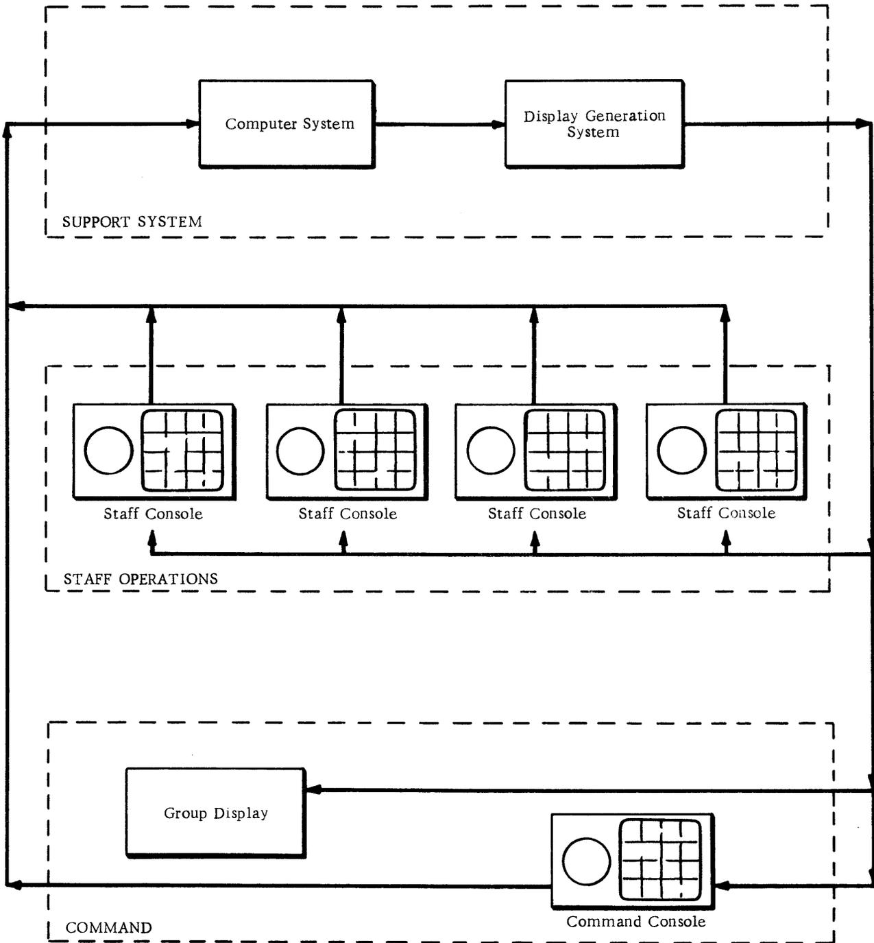
Figure 3-17. Command Node Configuration
