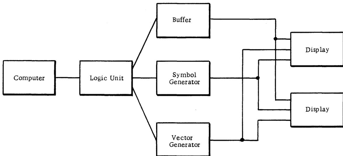
Figure 3-6. Multiple Console with Shared Components
