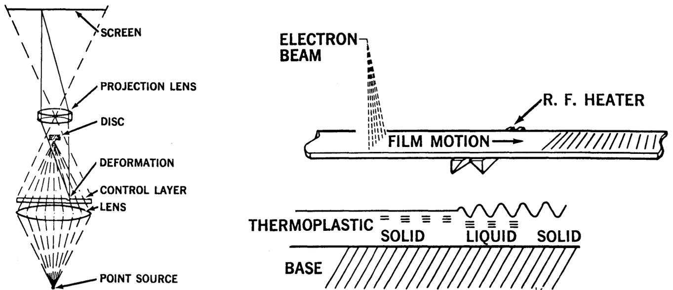
Figure 4-6. A Typical Light Valve Projection System
