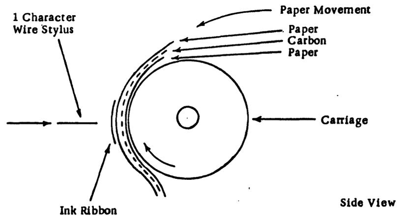
Figure 2-6. Stylus Printer
