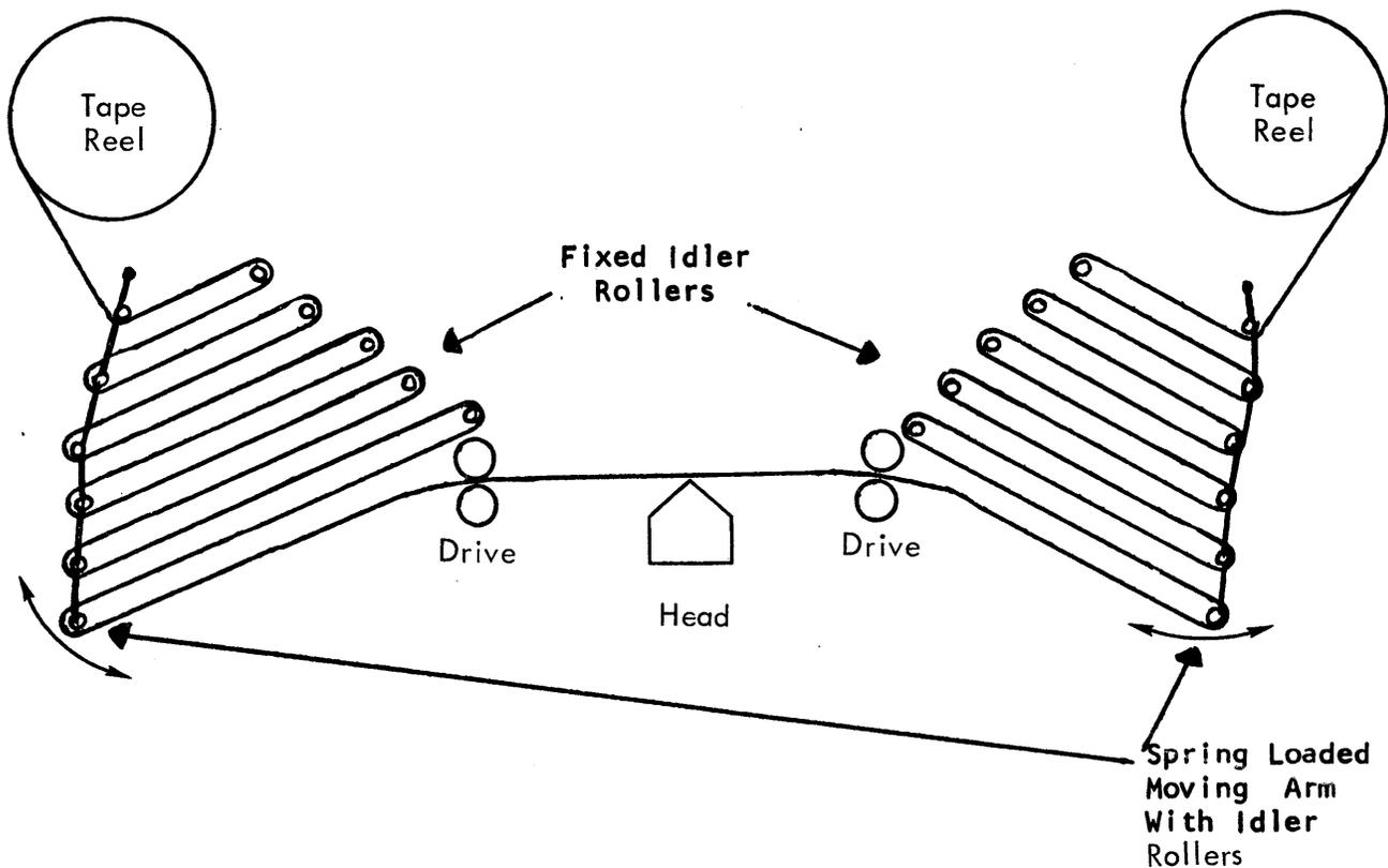
Figure 2-21. Typical Tension Arm or Mechanical Tape Buffering System
