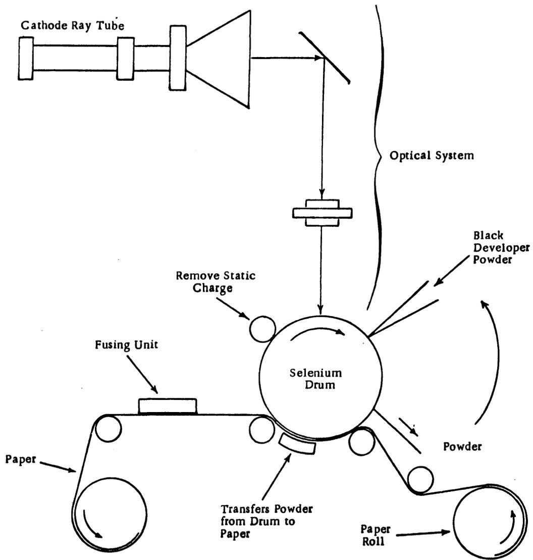
Figure 2-9. Electro-Optical Printer
