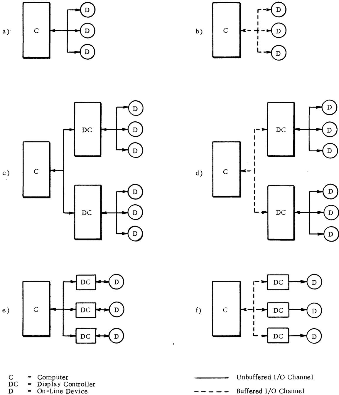
Figure 3-5. Computer/On-Line Device Configurations
