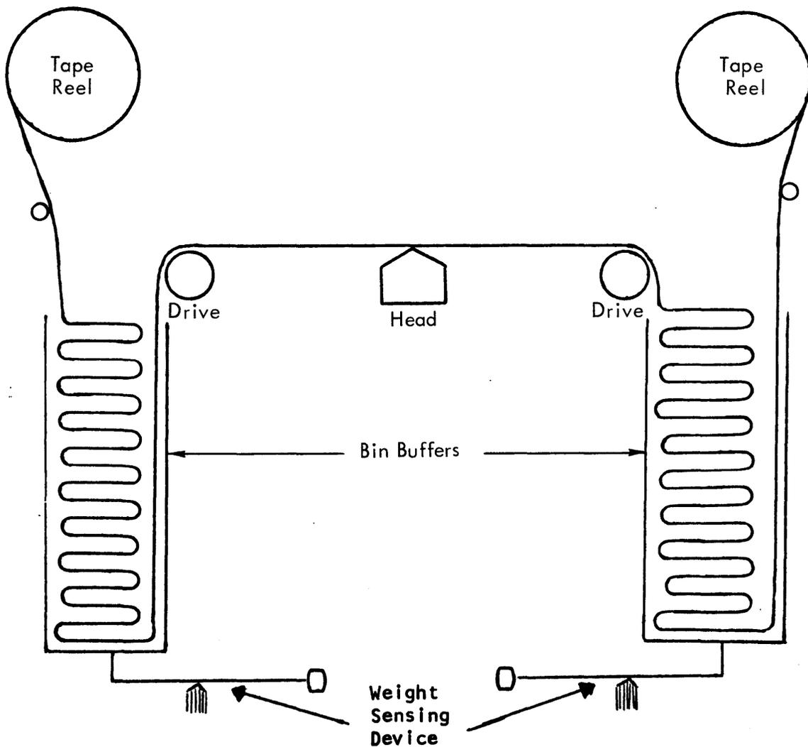
Figure 2-22. Typical Tape Bin, Tape Buffering System
