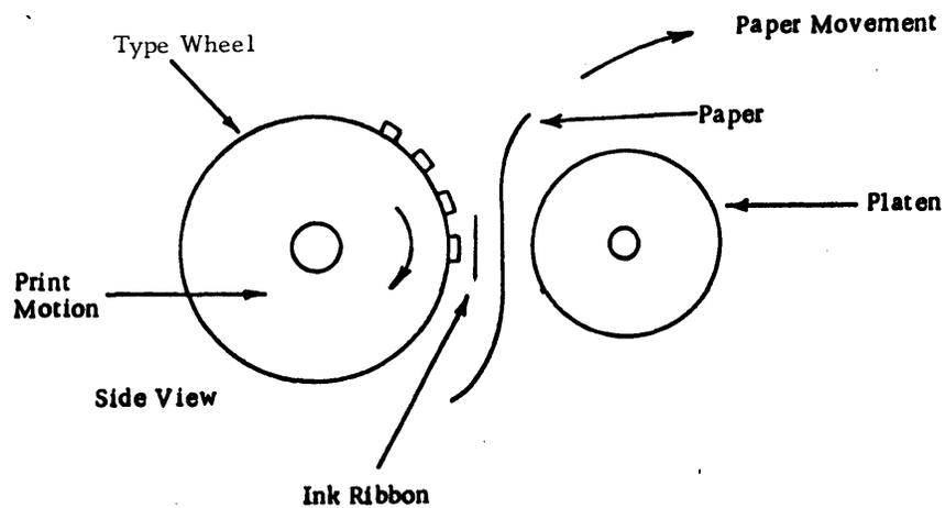
Figure 2-4. Impact Wheel Printer
