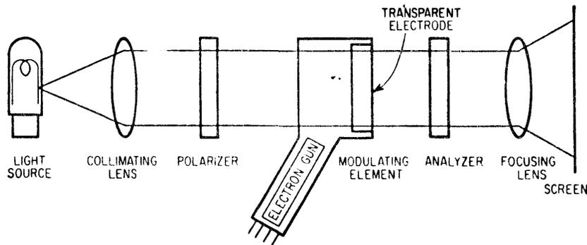
Light path through electro-optic light modulator. Modulating element is between polarizer and analyzer, and is scanned by electron gun at bottom.
