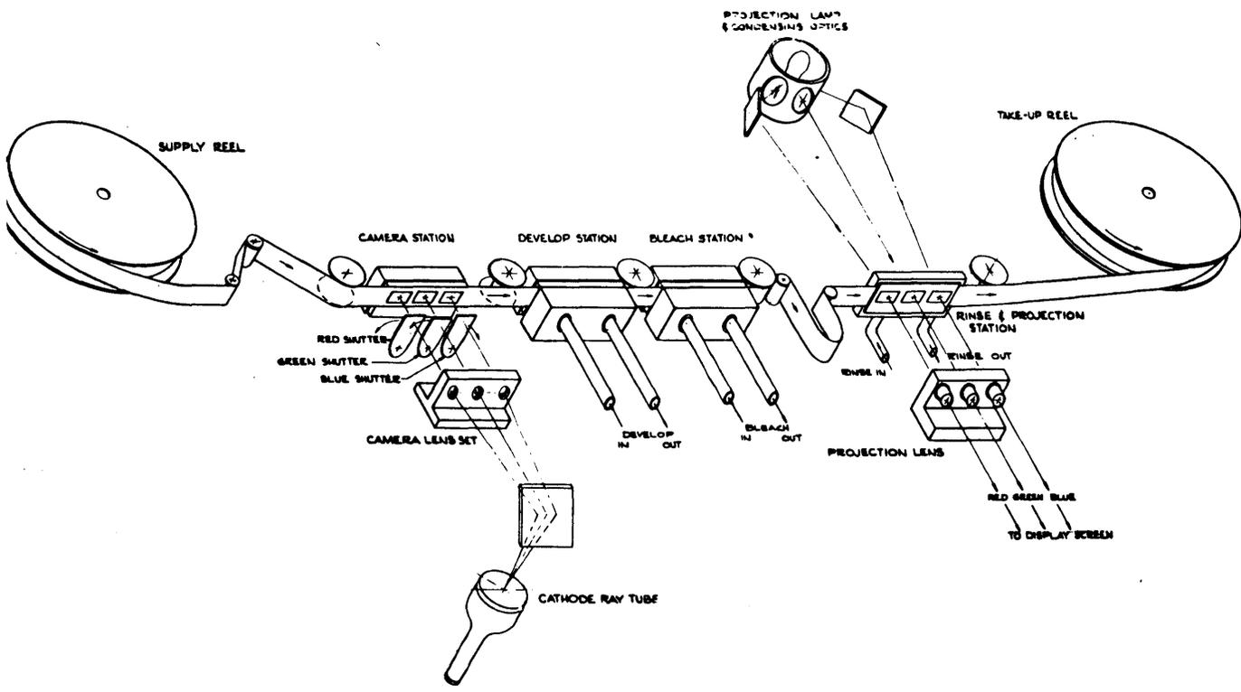
Figure 4-4. Multicolor Film Projection Display System
