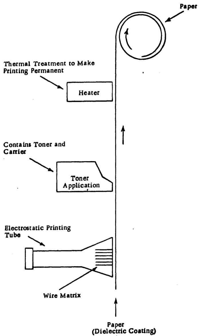
Figure 2-10. Electrographic Printer
