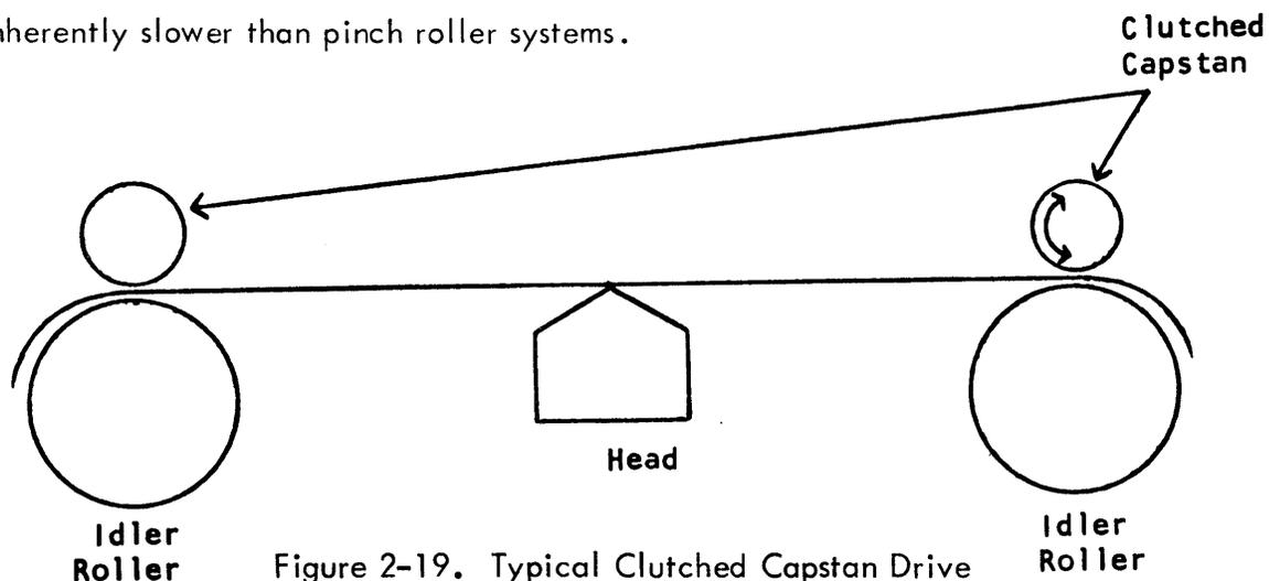
Figure 2-19. Typical Clutched Capstan Drive
