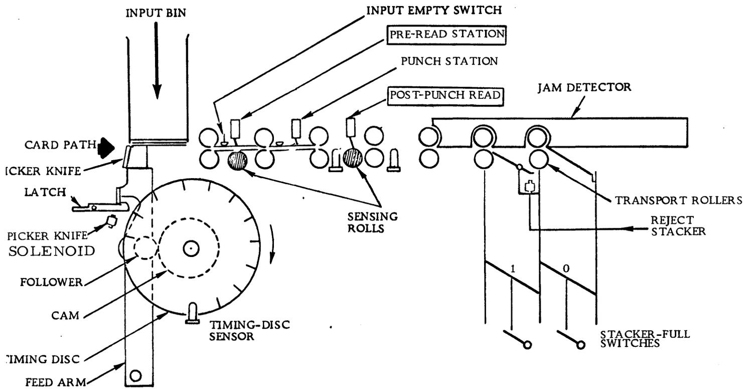
Figure 2-14. Card Punch Read Stations Before and After Punch Stations
