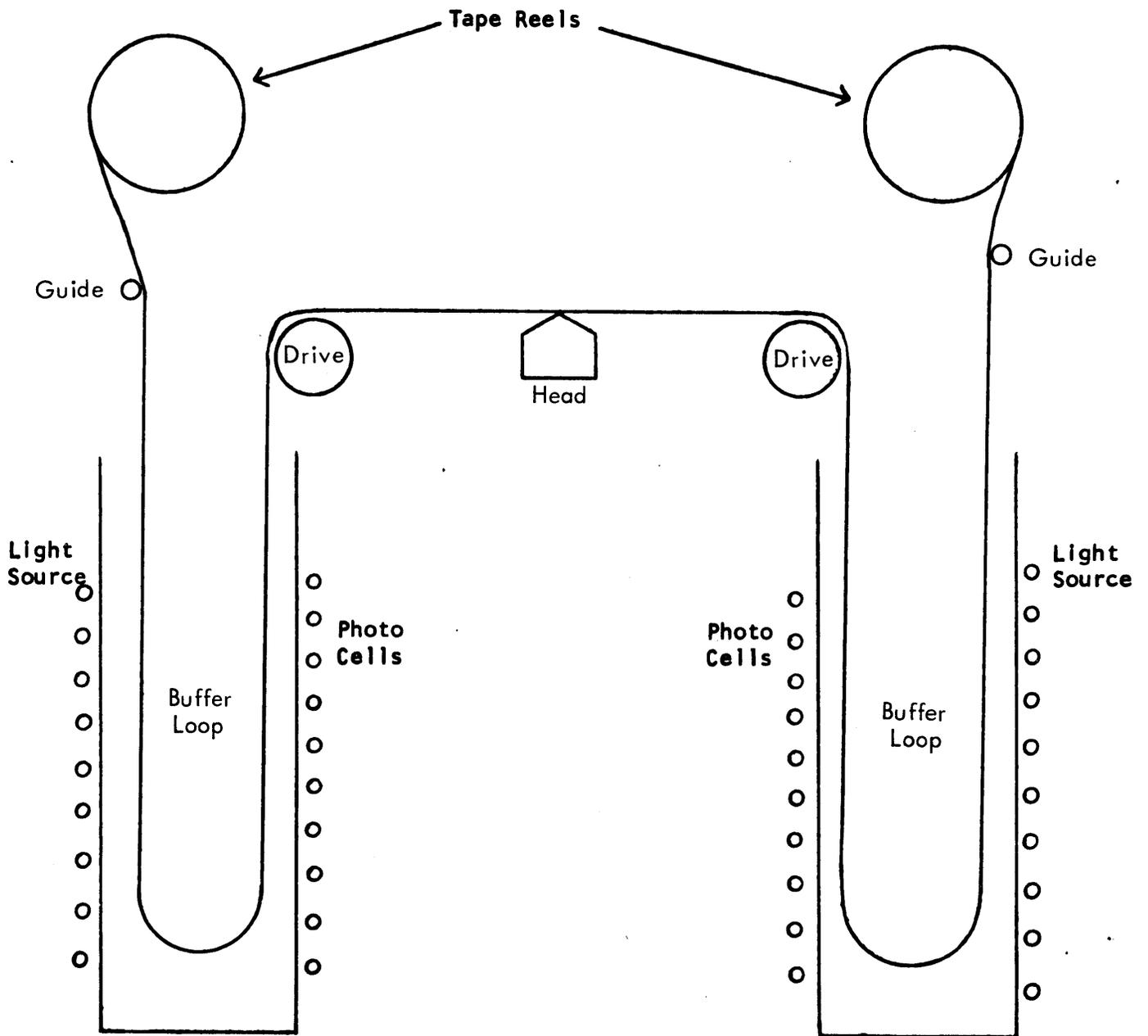
Figure 2-20. Typical Vacuum Column Tape Buffer Using Photo Electric Position Sensing
