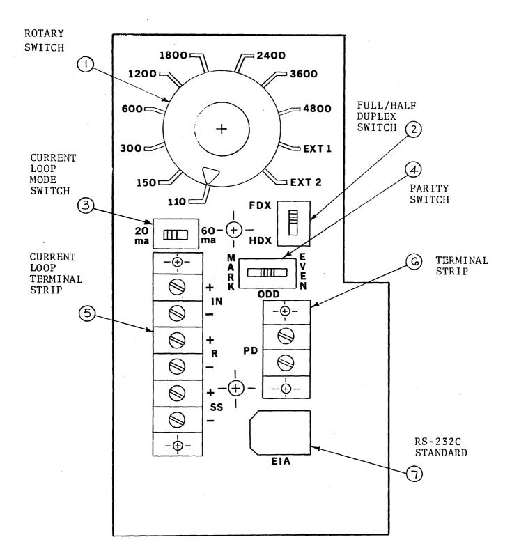
FIGURE 9: CONTROL PANEL OF ASYNCHRONOUS SERIAL INTERFACES I-103, I-104, and I-105
