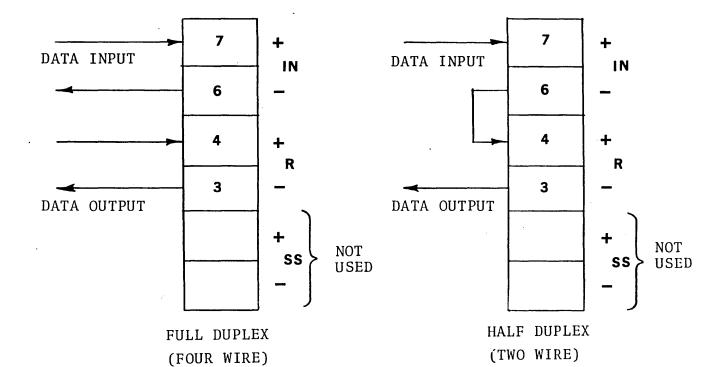
FIGURE 10: CURRENT LOOP CONNECTIONS
