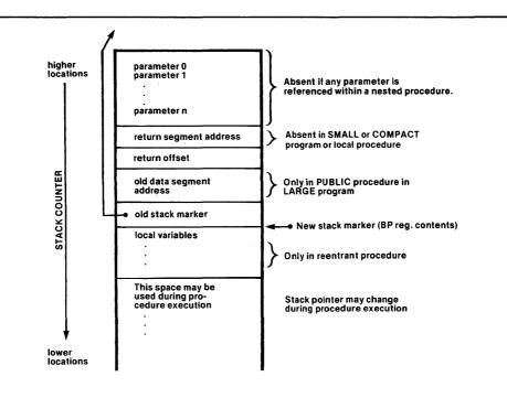
Figure H-2. Stack Layout During Execution of Non-Interrupt Procedure Body
