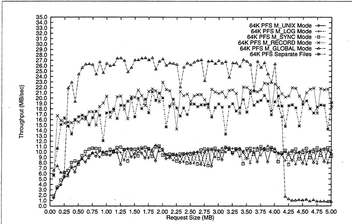
Figure 3-8. 64 KB PFS Read Performance (8 Compute Nodes, 8 I/O Nodes)
