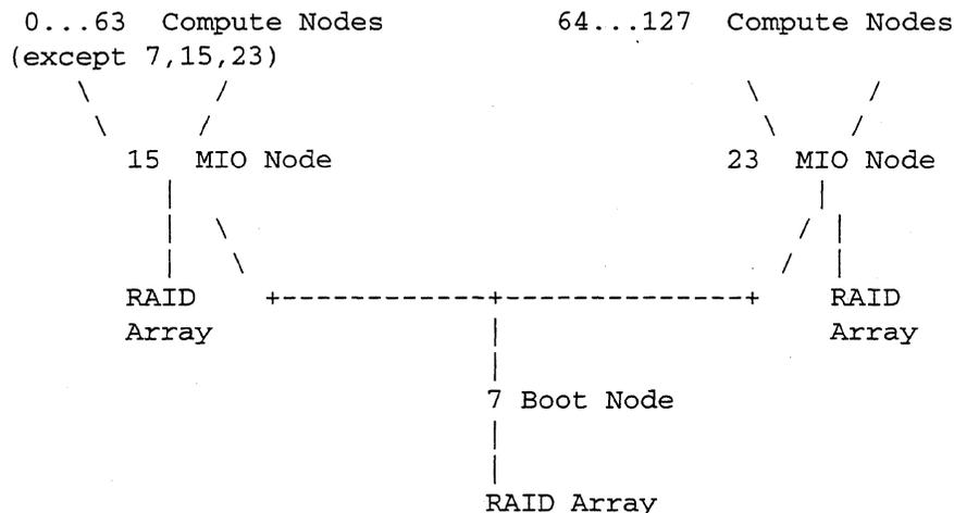
A three-level paging tree (as shown in the above diagram) where all the non-boot I/O nodes page to the boot node can be obtained by specifying the **-P1** option for **bootpp** in the **reset** script in `/usr/paragon/boot` on the diagnostic station. The default paging partition is `rz0b`.
