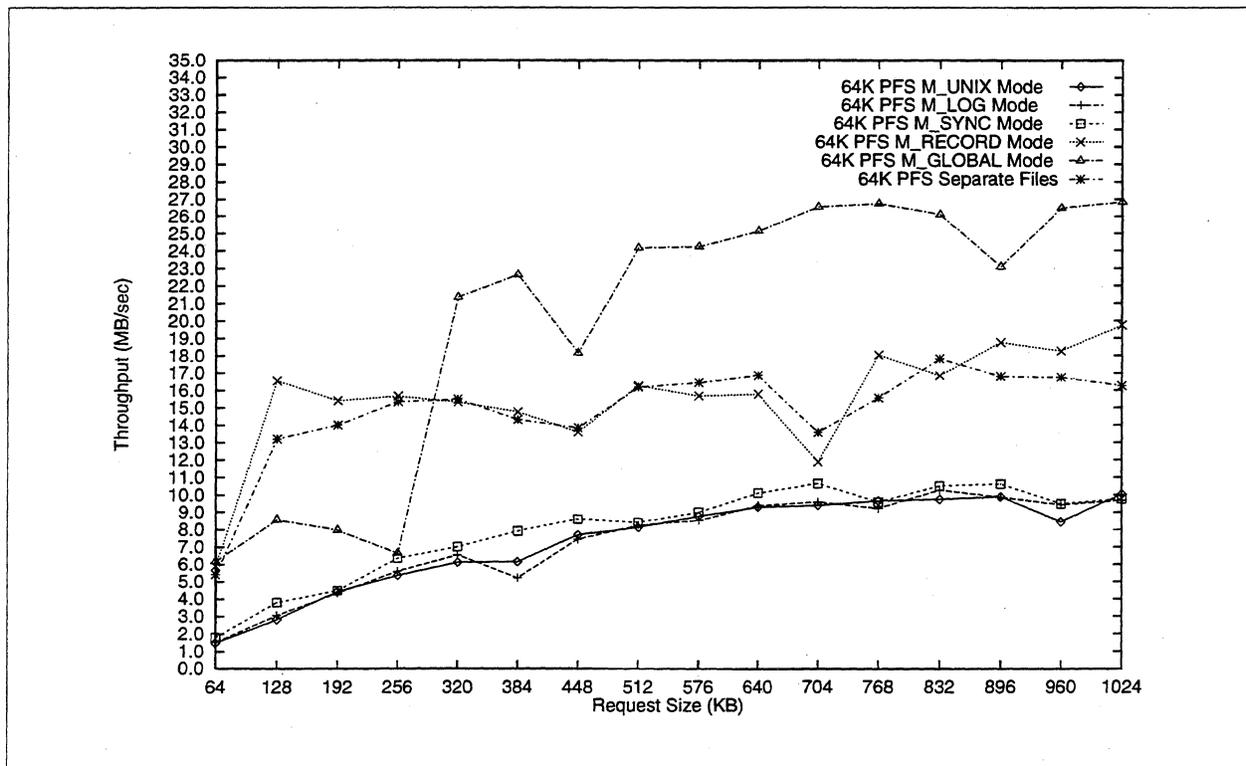
Figure 3-6. 64 KB PFS Read Performance (8 Compute Nodes, 8 I/O Nodes)
