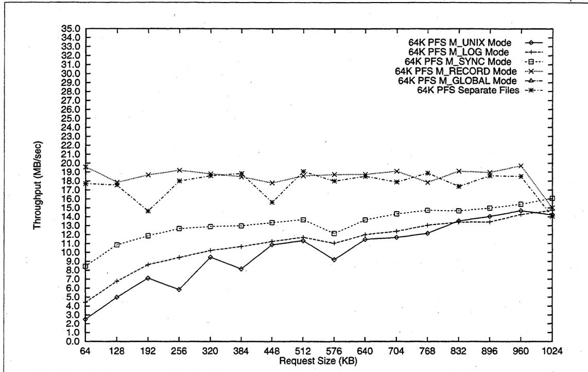
Figure 3-5. 64 KB PFS Write Performance (8 Compute Nodes, 8 I/O Nodes)
