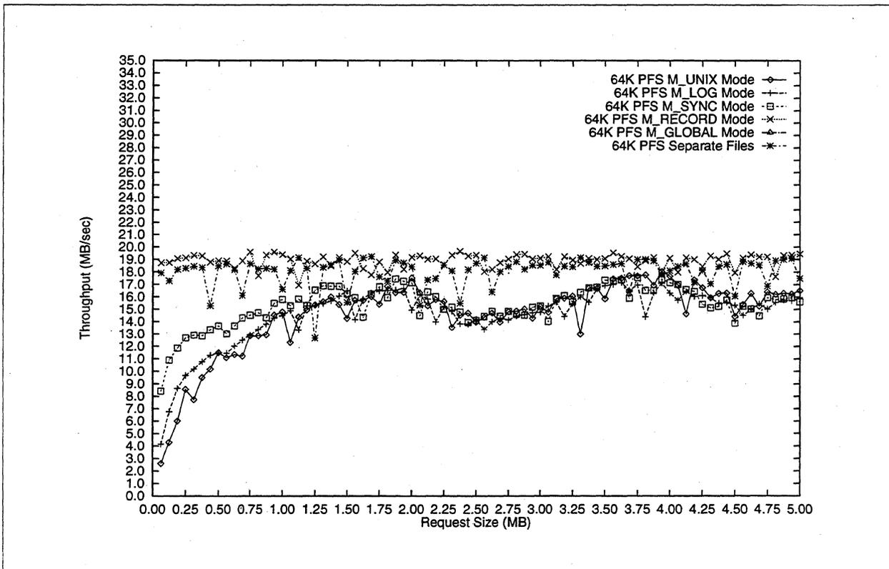
Figure 3-7. 64 KB PFS Write Performance (8 Compute Nodes, 8 I/O Nodes)
