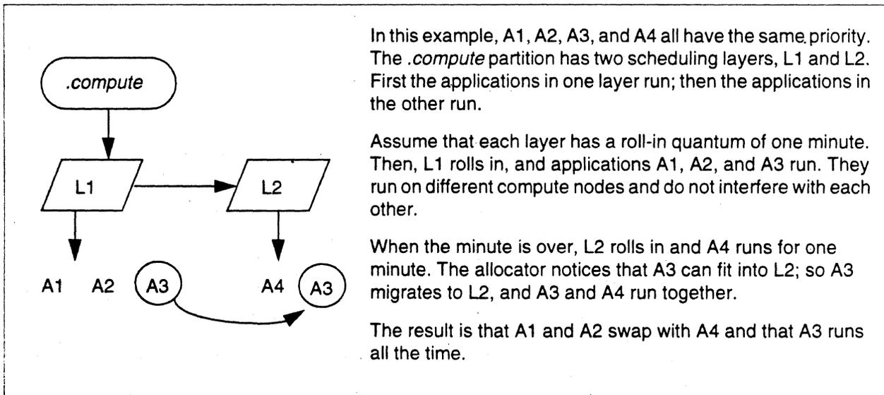
Figure A-2. How Applications Run in Two Scheduling Layers
