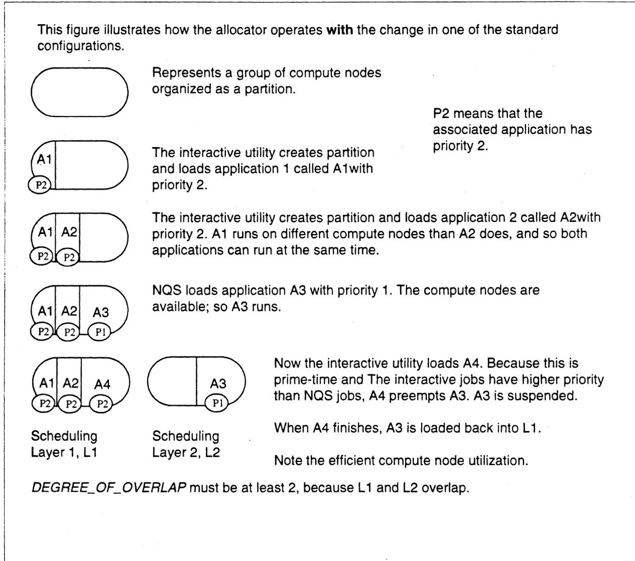
**Figure A-10. Standard NQS/Interactive Configuration with Allocator Change.**
