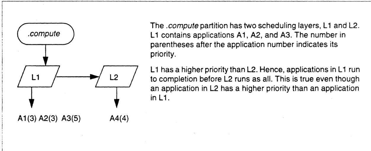
**Figure A-4. How Applications Run in Two Scheduling Layers (with priority)**
