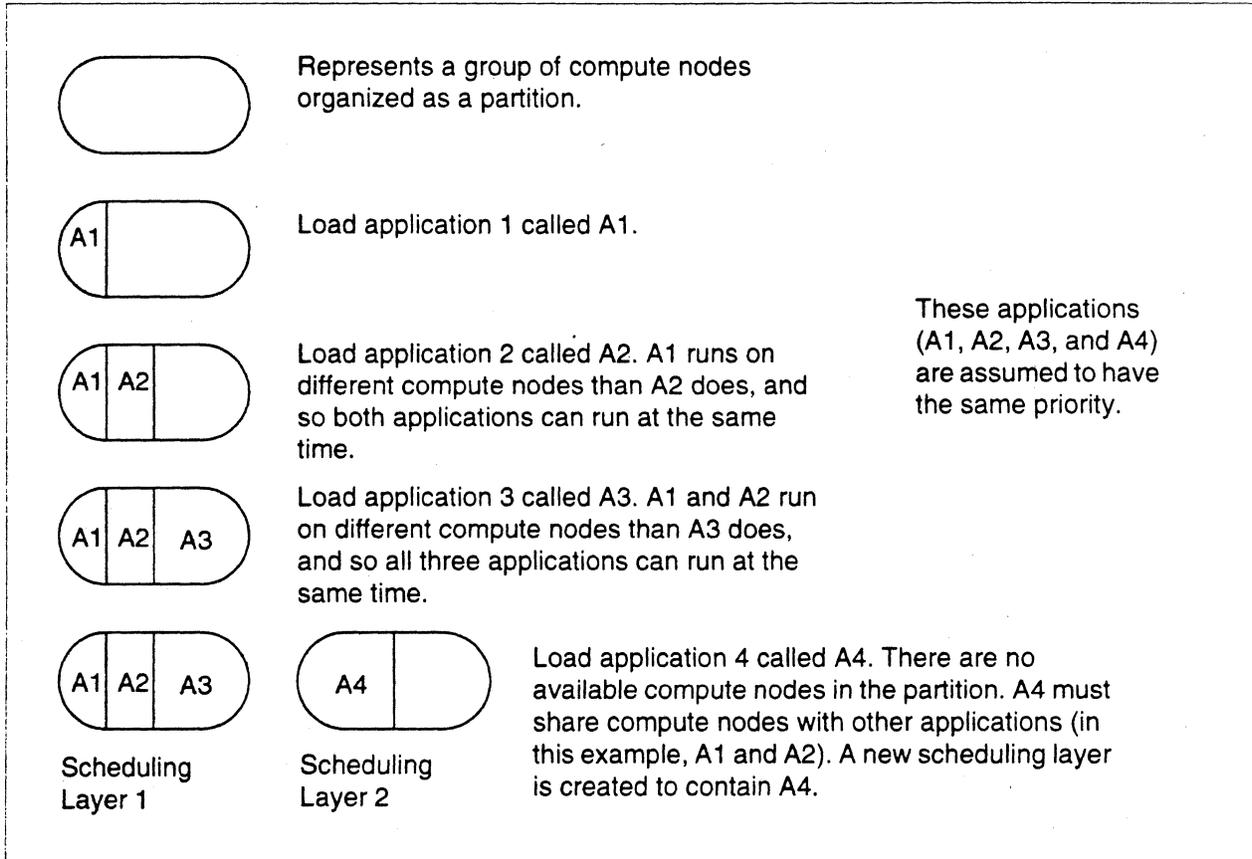
Figure A-1. Loading Applications and Making a Scheduling Layer
