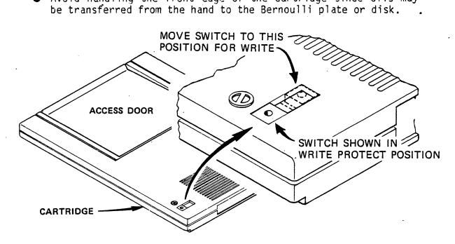
Figure 20. Cartridge with Write Protect Switch
