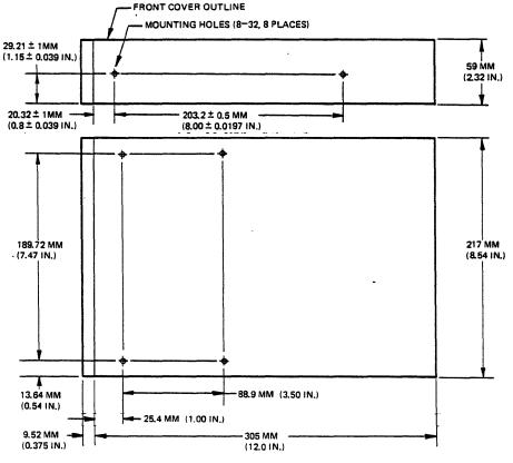
Figure 10. Drive Mounting Hole Locations
