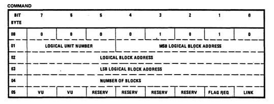
The READ DATA command initiates a transfer of data from the disk subsystem to the host. The starting block is specified by bytes 01, 02, and 03 of the CDB; and the number of blocks to be transferred is given in byte 04.
