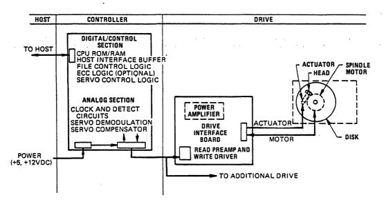
Figure 2. Disk Drive/Controller Architecture
