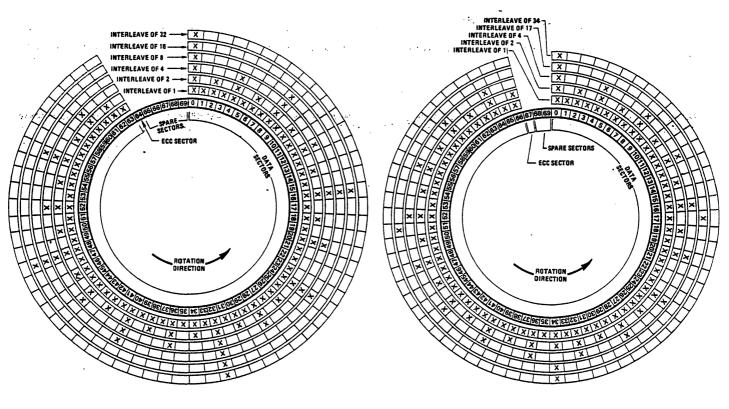
10 MEGABYTE INTERLEAVE INTERLEAVES OF 1, 2, 4, 8, 16, AND 32 ARE POSSIBLE. 10.5 MEGABYTE INTERLEAVE INTERLEAVES OF 1, 2, 4, 17, AND 34 ARE POSSIBLE
