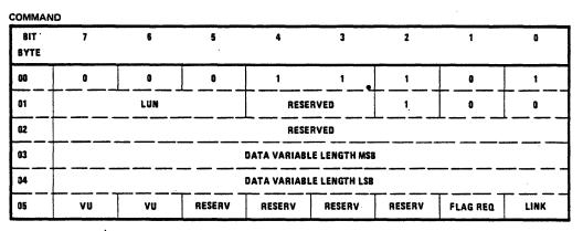
The SEND DIAGNOSTIC Command allows the host to invoke the startup diagnostic routines described in subsection 3.3 on the specified LUN. The controller will go off-line until the diagnostics are completed. Byte 02 must be issued as shown; the other SCSI options for this command are not supported. Any other configurations will generate an Illegal Request error.
