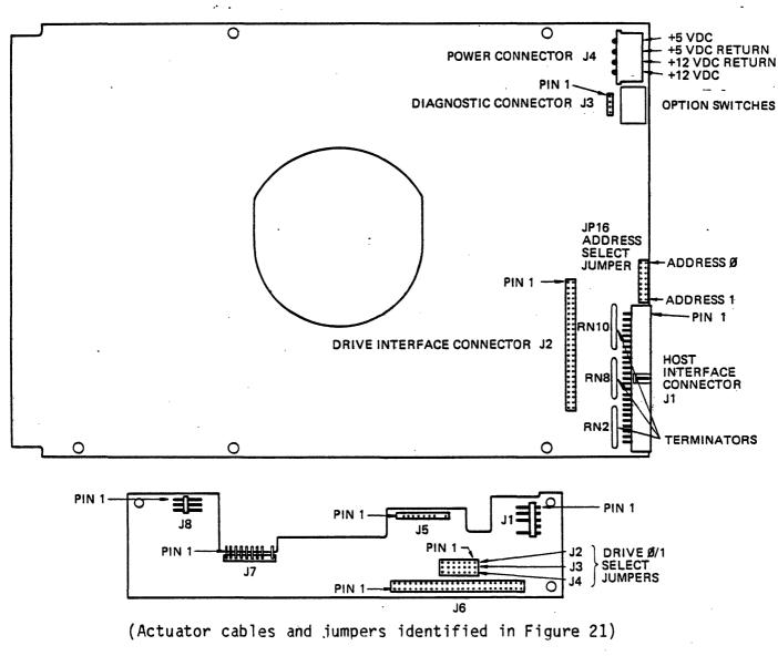
Figure 23. Digital Controller Terminations and Address Options
