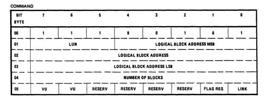
The READ LONG command functions identically to the READ DATA command, unless a CRC error is encountered. If a CRC error occurs using the standard READ
