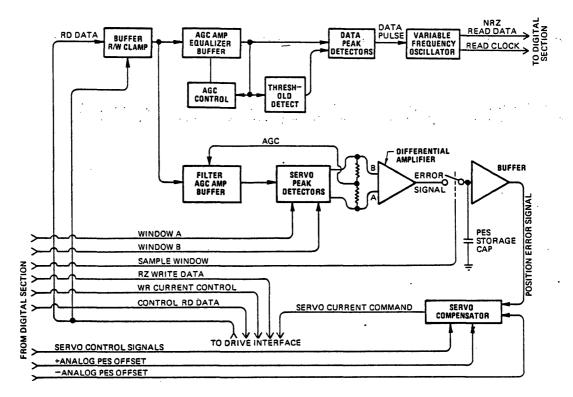
Figure 4. Block Diagram of the Subsystem Analog Functions
