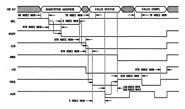
Figure 16. Hardware Busy Status Transfer Timing
