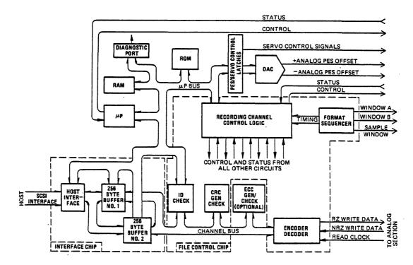
Figure 5. Block Diagram of the Subsystem Digital Functions
