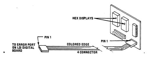
Figure B-3. Error Readout Assembly
