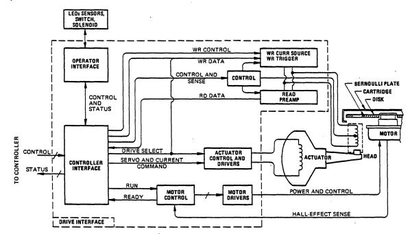
Figure 3. Block Diagram of the Subsystem Drive
