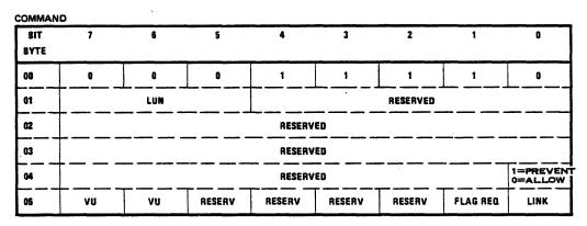
The PREVENT/ALLOW MEDIA REMOVAL command allows the host to prevent removal of the cartridge at an undesirable time, such as when updating a directory or packing the files on the device. This command works by instructing the controller not to poll the bezel switch on the specified drive. The command
