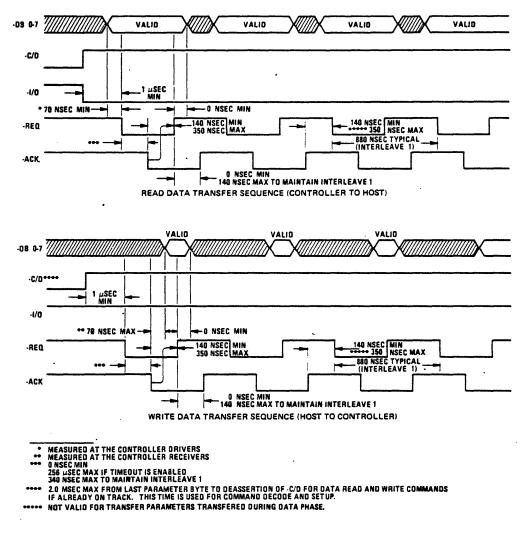
Figure 14. Data Transfer Sequence Timing
