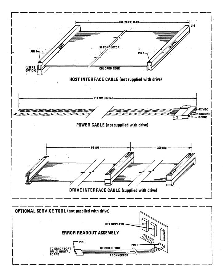
Figure 22. Cabling and Connector Requirements
