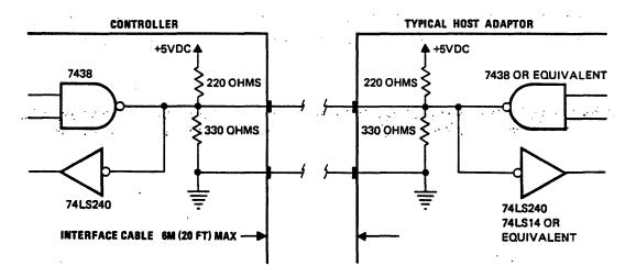
Figure 17. Host Adapter Bus Termination
