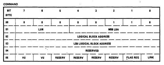
The FORMAT TRACK command allows the host to initiate a media checking/formatting sequence similar to the FORMAT UNIT command, but on a track basis rather than with the entire media. The track's sector IDs will be resequenced, the track checked for media defects, and sectors spared for any identified defects. If no spare sectors are available, the track will be spared. Recovery of user data for this track is not possible once execution of this command begins.
