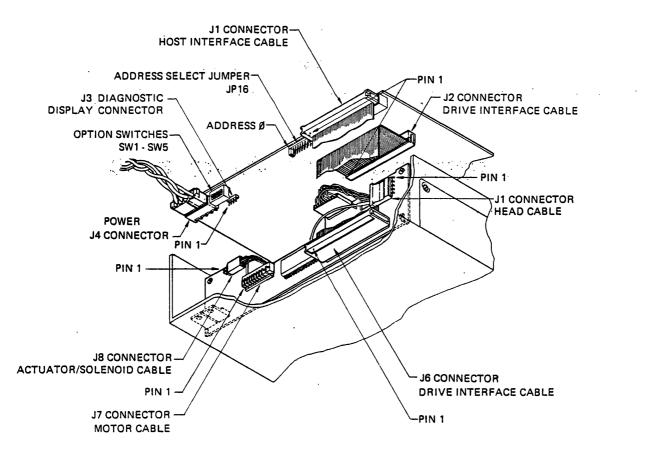
Figure 21. Printed Circuit Board and Main Cable Locations
