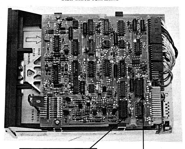
1E For Drive A: Pins 1-14 + 2-13 jumpered
