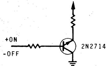
In this connection the transistor gain is less than unity — base drive must be greater than current switched. The advantage is that (nominally) emitter and collector assume identical voltages. In other words, there is zero collector-emitter drop.
