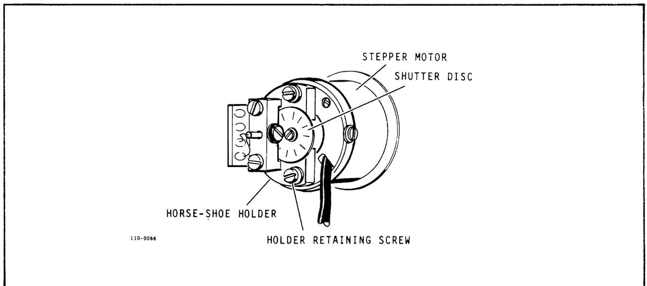
**Figure 5-3. Photo Shutter Adjustment**
