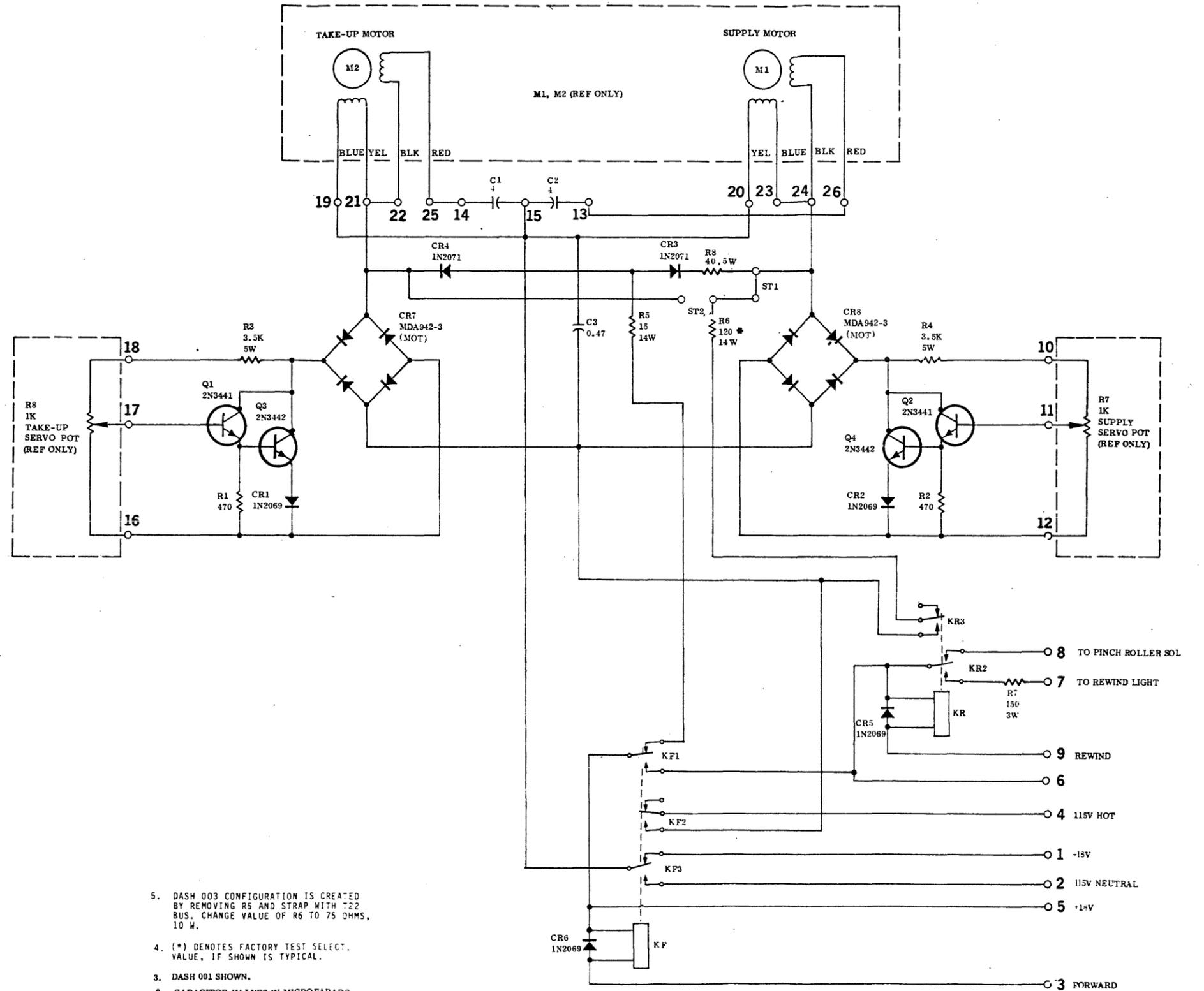
5. DASH 003 CONFIGURATION IS CREATED BY REMOVING R5 AND STRAP WITH T22 BUS. CHANGE VALUE OF R6 TO 75 OHMS, 10 W.
