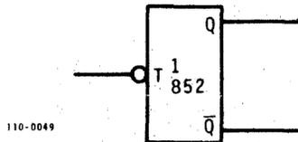
When R-S flip-flops are J-K connected the cross connection is indicated but not drawn:
