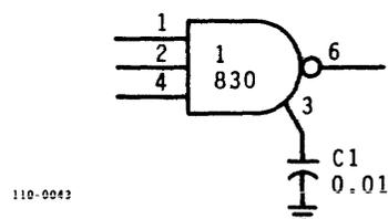
The output is delayed in going to ground by an amount proportional to capacitor size. Positive going output is not appreciably affected.
