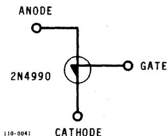
The SUS conducts at an anode voltage of about 7 volts if the gate terminal is open. Once fired the device continues to conduct until current drops below a threshold value.
