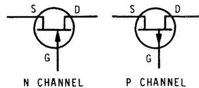
The N channel FET is conducting when 0 volts is applied to the gate and cuts off with negative gate signal (like a vacuum tube). No gate current flows.
