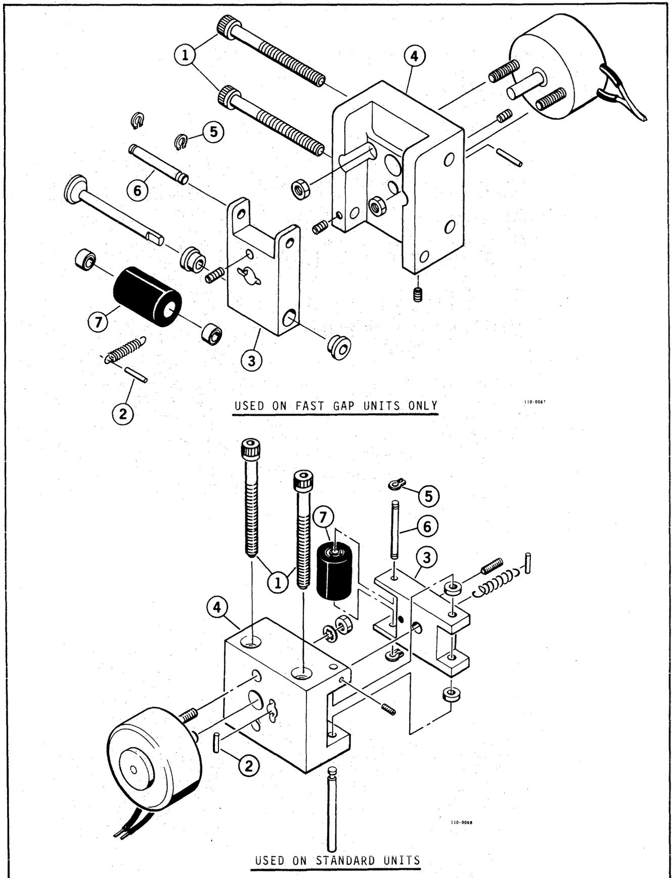
**Figure 5-4. Pinch Roller Replacement**
