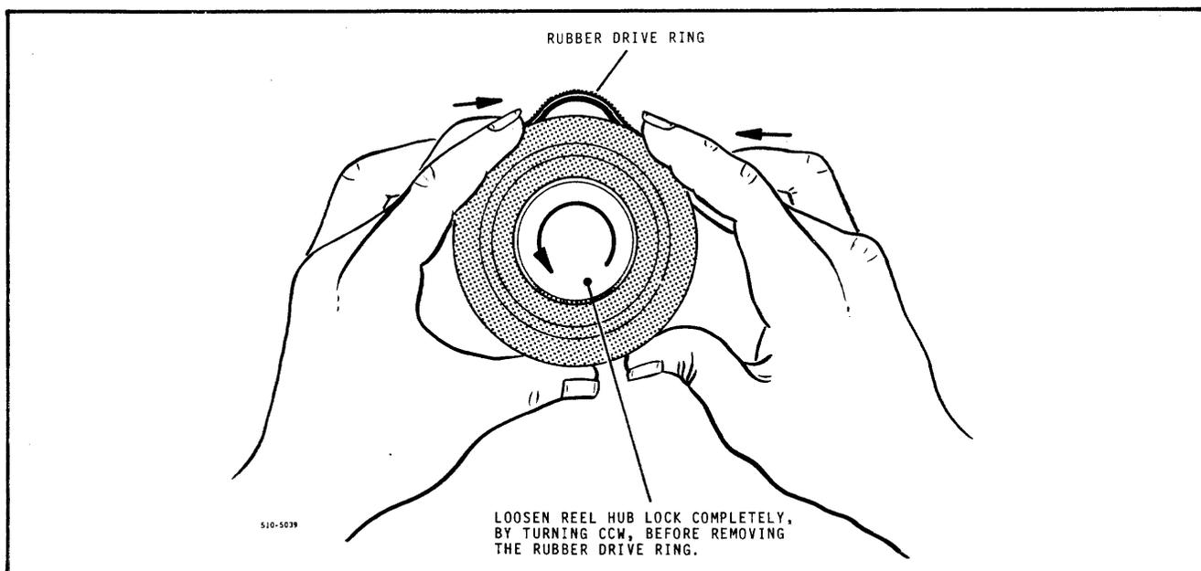
**Figure 5-5 Rubber Ring Drive Replacement**
