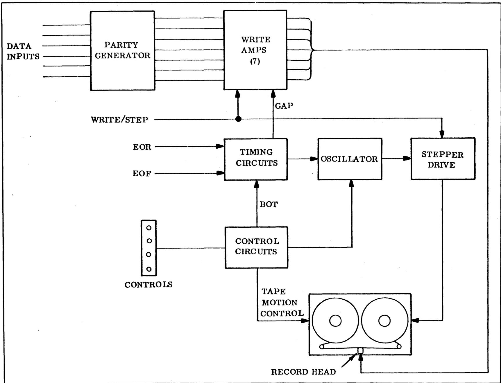
Figure 1-1. Incremental Recording System
