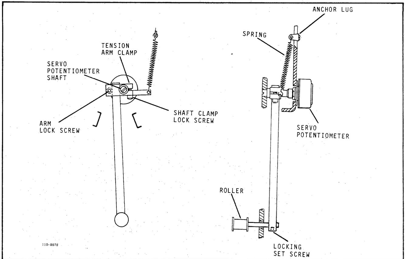
**Figure 5-1. Tension Arm Adjustments**
