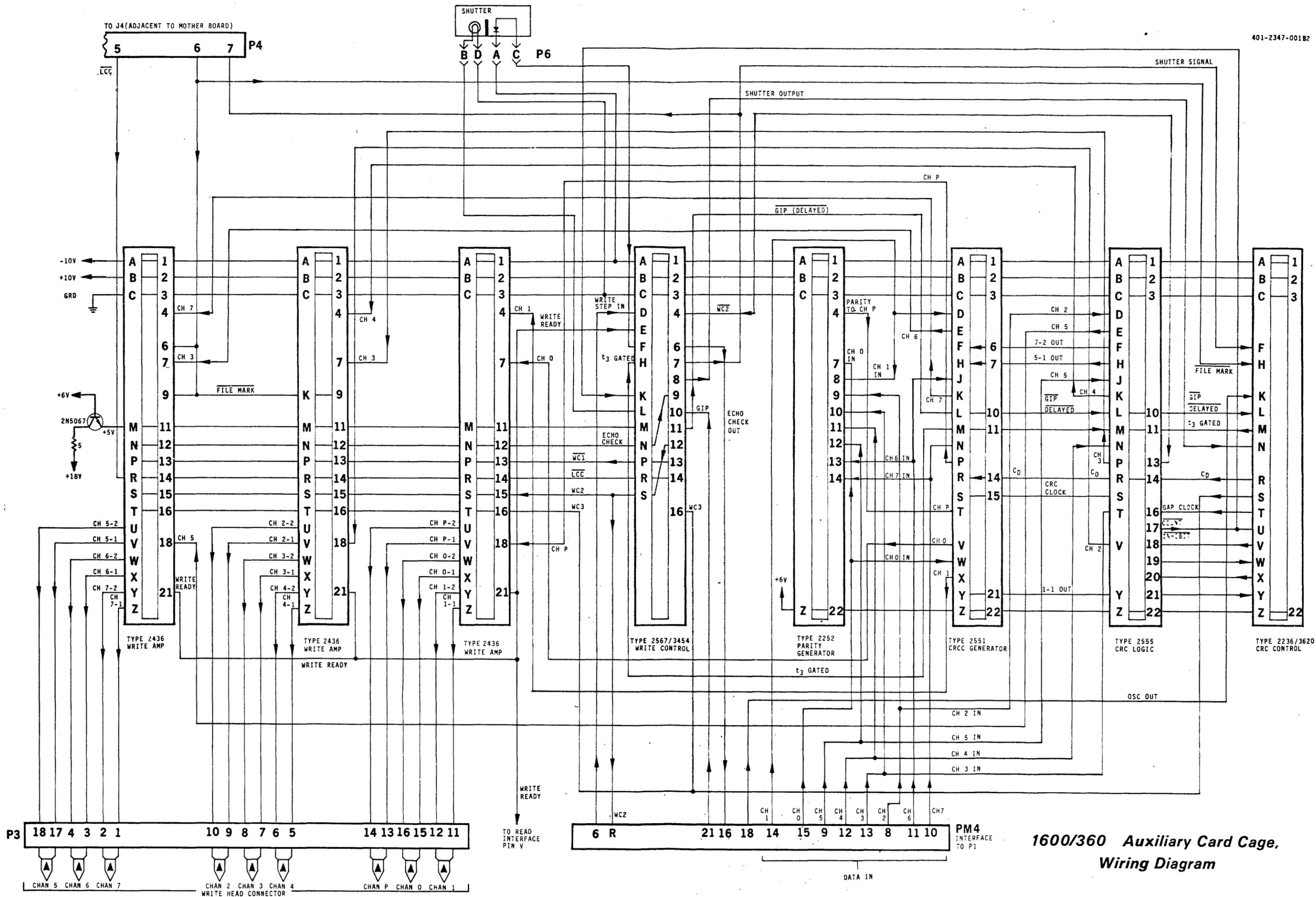
1600/360 Auxiliary Card Cage, Wiring Diagram
