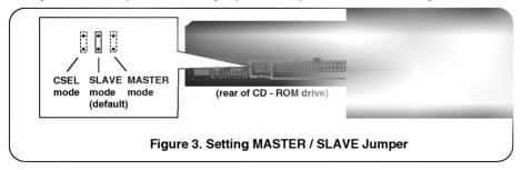
\* Move the jumper (clip on one pair of pins) from its default factory position (SLAVE), to CSEL or MASTER as needed (see the following description for the setup that matches your system), using the above diagram to place the jumper.
