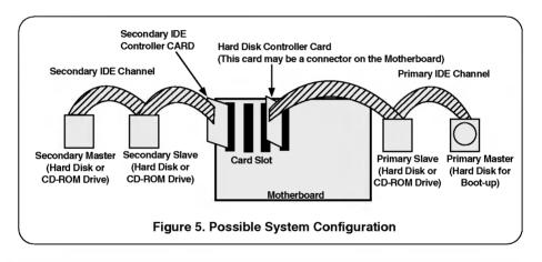
If you have the system with two IDE channels (in the case of an enhanced IDE PC), do not install an IDE controller card in your system.
