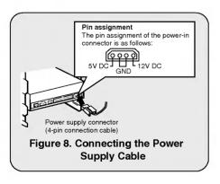
Step 5. Push the power supply cable connector firmly into the power in connector.
