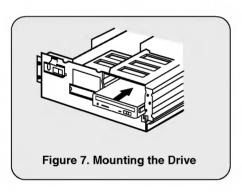
**Step 4.** Slide the CD-ROM drive into the half-height slot, and secure the drive in place with screws and brackets.
