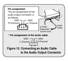
If you want to connect audio equipment or a sound card to the CD-ROM drive, use an audio cable to connect the drive to the sound device.
