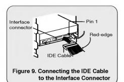
Step 6. Connect the 40-pin IDE Cable to the back of the CD-ROM Drive. Please make sure that the red edge of the IDE Cable is connected to Pin 1 on the CD-ROM Drive.
