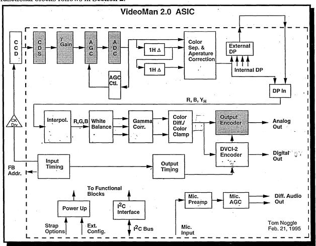
Figure 1 VASIC Functional Block Diagram
