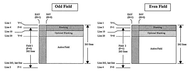
Figure 4c - CCIR656-NTSC and 640x480 Square Pixel @60Hz (Full Frame Rate)
