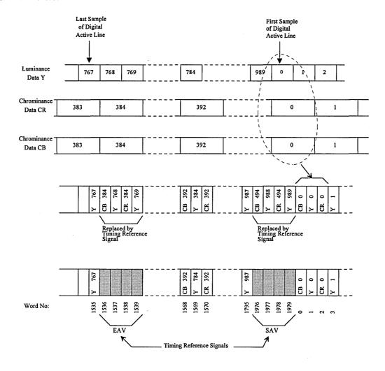
Figure 2f - Multiplex structure, 768x576 Square Pixel
