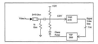
Bias setting is done by balancing of the combination of the pullup and pulldown resistors and the digitally produced low going clamping pulses. These clamping pulses (low signals) are generated by the VSP 2860 chip that forward bias the diode effectively grounding the bottom bias resistor.
