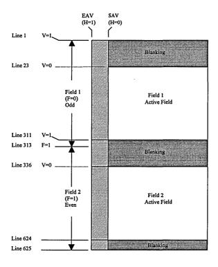
Figure 4b - Video timing reference signal locations, 625-line systems
