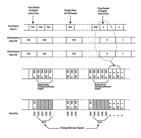
Figure 2e - Multiplex structure, 768x576 Square Pixel
