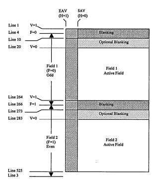
Figure 4a - Video timing reference signal locations, 525-line systems
