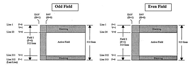
Figure 4d - CCIR656-PAL @50Hz (Full Frame Rate)
