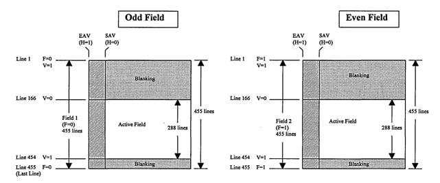
Figure 4f - 768x576 Square Pixel @30Hz (Half Frame Rate)
