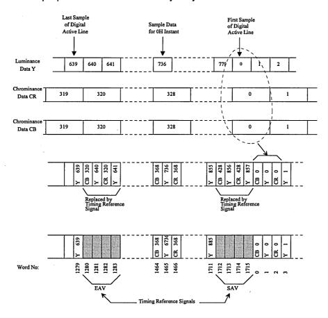
Figure 2g - Multiplex structure : 640x480 Square Pixel
