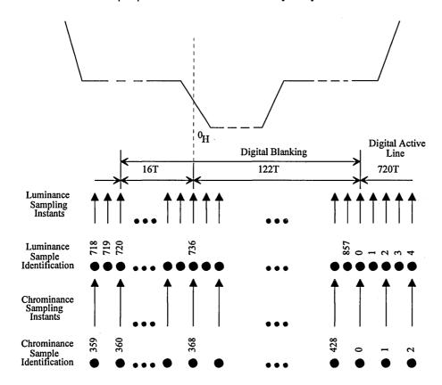
Figure 2a - Horizontal sync relationship, CCIR656-NTSC (60Hz) and Modified 30Hz PAL
