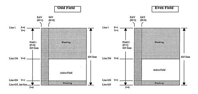
Figure 4g - CCIR656-PAL @ 25Hz (Half Frames Rate)
