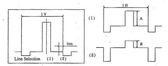
Note 1) To measure the smear signal, use the average function of the oscilloscope to improve accuracy.
