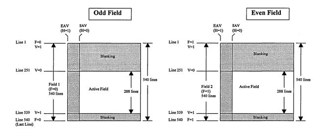
Figure 4e - 768x576 Square Pixel @ 25Hz (Half Frame Rate)
