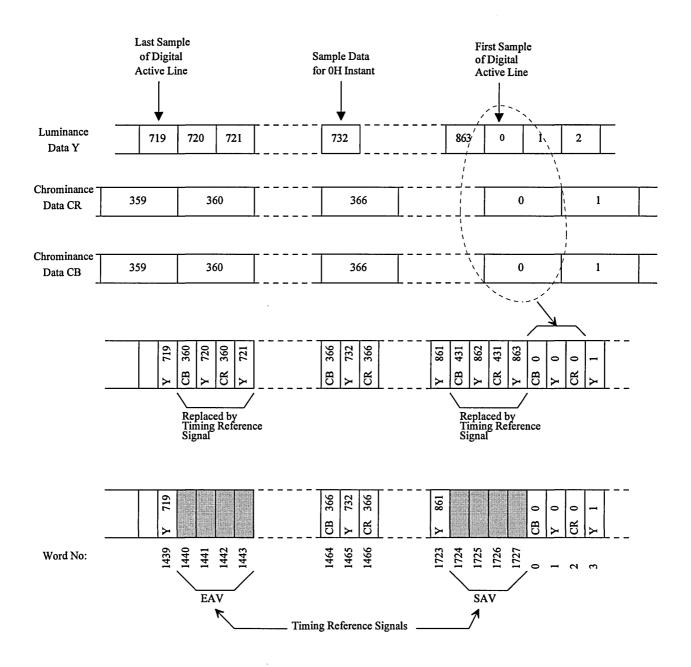
Figure 2d - Multiplex structure, CCIR656-PAL (50Hz) and Modified 25Hz CCIR656-PAL
