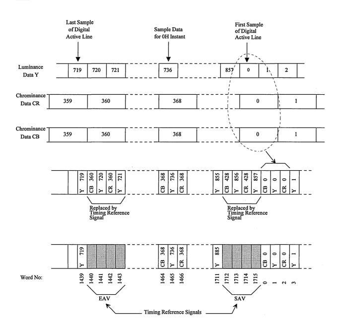
Figure 2b - Multiplex structure, CCIR656-NTSC (60Hz) and Modified 30Hz PAL
