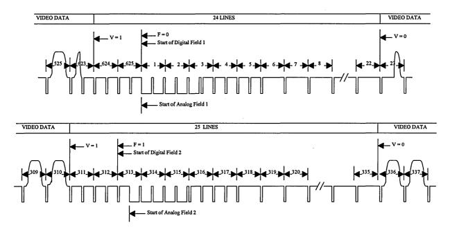
Figure 3b - Relationship of video data and vertical sync, 625-line Systems Used by CCIR656-PAL and modified CCIR656-PAL format
