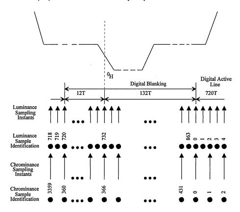
Figure 2c - Horizontal sync relationship, CCIR656-PAL (50Hz) and Modified 25 Hz CCIR656-PAL
