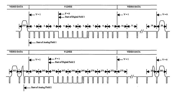
Figure 3a - Relationship of video data and vertical sync, 525-line systems
