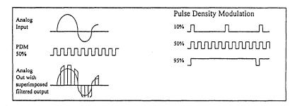
The modulated digital waveform is then multiplied with the audio input signal. The process is ismilar to chipping, and results in an attenuated analog audio signal, as shown above (left). For the WAVE audio, the left and right volume information is carried on a signal line, two lines are used for the other two types of audio signals. The resulting signal is mixed with other audio signals.
