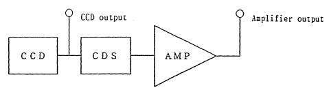
The output voltage is measured at the CCD output. The gain of the amplifier is adjusted to the unity between the CCD output and the Amplifier output.
