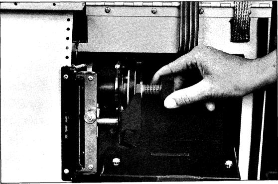
Figure 7. Aligning Top of Form
