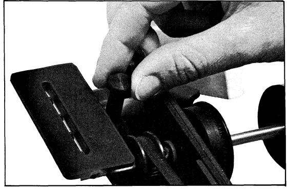
Figure 48. Adjusting for paper width
