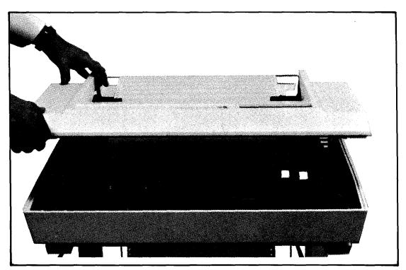
Figure 42. Opening printer cover
