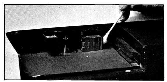
Figure 38. Cleaning head guides
