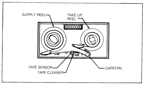
Figure 2. Tape Threading
