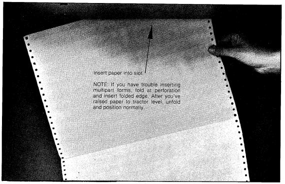
Figure 4. Inserting Paper
