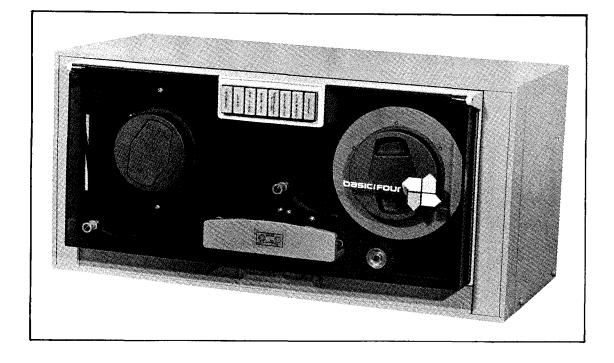
The magnetic tape drive provides a means of storing large volumes of data. This unit can be used in applications where the faster data access time of the disc drive is not needed.
