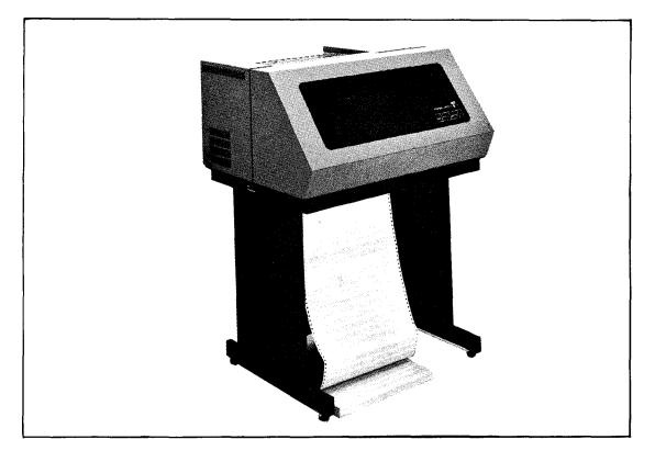
These line printers produce large volumes of forms and reports at a rate of 150 or 300 lines-per-minute, in addition to having the capability of plotting graphs. They are free-standing and have an enclosure to reduce printer noise.
