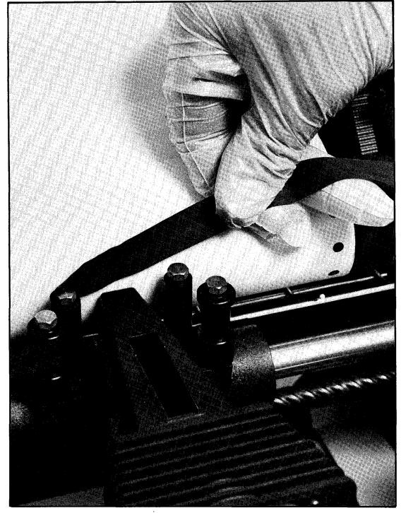
Figure 56. Threading ribbon around printer head
