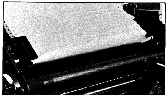
Figure 49. Paper aligned incorrectly
