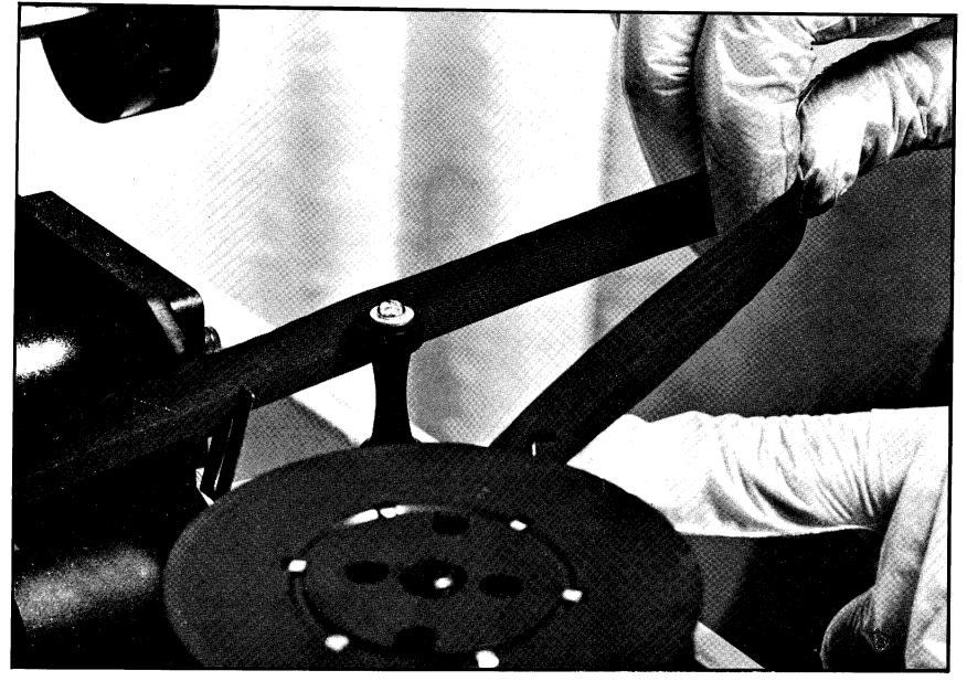
Figure 57. Lifting new ribbon over righthand tension arm
