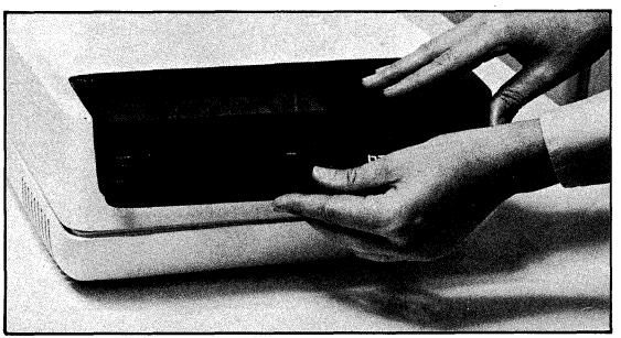
*Figure 36. Removing tape drive unit cover*
