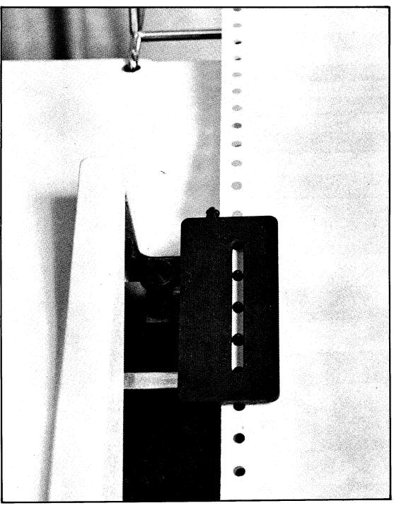
Figure 43. Tractor holding paper in place
