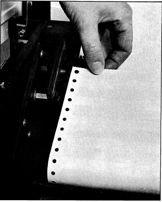
*Figure 46. Placing paper holes on opened tractor*
