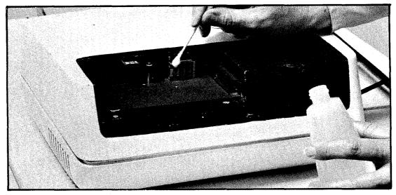
Figure 37. Cleaning head surfaces
