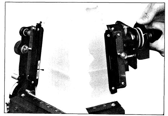
Figure 6. Aligning First Print Line Position
