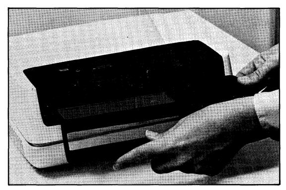
Figure 40. Replacing tape drive unit cover
