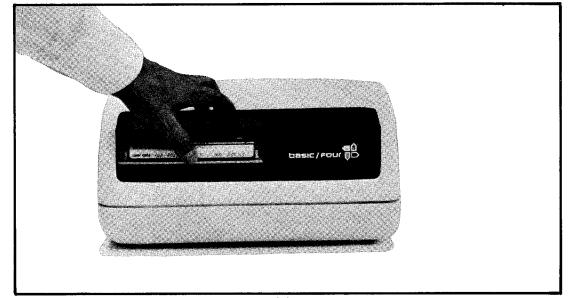
Figure 15. Inserting tape cartridge
