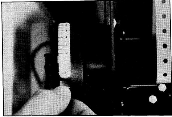
Figure 52. Adjusting for forms of different thickness
