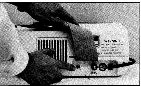
Figure 13. Tape cartridge drive power switch
