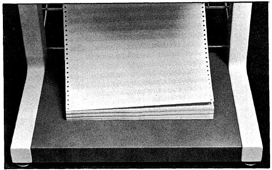
Figure 41. Paper stacked on printer base
