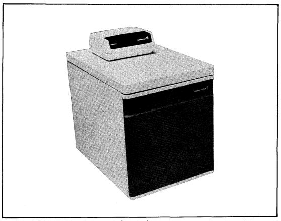
Figure 8. Central processing unit
