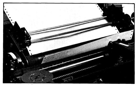
Figure 45. Threading paper under platen
