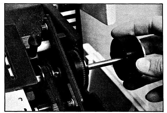
Figure 51. Adjusting paper with platen knob
