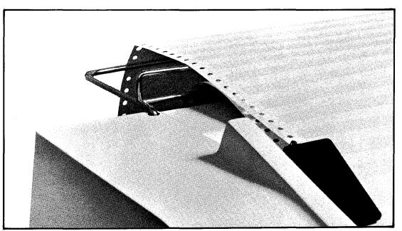
Figure 50. Threading paper back over top rack
