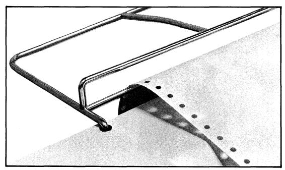
Figure 44. Threading paper between rods 6 and 7
