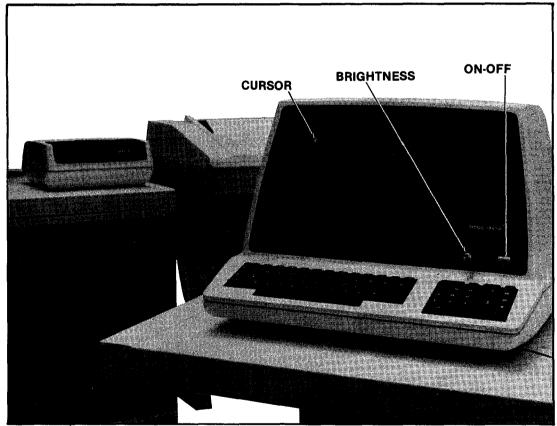
Figure 7. VDT front controls
