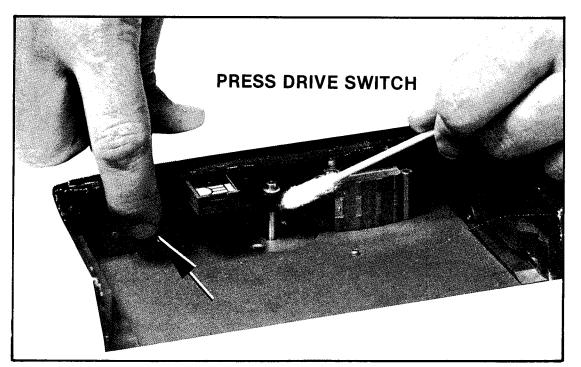
Figure 39. Cleaning motor capstan
