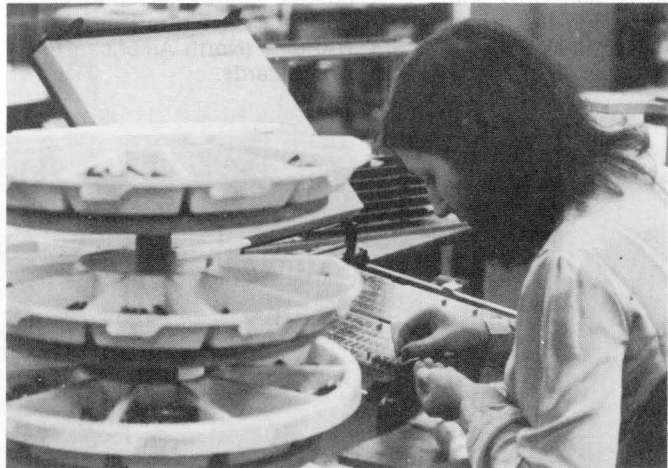
Figure 6. A manual assembly area is used for low-volume standard products or custom products.
