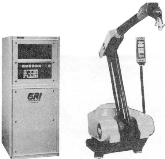
Figure 4. Matrox MTX-1632 Video RAM is used in the console of this industrial robotics system. (photo courtesy of Graco Robotics Inc.)
