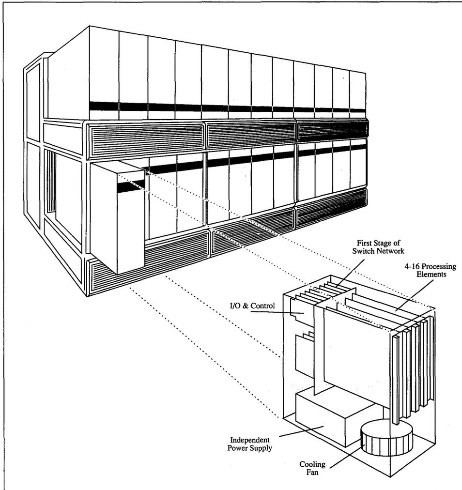
Modules are rack mounted and inter-connected in groups of 4. The 24 module system illustrated supports up to 256 superscalar SPARC PEs. Extension of this system is straightforward, with large systems constructed from multiple modules connected by a central switch.
