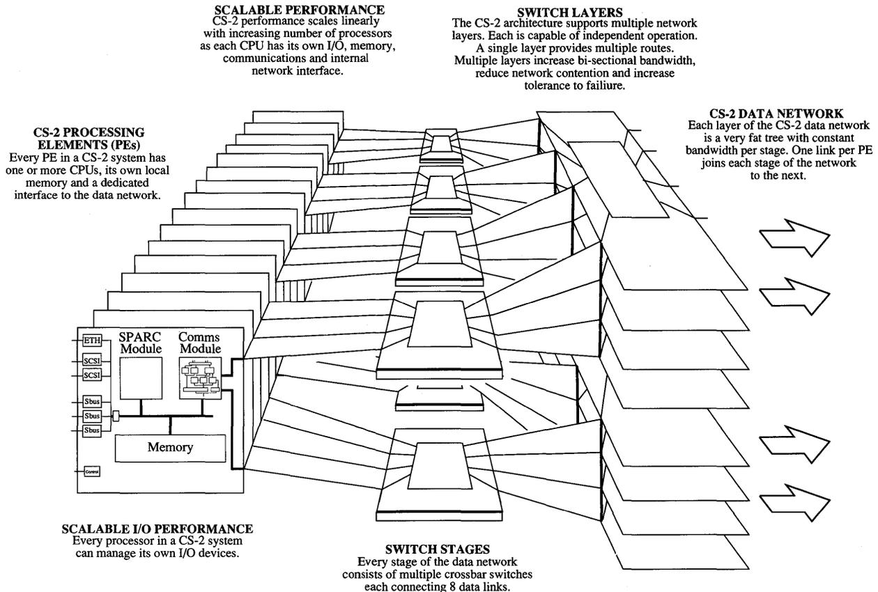
The distributed memory architecture guarantees a constant ratio of CPU performance, to memory and I/O bandwidth whatever the size of system giving scalable, balanced system performance.
