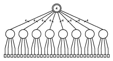
Allocation of Elan Id's becomes more complex when SPARC/Compute boards and single SPARC boards are both installed in the CS-2 system. Modules populated with SPARC/Compute boards include one level of switching integral to the module, whereas modules with single SPARC processor do not. Networks consisting of mixed module types have processors at more than switch level.
