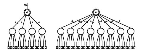
We use a binary form for network size, equal to the number of bits in the network identifier of the lowest processor in the network. This is used because the top stage of the network can use either 4 or 8 links.
