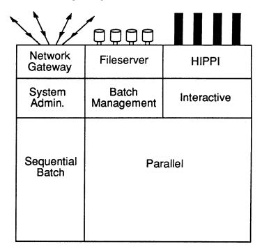
Users login to the system and are connected to processors in the *interactive* partition. The connections are managed by processors in the *network gateway* partition, which are dedicated hosts of the network adaptors and *login load balancers*; these processors do not run user processes.
