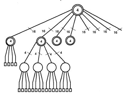
In this case all network routes are expressed by three components; processors on level 2 have do not need the third component so it is always set to zero. This means that the single SPARC boards at level 2 have Elan Id's that increment by 4.
