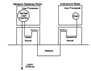
The connection between the original login daemon process and the shortcircuited link is set up as a loopback link, simply forwarding data in and out of the short-circuit and acting as a kernel gateway for the login connection. The ptsfilt streams module is pushed onto this loopback, to allow the login daemon to perform its internal communications with the remote pseudo terminal link.
