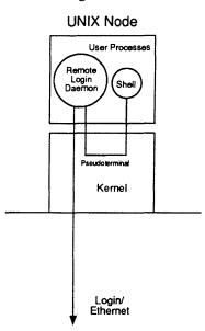
When using the login load balancer a TCP/IP link is created to connect the incoming login request stream and a pseudo terminal on the load balanced node. Two processes act as endpoints for this connection — logbalclient and logbalserver (see Figure 2-3).
