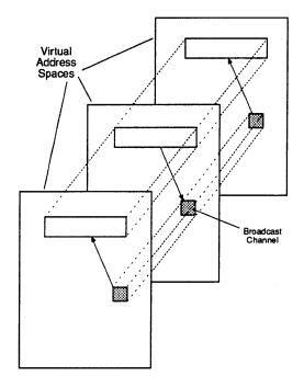
A broadcast channel is a global object. It is used to barrier synchronise and replicate the slices of other global objects. See EW\_BCHAN. It has a non-blocking interface which allows up to one outstanding broadcast at a time. Multiple broadcast channels may be used by a group of processes to allow more outstanding broadcasts.
