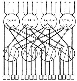
Figure 3-2 Shift by 5 on a 16 processor CS-2 network.
