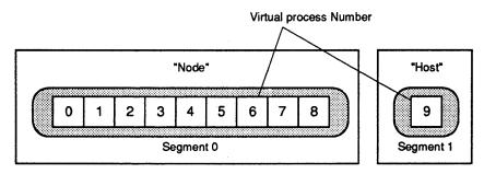
All processes in all segments of a parallel application start up together. This assigns every process a unique virtual process number in a contiguous range starting from 0, and makes every process's address space accessible to its peers through the network. For more information see ew init().
