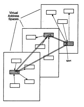
Tagged messages are passed between tagged message passing ports, called tports. See EW\_TPORT. They support both buffered and unbuffered message passing, with a non-blocking interface which allows arbitrary numbers of out standing transmits and receives. Messages may be received selectively, both ( the sender and on the tag. Given equivalent selection criteria, messages passe from the same source to the same destination remain ordered.
