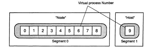
Every process in a parallel program has a unique process id; this is translated to a physical processor id by the inter-processor communication hardware. The ordering of segments and hence the numbering of processes depends upon the programming model; some number the controlling (or host) process 0 and the processes of the parallel program 1,2,...,n, others number the parallel program 0,1,2,...n-1 and the host n.
