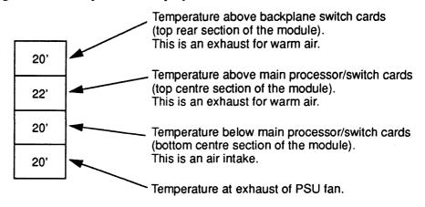
The mapping from displayed temperatures to sensors position in the disk modules is shown below:
