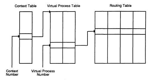
Virtual process IDs are translated through a per context virtual to physical processor translation which points at the route bytes needed to direct a message to this processor.
