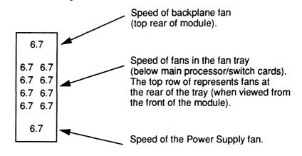
The mapping from displayed speeds to the fan positions in the disk modules is shown below:
