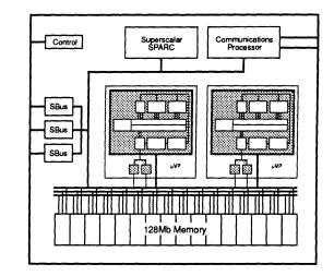
The memory system is implemented as 16 independent banks, with a (current) total capacity of 128 Mbytes. Memory bandwidth for each of the 3 ports is 1.2 Gbytes/s, with a total bandwidth of 3.2 Gbytes/s.
