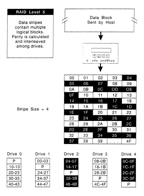
Rather than striping in units of single logical blocks, RAID 5 permits the user to select a stripe size. (The CRD-5000 supports stripe sizes from one to 255 logical blocks.) When the host sends a chunk of data to be written, the CRD-5000 breaks it up according to this stripe size and writes the pieces to one
