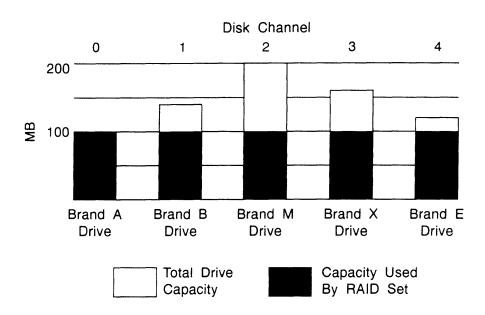
If you wish to enable tag queuing, all drives on the rank must be identical. The CRD-5000 will not support tag queuing, if the drives in a rank are made by different manufacturers. This is because all drive manufacturers do not implement tag queuing in the same way.
