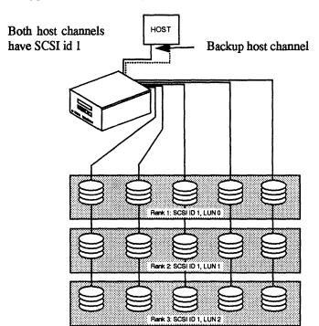
Figure A-1 Typical RAID Configuration
