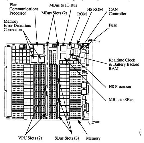
Figure 2-1 Board Schematic Showing Major Components (MK403)
