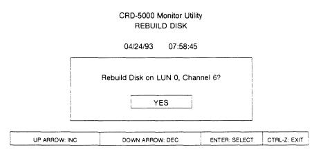
Use the arrow keys to toggle between "YES" and "NO." If you select "NO," the monitor utility will search for the next eligible disk drive and repeat the above display with that drive's LUN and channel. A "YES" selection will begin the rebuilding process and the following screen will appear.
