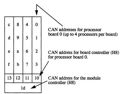
Figure 1-5 CAN Addresses within a Module
