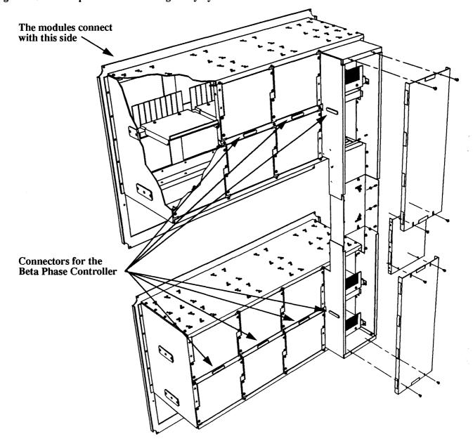
Figure 4-3 Backplane Box for a Single Bay System
