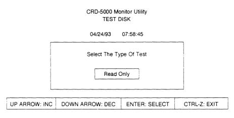
Use the arrow keys to toggle between the read-only test and the write/read test. Press Enter to move to the next screen.
