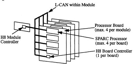
Figure 1-1 L-CAN Connections within a Processor Module
