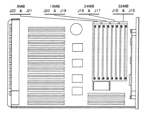
The CRD-5000 is "cache-ready," meaning that the unit will configure itself automatically to use cache as SIMMs are installed.
