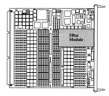
Figure 3-3 Position of SBus Module 0
