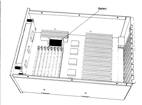
The CRD-5000 drains current from the battery only when primary power is shut off. So for systems that are powered up nearly all the time, the useful life of the battery should approach its shelf life: approximately ten years. The battery on a system that is powered down more often will have a shorter life. The unit will periodically run a battery test and flash an error message on the frontpanel LCD if the current is getting weak.
