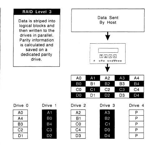
The parity drive virtually guarantees that your data will always be available. RAID cannot make a total guarantee of data availability, however. No RAID level employing parity can survive the failure of a second drive before the first failed drive has been rebuilt. The probability of a second drive failing in the time it takes to rebuild the first drive is very low, however.
