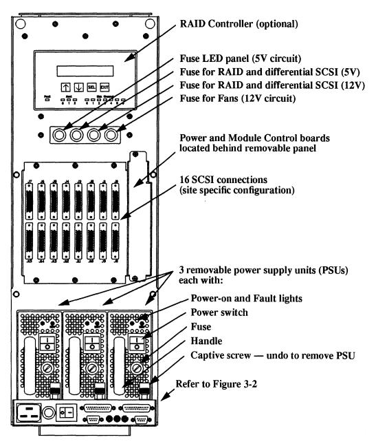
**Meko** Installing the Peripheral Module
