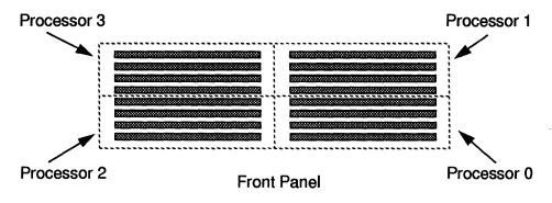
SIMMs can be either 4Mbit DRAM or 16Mbit DRAM technology, either single or double sided. This gives a total minimum memory configuration of 64Mbytes and a maximum of 512Mbytes (16–128Mbytes per processor).
