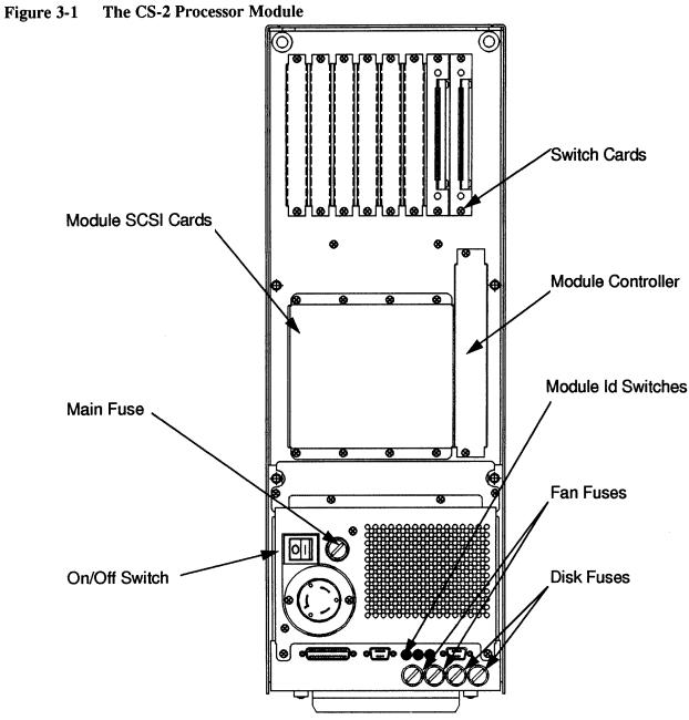
**Meko** Installing the Processor Module
