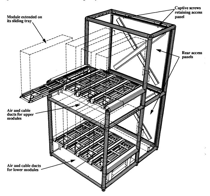
Figure 4-1 Skeletal Illustration of a Single Bay
