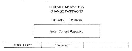
The system asks for the current password to prevent unauthorized password changes. (If you are changing the password for the first time, the default password is 333333.) This screen will continue to appear until either the current password is entered correctly or the user exits by pressing Ctrl-Z.
