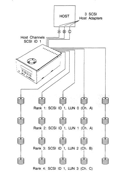
The purpose of this configuration is to break up the data transfer bottleneck that can develop when you have multiple disk channels transferring data from *multiple* ranks to the CRD-5000, which must turn around and transfer all this data to the host on *one* host channel. By dedicating a host channel to no more than one or two ranks, you can lighten the data transfer load that each channel must bear, effectively speeding up performance on the system as a whole.
