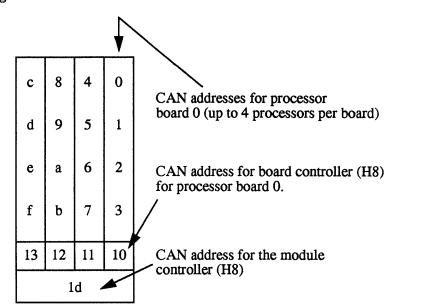
Figure C-1 CAN Addresses within a Module
