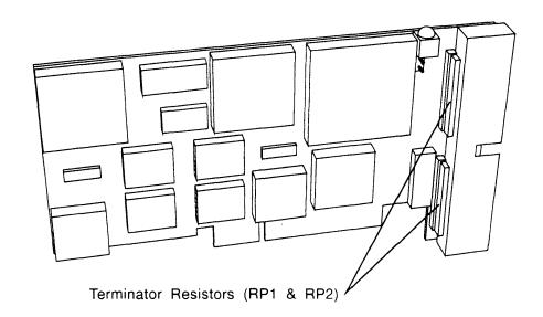
CMD has used active terminators in the CRD-5000. When running in synchronous mode at seven megabytes per second or faster, the SCSI device at the other end of the bus may require special terminators.
