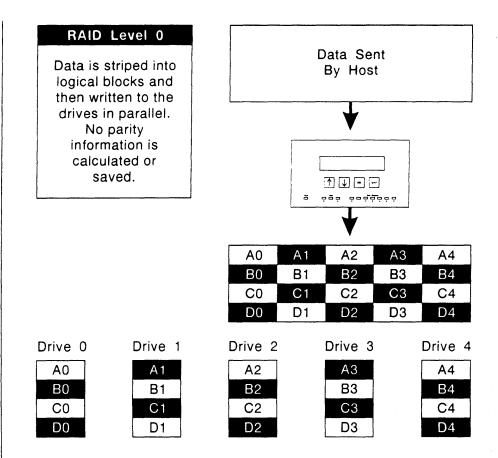
Similarly, when the host issues a read request, the CRD-5000 fetches the data from each drive in the array in parallel.
