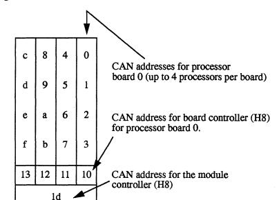
Figure C-1 CAN Addresses within a Module
