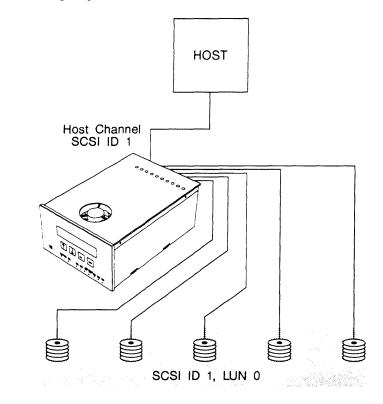
Each drive in the rank must be connected to a separate disk channel. While this configuration is for a five-drive rank, the CRD-5000 will accept as many as seven disk drives on each rank—as long as there is a disk channel module for each drive. All the drives on the rank must have the same SCSI ID. In this case, the host computer is connected to a CRD-5000 host module that has a SCSI ID of one; therefore, the host will recognize the rank by the address SCSI ID 1, LUN 0.
