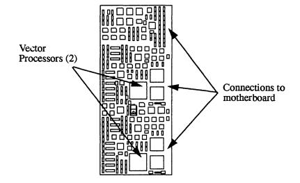
Figure 2-2 Board Schematic Showing Major Components (MK534)
