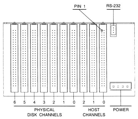
Remember, the disk channel numbers assigned to the slots are just *physical* designations. Once you cable the drives up and create a RAID set, the CRD-5000 will assign *logical* channel numbers to each drive. It is these logical numbers that really mean something to the system. Initially, the logical and physical numbers will be the same. But the CRD-5000 permits you to swap cables and
