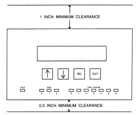
If the CRD-5000 and the disk drives it controls are housed in the same enclosure, make sure the enclosure has its own ventilation system, preferably a fan and vent system that pulls fresh air through the front and exhausts hot air through the back.
