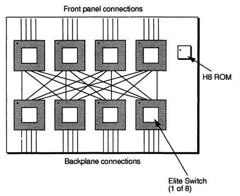
Both the Elite switches and the H8 ROM are held in sockets and can be removed using the appropriate tool. Take care not to damage the component or its neighbours when installing or removing these devices.
