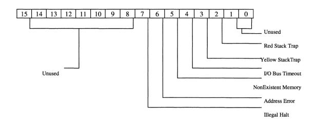
Figure 6.2 CPU Error Register.
