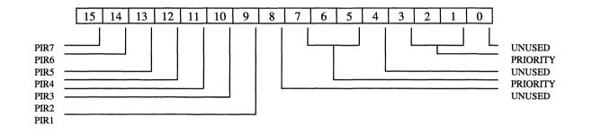
Figure 6.3 Program Interrupt Request Register.
