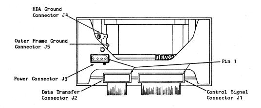
Figure 3-1. Power and Interface Connections
