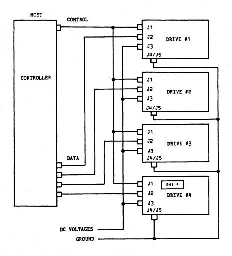
Interface Terminator RN1 is installed <u>only</u> in the last physical drive in the control chain.
