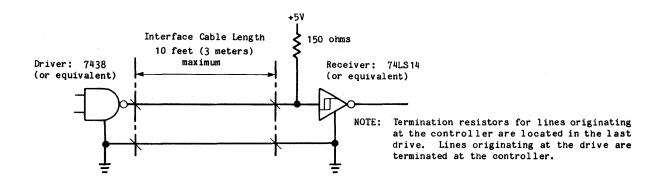
Figure 2-1. Control Signal Driver/Receiver Combination
