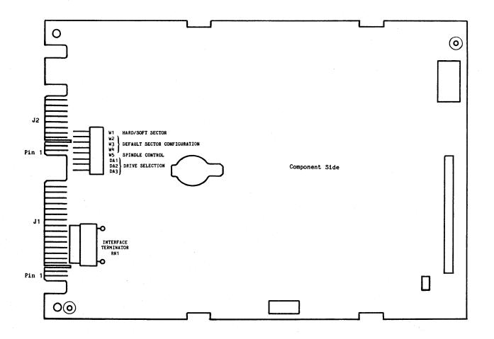
Figure 3-2. Option Jumpers and Interface Terminator
