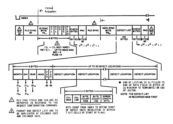
Figure 5-6. Defect List Format
