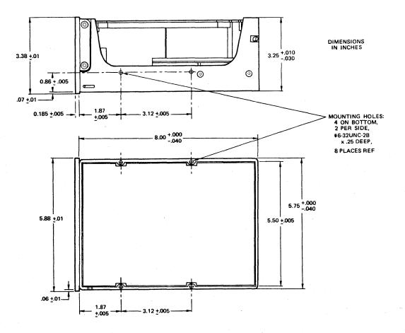
Figure 3-4. Dimensions and Mounting
