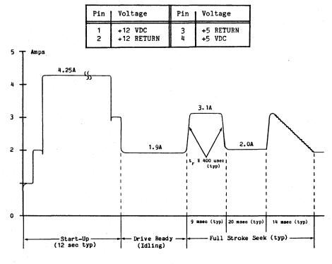
Figure 4-1. 12V Peak Current Profile (typical, 1355)
