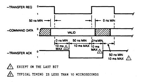
Figure 2-6. One Bit Transfer Timing - To Drive
