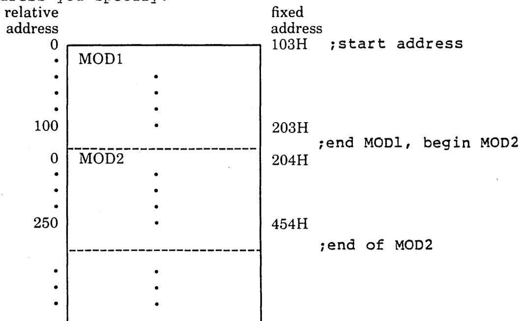
Figure 1.3: Loading Changes Relative Addresses to Fixed
