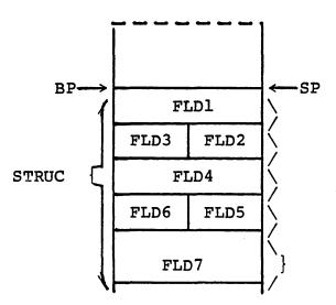
This method makes all values on the stack are available all the time, not just the value at the top. Therefore, this method makes the stack a handy place to pass parameters to subroutines. 3.3 OPERATORS
