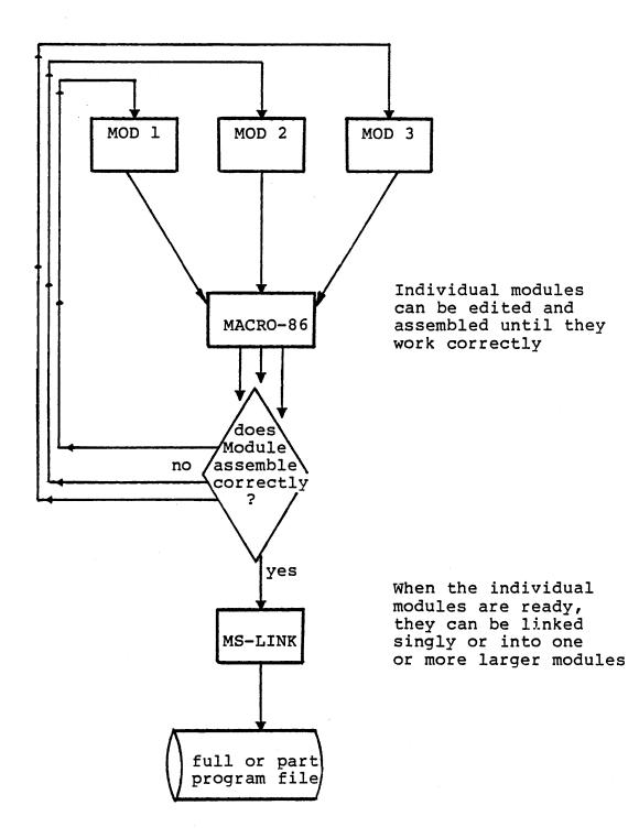
MACRO-86 supports Microsoft's complete 8080 macro facility, which is Intel 8080 standard. The macro facility permits the writing of blocks of code for a set of instructions used frequently. The need for recoding these instructions each time they are needed is eliminated.
