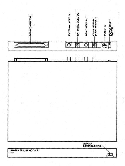
Figure 2-1: The Image Capture Module
