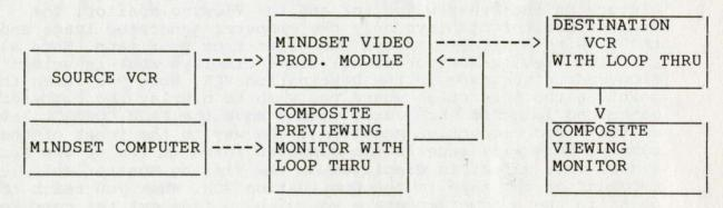
FIGURE 1. PREVIEWING MINDSET GRAPHICS USING A LOOP THROUGH COMPOSITE MONITOR
