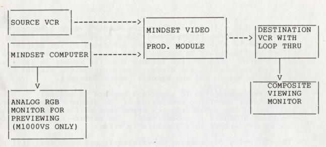
FIGURE 2. PREVIEWING MINDSET GENERATED GRAPHICS USING AN ANALOG RGB MONITOR.
