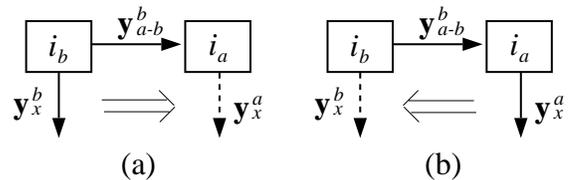
Figure 6: (a) To change the reference frame of flow  $\mathbf{y}_x^b$  from  $i_a$  to  $i_b$ , the  $x$  and  $y$  components are forward warped along  $\mathbf{y}_{a-b}^b$ , producing the dotted flow  $\mathbf{y}_x^a$ . In (b), backwards warping is used to compute the inverse.
