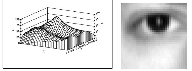
Figure 2: The cross-correlation of the template reported on the right. Note the diffuse shape of the peak that makes its localization difficult
