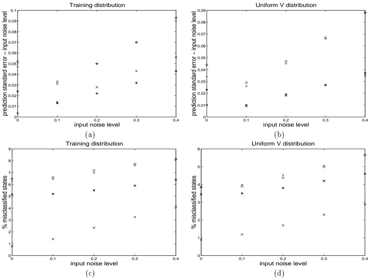
Figure 5: Test set performance of the MME and ME models for various levels of the input noise  $\sigma_{in}$  on two different distributions. (a) and (b):  $(\text{Prediction MSE})^{1/2} - \sigma_{in}$ ; (c) and (d): the percentage of misclassified states.  $\times$  - MME, no noise;  $*$  - MME noise 0.2;  $\circ$  - ME, no noise;  $+$  - ME, noise 0.2.
