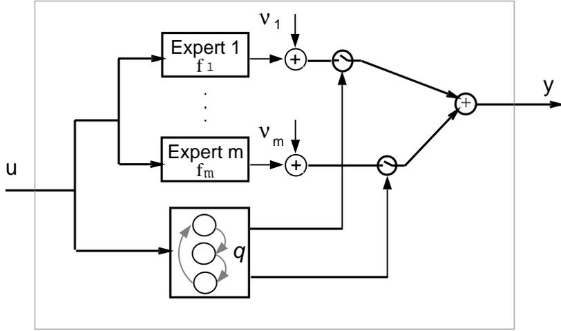
Figure 2: The Markov Mixture of Experts architecture
