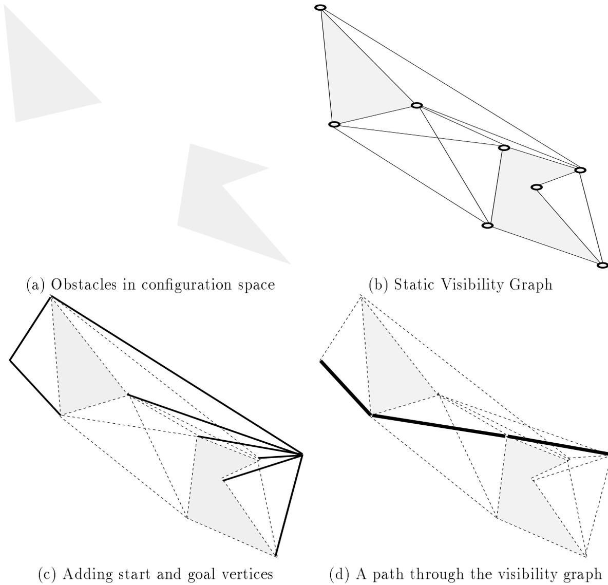
Figure 1: An example of path planning using a Visibility Graph
